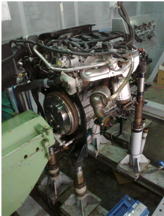
Fig. 1. Diesel engine 2.0 TDI 140 hp EURO 4 Volkswagen Group
