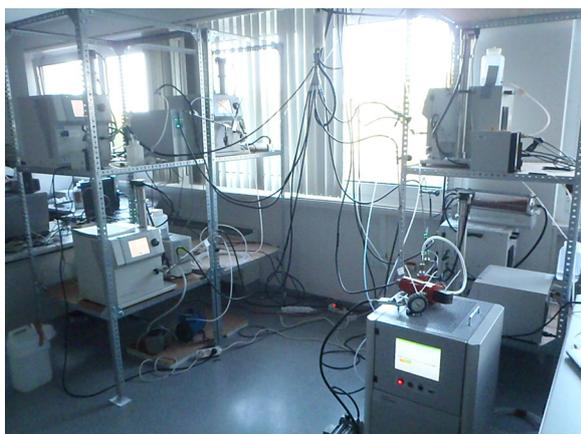
Fig. 1. In this picture it is possible to see three SMPSs on the left side and two SMPSs and an UFP on the right side during the instrument intercomparison. The flow splitter is in the top side
