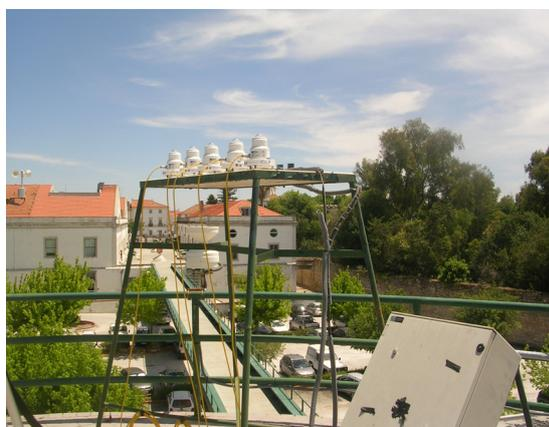
Fig. 2. Set of Kipp&Zonen radiometers that are installed in CGE atmospheric observatory.
