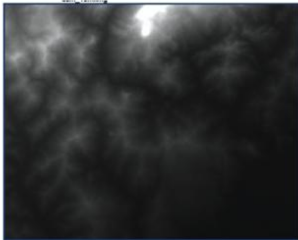
Fig. 4. DSM (digital surface model)_10m: Generated from TerraSAR-X StripMap (3m resolution)
