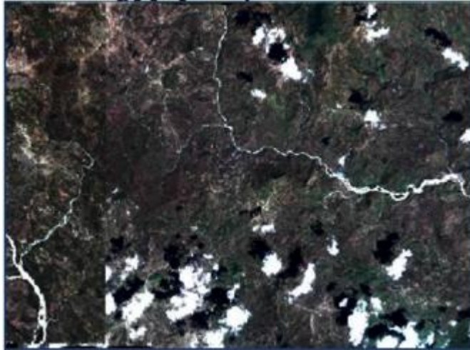
Fig. 3. Raster data: Orthorectified and ran mosaic from archived GeoEye-1 images (50 cm resolution) (scene date: 13 Nov 09 and 19 Sep 09), Natural color (3-bands), Unsigned 8 bit
