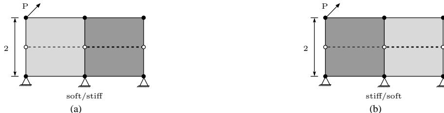
Figure 4: Mesh and loading conditions (dashed line indicates the prescribed discontinuity): (a) first element soft and second element stiff; (b) first element stiff and second element soft.
