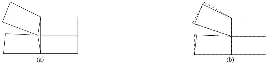
Figure 5: Deformed mesh for soft/stiffer case obtained with: (a) the GSDA; (b) the new formulation (continuous) and GFEM/XFEM (dashed).
