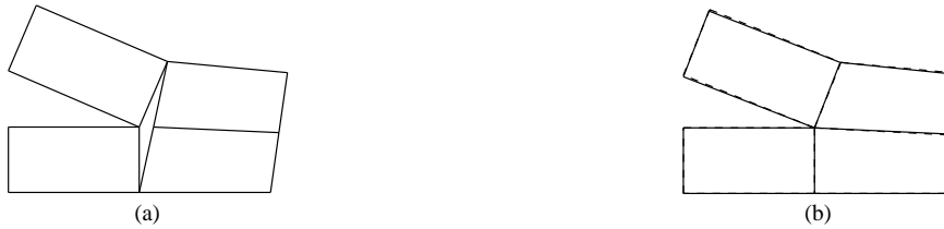
Figure 6: Deformed mesh for stiff/softer case obtained with: (a) the GSDA; (b) the new formulation (continuous) and GFEM/XFEM (dashed).
