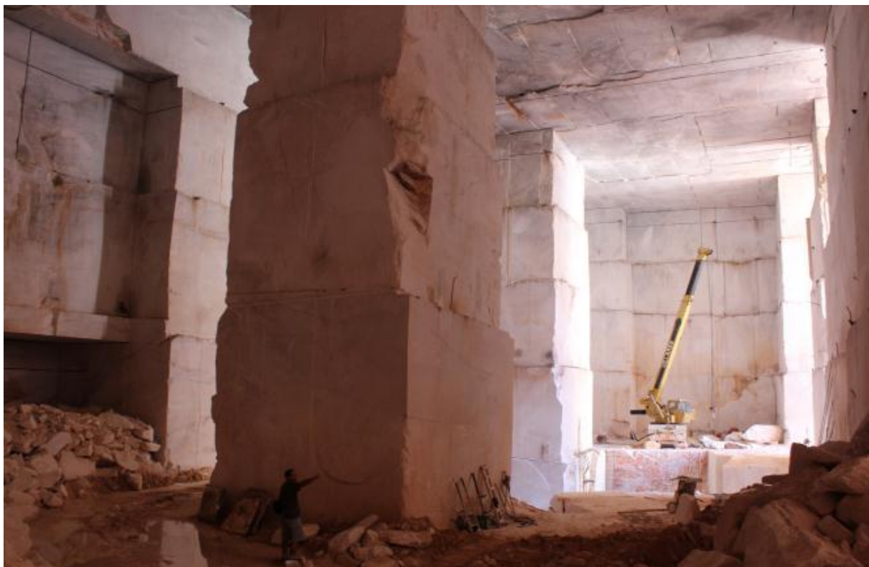
Figure 6. Underground quarry in the SW limb of the Estremoz anticline. The best quality marble pursuit requires a good geological knowledge of the deposit and only then becomes profitable underground mining of this resource. Lugramar Company Quarry.
