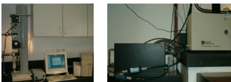
Figure 1. Pictures of the nephelometer (left) and TEOM (right) inside the laboratory
