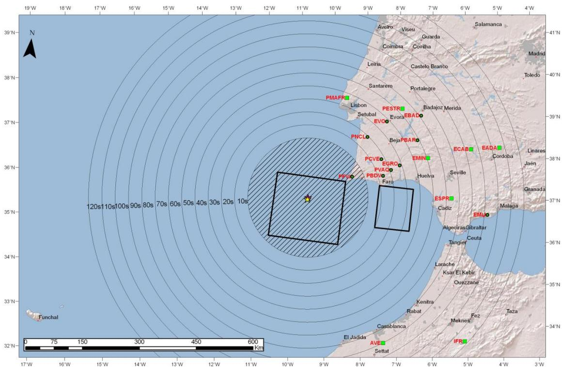
Figure 4.1.- Lead time scenario for a M5.5 earthquake, obtained from an automatic detection and location performed with 6 stations. Automatic epicenter (purple star) and reference epicenter (yellow star) are shown, together with , blind zones( dashed line circle) and lead times . Stations with median time picking differences <0.1s are shown as green circles, and stations with larger differences as green squares
