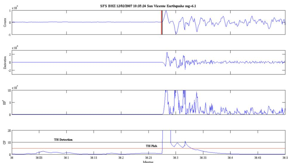
Figure 3.1 Automatic picking (Baer and Kradolfer algorithm) for 2007 S. Vicente earthquake ( $M_w=5.9$ ) for SFS station. From the top to the bottom BHZ record, its derivative, the square EF function, and the characteristic function CF and the threshold are shown
