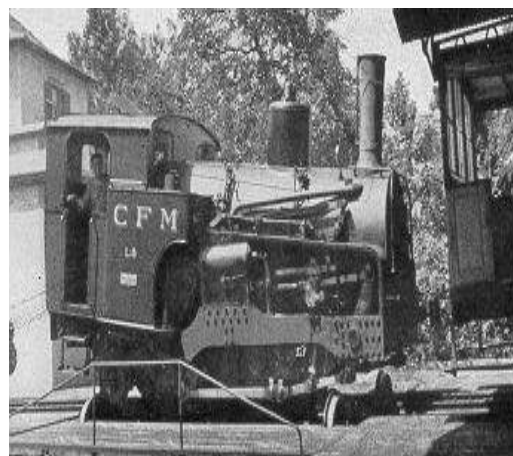
Figura 7. Locomotiva de montanha L-5 (0-2-1) do CFM. © Por Ransome-Wallis, On railways at home and abroad , estampa 72.
