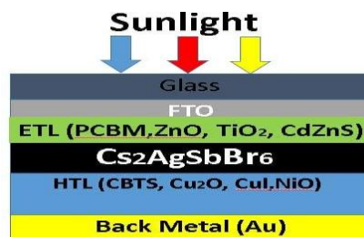
Fig. 1. Device structure of the \text{Cs}_2\text{AgSbBr}_6 -based perovskite solar cell.
