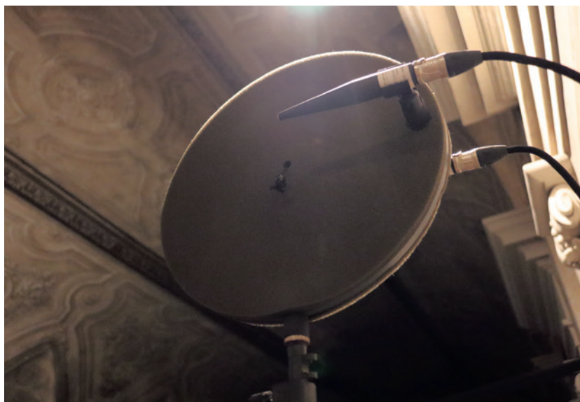
Fig. 8. Positioning the recording system: Jecklin disk and DPA 4090.
