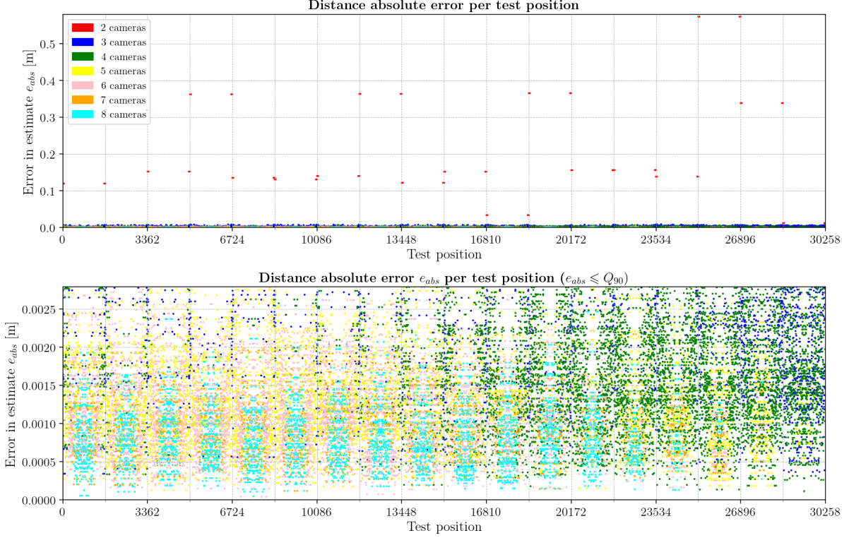
Distance absolute error e_{abs} per test position Test: 02, Camera Model: OV2640, Resolution: 1600×1200, 8 cameras
