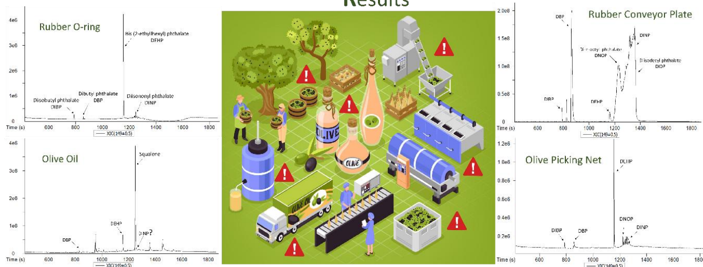
Figure 2. Extracted ion chromatograms showing m/z 149 (characteristic of PEs) from the extract of different materials used in olive oil production, and of olive oil itself.
