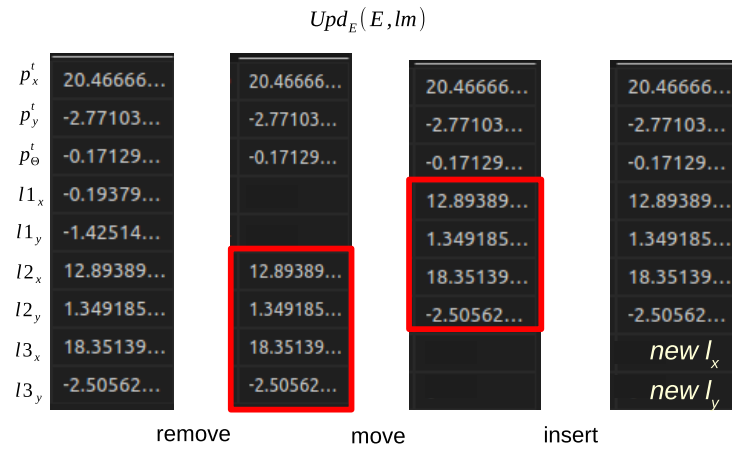
Figure 4. A simple example of updating the state vector with N_{lm} = 1 and k = 3 . The red box highlights the items that are moved during the update.
