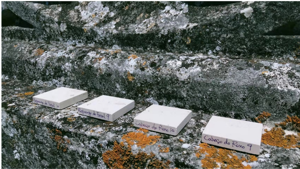
Fig. 2. Uncoated and SiO x deposited stone samples placed on the roof of Batalha Monastery (from left to right, 1st and 3rd covered with SiO x thin film, 2nd and 4th uncoated).
