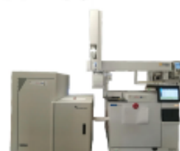
GC-ToFMS (Agilent 8890, Markes Int. Bench TOF-select detector, CTC Analysis autosampler PAL-System)
