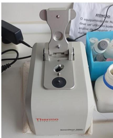
**Figura 9** - NanoDrop 2000c Spectrophotometer Thermo scientific.
