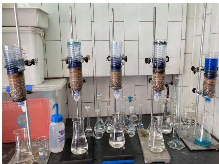
Figure 2. Preparation of filters containing sand and low-cost adsorbents. Different steps in the filtration process (Photo is the authors' own).
