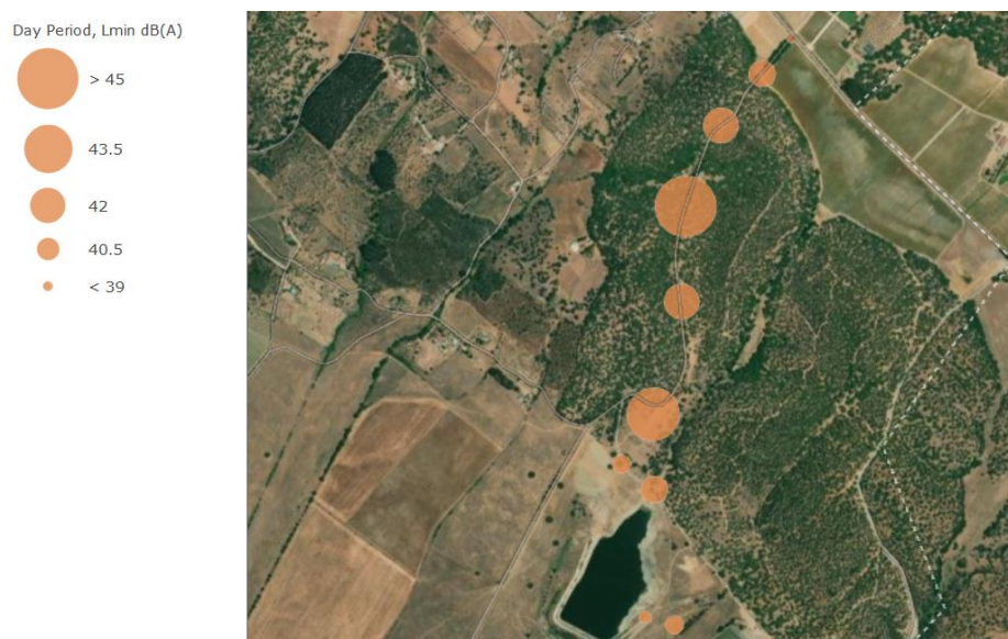
Figure 52: Noise mapping of Quinta Do Carmo for L_{min}
