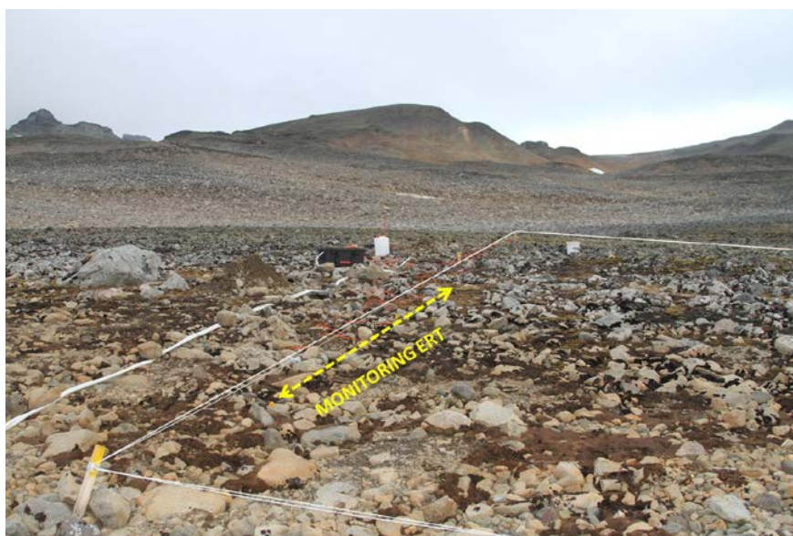
Figure 4. Picture of the MONITORING area described in the text. In white are shown part of the limits of the area where 2 shallow boreholes for temperature and moisture monitoring were excavated. The ERT was done along the left limit in the picture (yellow double arrow) where the cables in orange and the stainless electrodes can be seen. The black box on the top contains the resistivity meter which will continue to monitor the ground resistivity in an automatic way.
