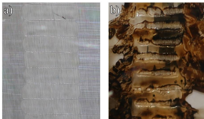
Figure 14 – a) Welding lines of a) samples welded with W \approx 2 W, v = 5 mm/s and b) samples welded with W \approx 8 W, v = 20 mm/s.
