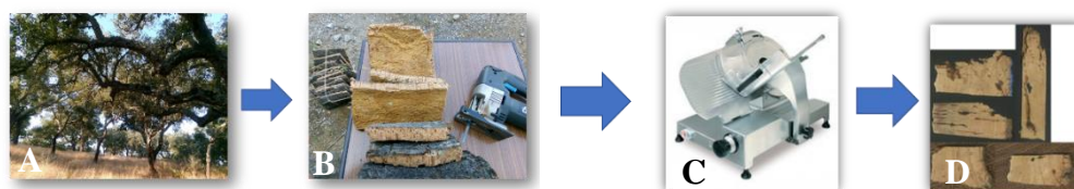
Fig. 44 Steps of cork samples preparation: A – example of a plot; B – samples collected; C – Slicer machine; D – cross-sections
