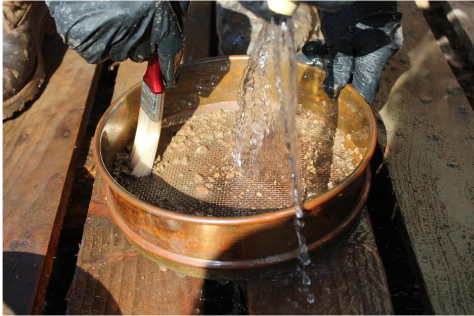
Figure 18 - Sieving process. Picture taken by Pedro Bonifácio.
