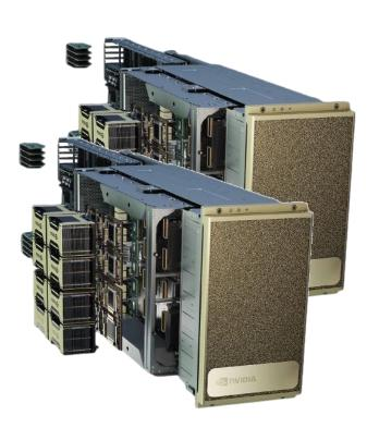
Two NVIDIA DGX<sup>™</sup> A100 Stations are deployed in the HPC laboratory "VISTA Lab" in the Évora University. Universal system purpose-built for all AI infrastructure and workloads, from analytics to training to inference. Each station is built on eight NVIDIA A100 Tensor Core GPUs. Docker Containers platform is used to deploy the toolset for high-performance computing (HPC) in the Vista Lab.
