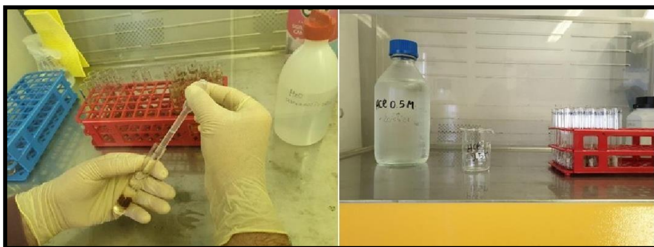
Fig 21. The process of changing acid and neutralising the samples (right) the sample placed in the tubes with HCl solution (left), (Photo by Abobaker Afat).
