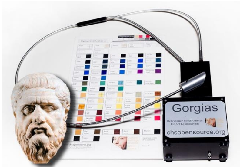
Figure 2-10: Gorgias Reflectance Spectrometer for Art Examination 2
