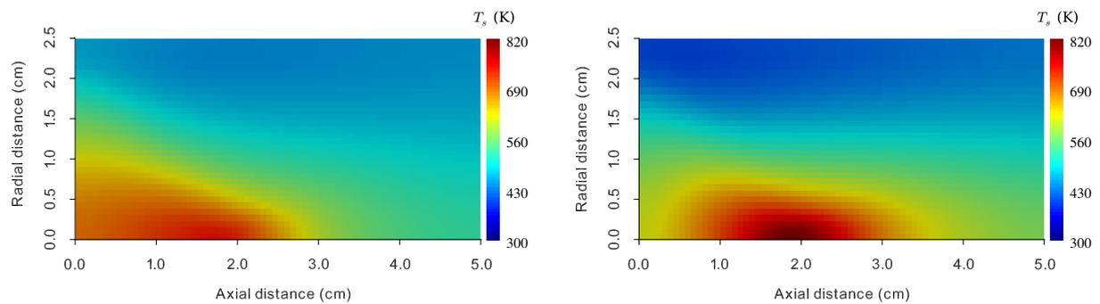
**Figure 2.** Temperature distribution in solid phase ( $T_s$ ) of receiver configurations (a) A and (b) B.
