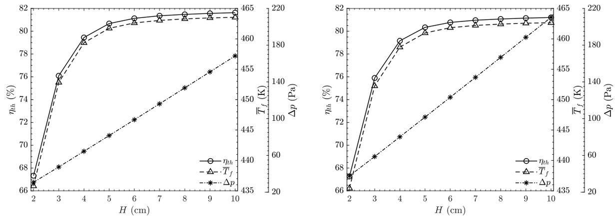
**Figure 3.** Thermal and hydrodynamic performance of the receiver configuration (a) A and (b) B with different thicknesses.
