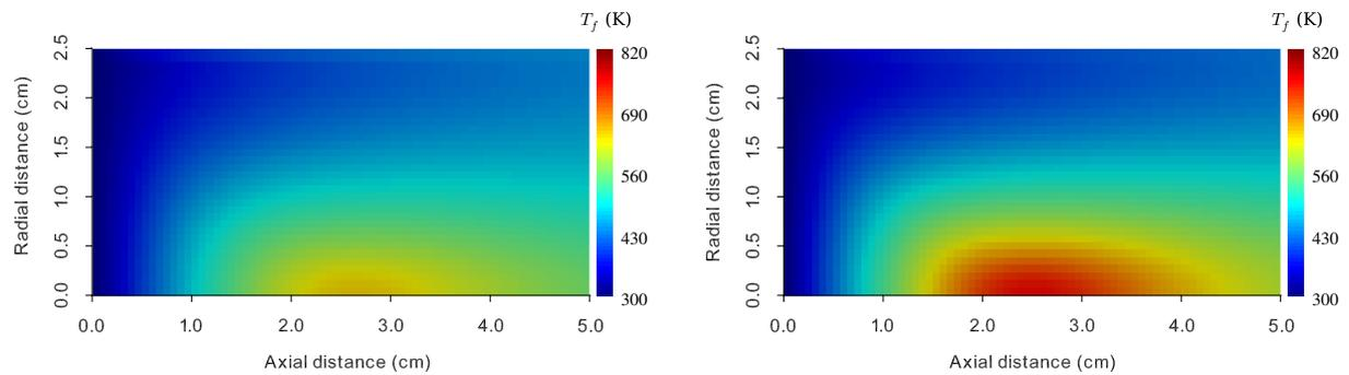
**Figure 1.** Temperature distribution in fluid phase ( $T_f$ ) of receiver configurations (a) A and (b) B.
