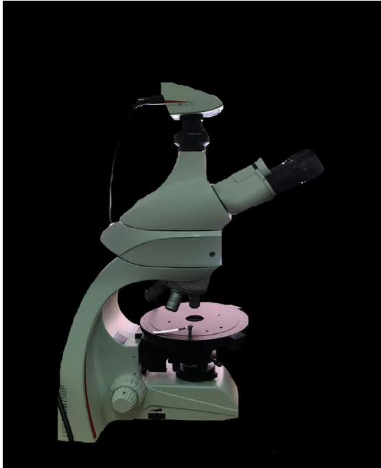
Figure 2.7 - Leica DM750PZeiss D-7082 Oberkochen polarized optical microscope equipped with a Leica MC190-HD camera (Department of Earth Sciences, Sapienza University of Rome, Italy)
