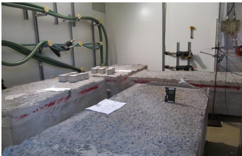
Figure 11 Curing samples under controlled conditions (40°C and 60% RH).
