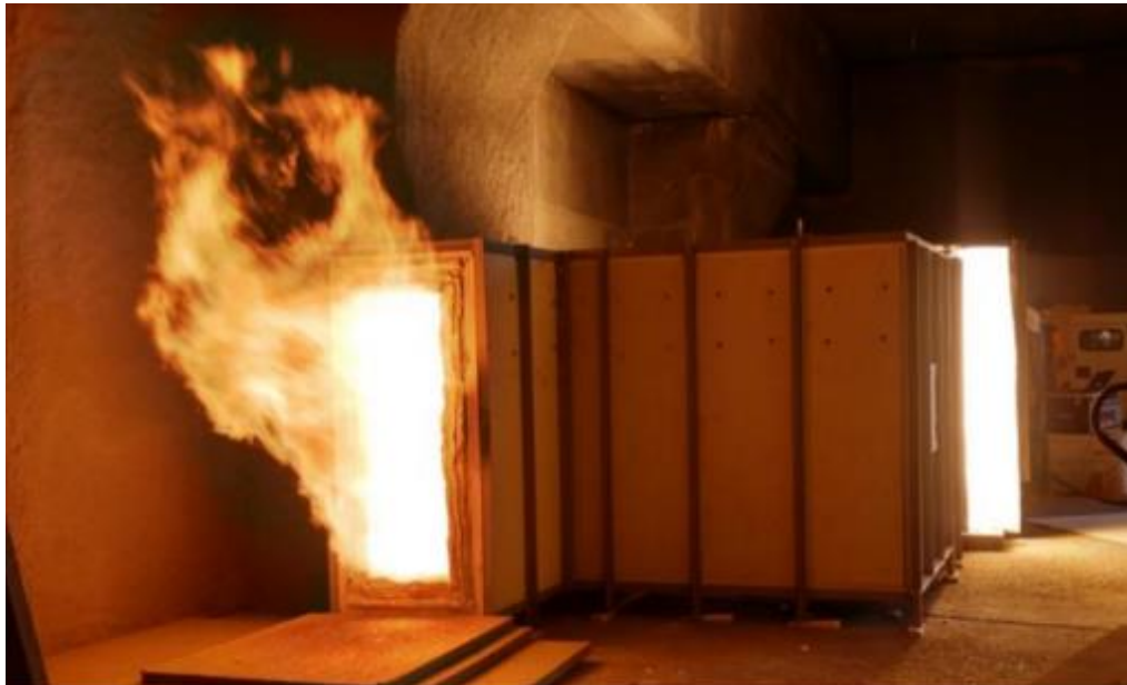
Figure 3 Picture of the fire chamber. The mobile fuel-fired furnace is hidden behind. This picture was taken in one of the tested tunnels located along the Paris ring road.
