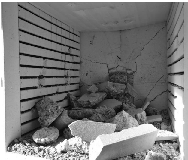
Figure 5 Prismatic sample after spalling
