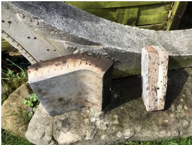
Figure 6 section of the leaf which has been in a fire temperature over 1,000 degrees, sufficient to make steel 'white hot'. The ferrocement maintains its integrity after cooling.
