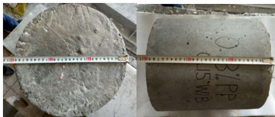
Figure 2 \phi 30 \times 30 cm cylinder
