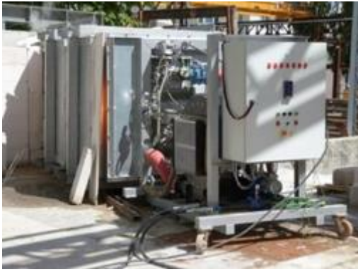
Figure 1 Combustion control cart and heat protective shield of the mobile oil-fired furnace.
