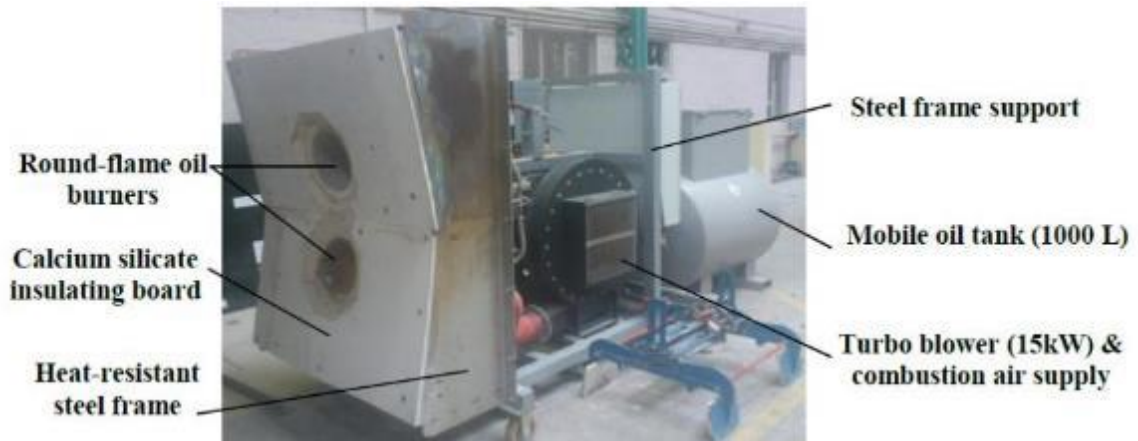
Figure 2 Firing hood with two oil burners.
