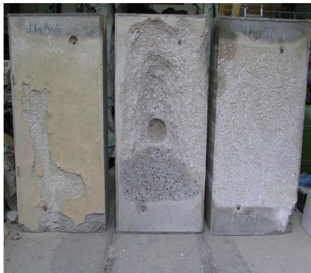
Figure 8 Comparison of specimens following hydrocarbon fire test (1kg/m 3 PVA fibres on left, no fibres in middle and 1kg/m 3 p/p fibres on right)
