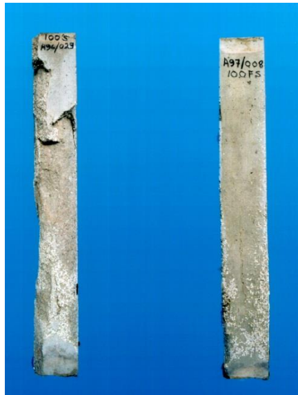
Figure 3 Comparison between high strength unreinforced columns with (right) and without (left) fibres.
