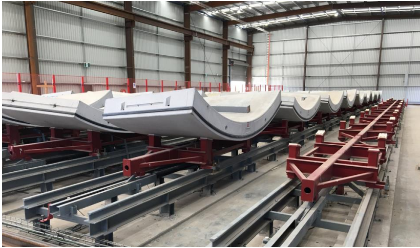
Figure 4 Tunnel Lining Segments
