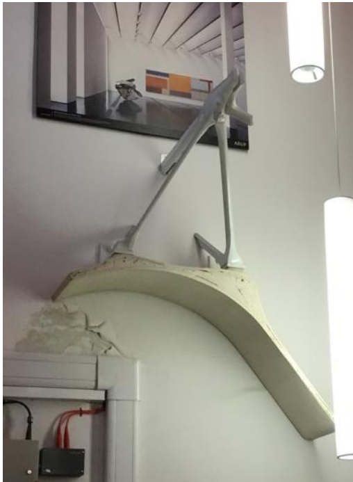
Figure 3 Section of deMenil roof leaf displayed in Leeds University Civil Engineering Department
