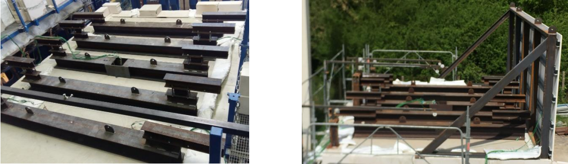
Figure 2. Mechanical load used for standard fire tests (left) and compartment fire tests (right)
