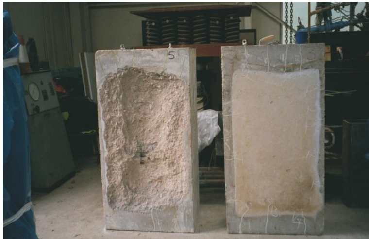
Figure 7 Comparison of test specimens with (right) and without (left) p/p fibres.
