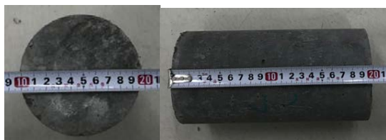
Figure 3 \phi 10 \times 30 cm cylinder
