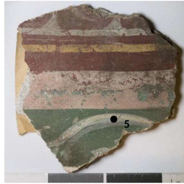
Fig. 19: sample overview (front) with indication of colorimetric and spectrophotometric analysis of spot 5
