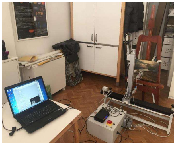
Figure 16. Analysis software in running on a laptop connected to Control Unit
