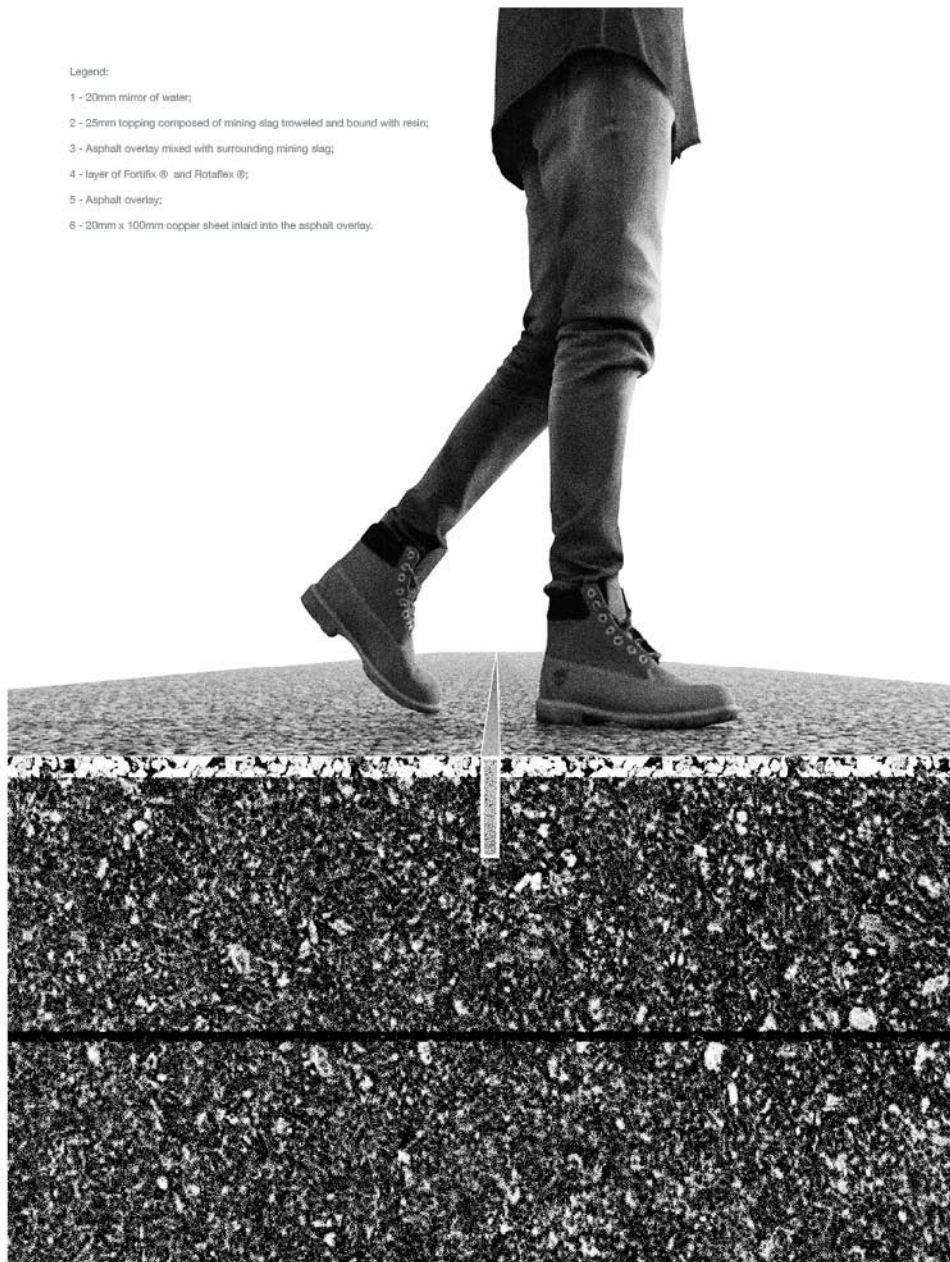
275 Detailed section (© Jared Miguel Fantasia, 2018) showing impermeable covering of the proposed project with the inlaid copper plates that delimit the once visible S. Domingos orebody (left) without water (right) with water covering. Note: The above drawings are for illustrative purposes only.
