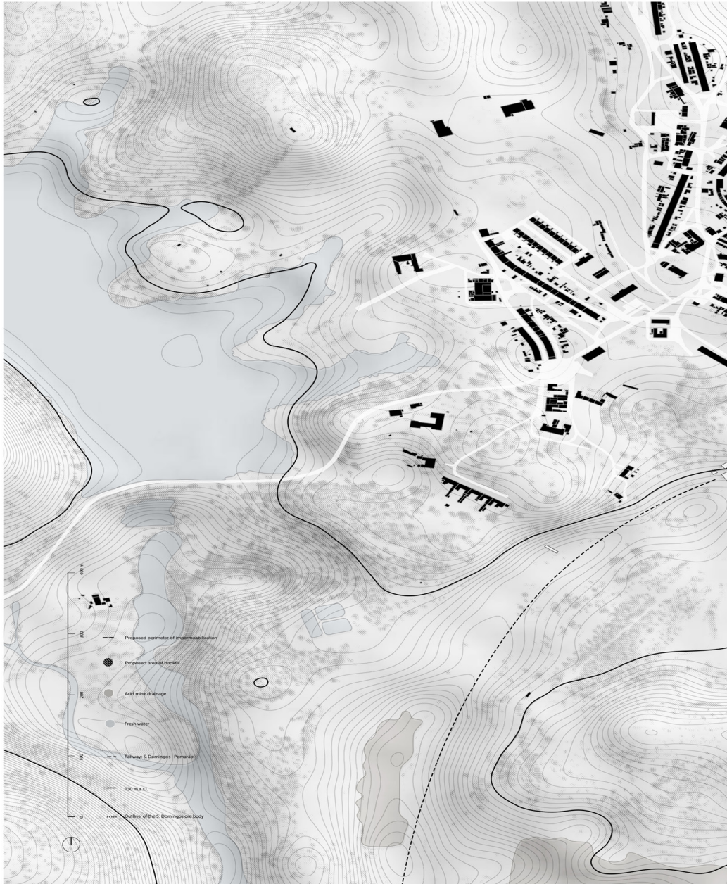
220 Map showing the project consisting of the backfilling of the S. Domingos open pit to the mining level of 130m above sea level (equivalent to the 0m mining level). © Jared Miguel Fantasia, 2018
