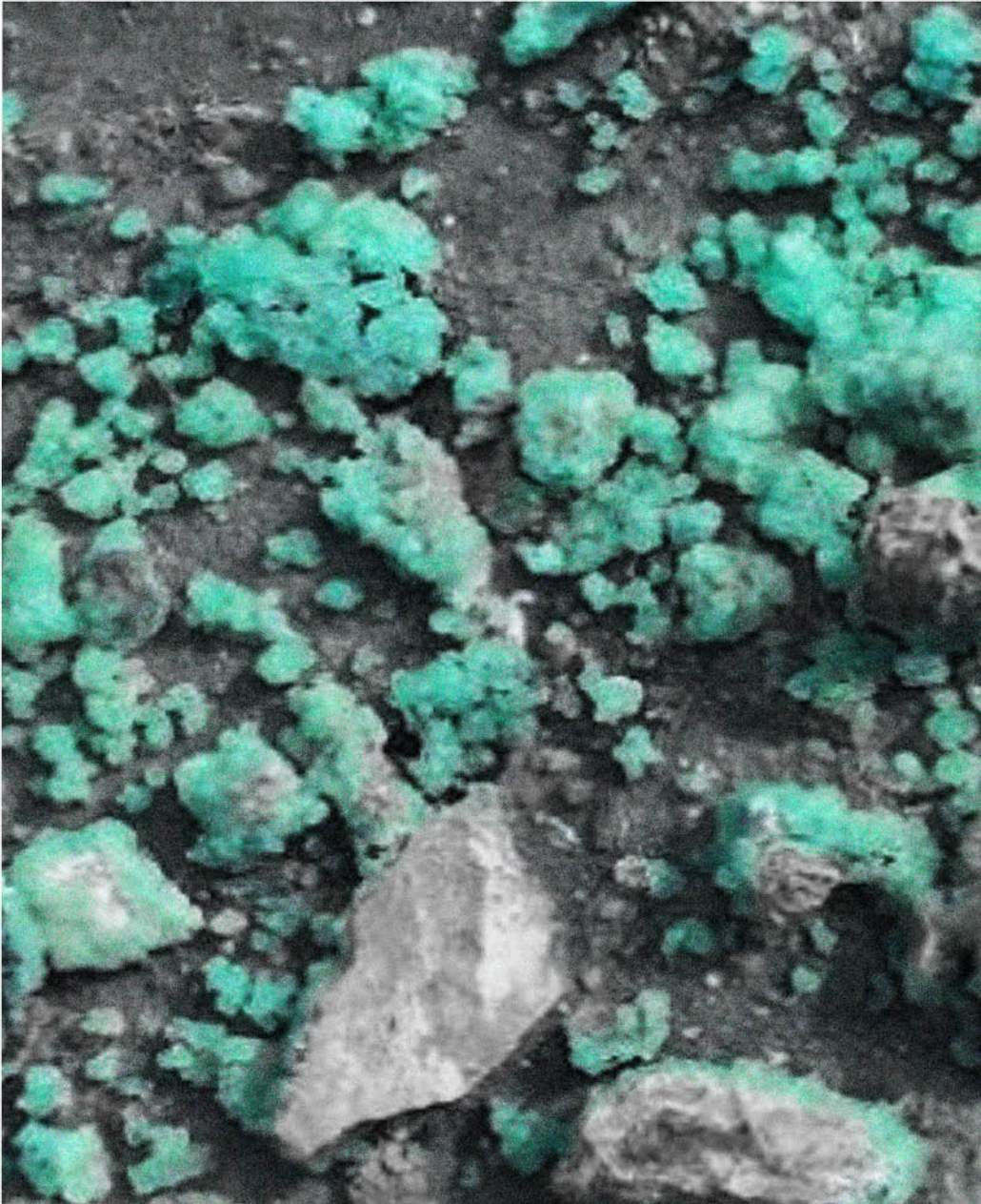
218 "Due to the extremely high concentrates of S-bearing minerals as well as sulphate salts, it is common to find carapaces made up of native sulphur crystals and neo-formed sulphates (melanterite, jarosite) at the edges of the various acid dams in the area. The sulphates are mostly visible in summer as they dissolve when it rains."(De Oliveira, D. 2018.)
