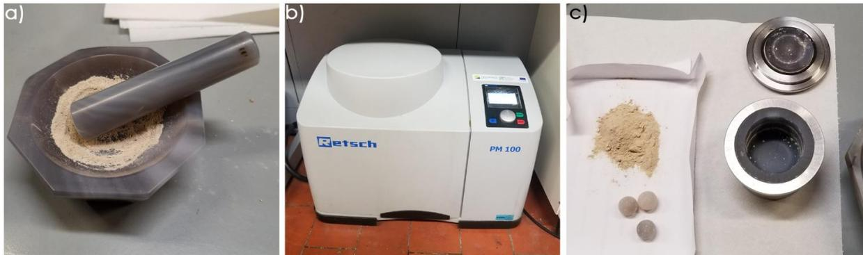
Figure 3-8. Tools used for the preparation of the powdered samples: a) Disaggregation by mortar and pestle, b) Powdering equipment PM 100 Planetary Ball Mill (Retsch), c) Agate grinding jar and grinding balls
