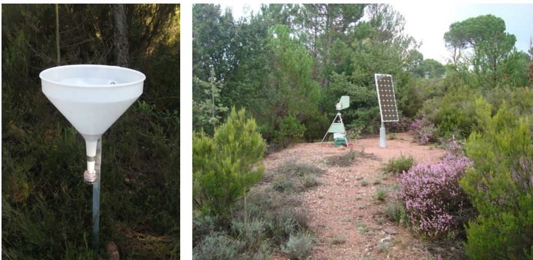
Figure 6.3: Example of a passive spore traps or funnel spore trap (Left) and an active (Burkard) spore trap (Right) using a solar panel as a source of energy supply (Photo credits: Carles Castaño).
