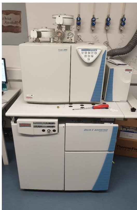
Figure 4.3: EA-IRMS equipment which was used for nitrogen and carbon stable isotope analysis at HERCULES Laboratory.
