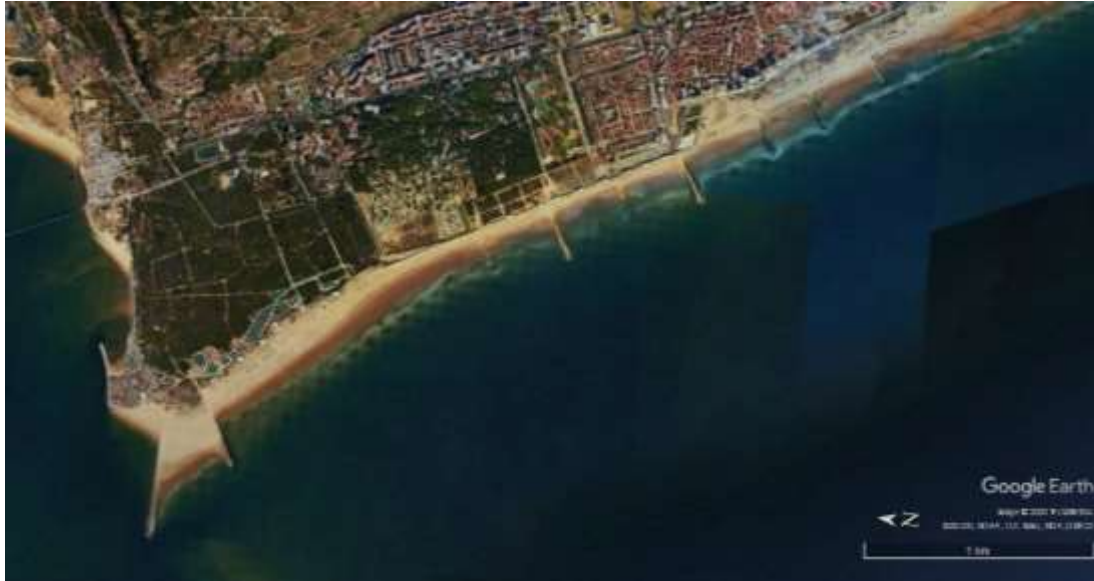
Figure 20: Spurs built in Costa da Caparica and Cova do Vapor. Image: Google Earth, 2015.
