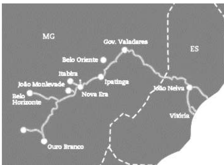
Figure 20: Vitória-Minas Railway over its 905km of length, which connect the iron ore operation points in the interior of Minas Gerais to the Port of Tubarão, in the state of Espírito Santo. Accessed in 24 mar 2020 <>www.vale.com.br
