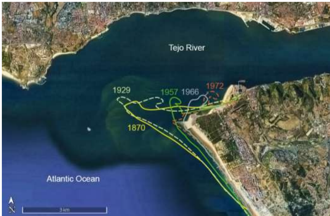
Figure 14 : The evolution of the Costa line between 1870 and 1972, based on a satellite image from Google Earth 2015. Adapted from (Gomes, Costa da caparica Artificial Sand Nourishment and Costal Dynamics 2009, 679).
