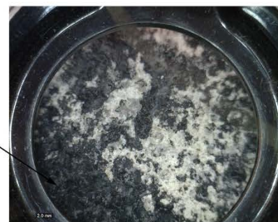
Portable optical microscope image E3418 displaying black paint layer affected by salts' efflorescence, magnification 20x
