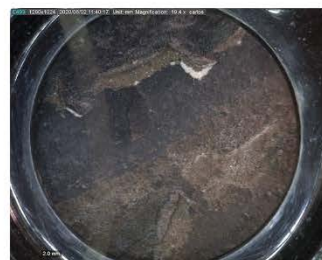
Portable optical microscope image E496 displaying the flaking brownish paint layer magnification 20x
