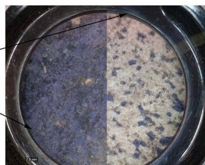
Portable optical microscope images E367 (on the left) and E365 (on the right) displaying different stages of salts' formation, magnification 20x
