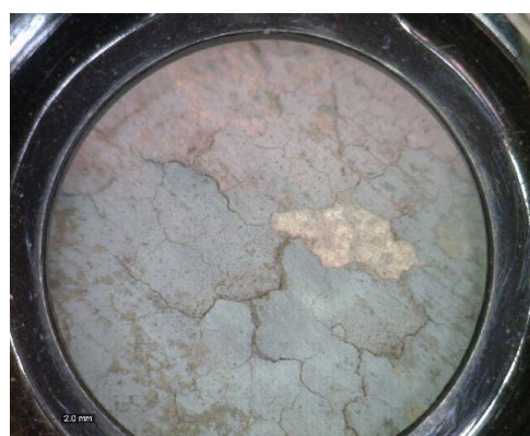
Figure 19. Portable optical microscope image E574 of a flaking greenish layer of Angel's garment, mag. 20x
