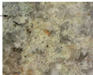
Portable optical microscope image E735 of greenish paintlayer in the background affected by flaking and salts, magnification 434x
