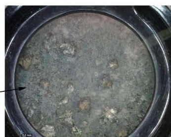
Portable optical microscope image E378 displaying green paint layer affected by salts' formation, magnification 20x
