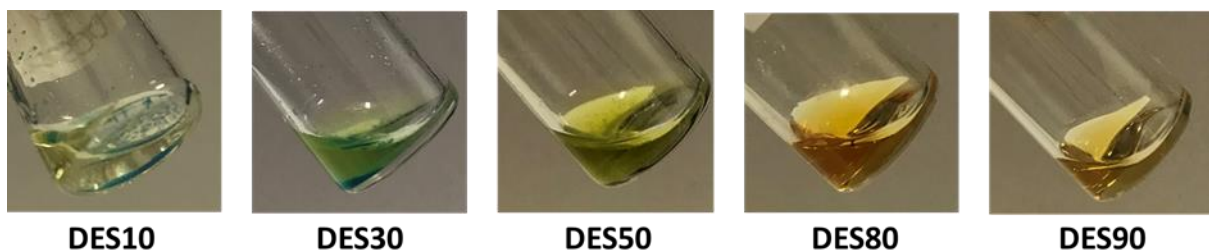
Fig. 4.3 Photos of the dissolution test taken after several days after adding copper corrosion powder to the mixture.
