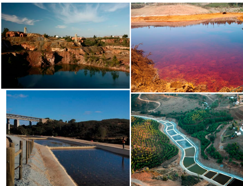
Figure 13 – Lousal mine. Pictures represent the acidic waters and the lagoons with floating macrophytes for reduction of pH and metals concentrations.
