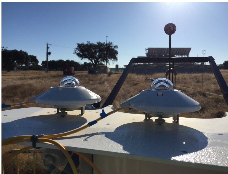
(b) Two pyranometers are used for GHI and DHI measurements (MIT station).
