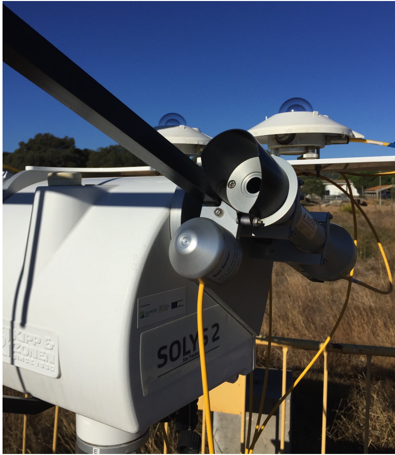
(a) One pyrheliometer is used for DNI measurements (MIT station).
