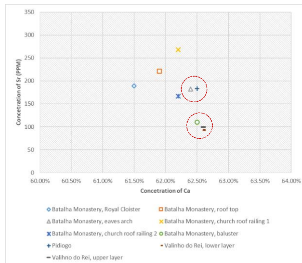
Fig. 7. Ca-Sr element alignment based on XRF.
