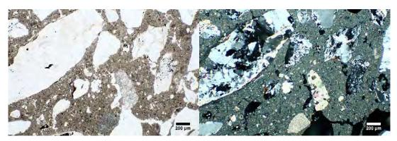
Figure 5: Thin section from *intonaco* of the Holy Cross Chapel, with a high B/A and mainly crystalline rock fragments as aggregate. Sample 24980: Left PPol, right XPOL.
