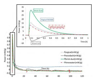
Figure 6: The kinetics evolutions of the pastes with different Pozzolans 10% at 40  $^{\circ}$  C
