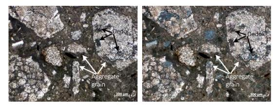
Figure 5: Sample D1 under optical microscope. Magnification 50x, PPT (left). Magnification 50x, XPT (right).
