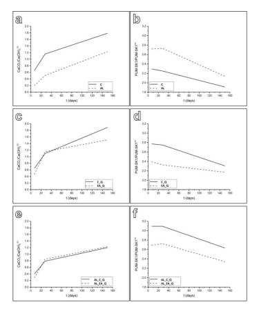
Figure 1. CaCO<sub>3</sub>/Ca(OH)<sub>2</sub><sup>(0)</sup> and PUM-SK1/PUM-SK1<sup>(0)</sup> ratios over time for each pair of grouts. Degree of carbonation of grouts (a) AL and C, (c) EA\_Q and C\_Q, (e) AL\_EA\_Q & AL\_C\_Q; decrease of the PUM-SK1 fraction of grouts (b) AL and C, (d) EA\_Q and C\_Q, (f) AL\_EA\_Q and AL\_C\_Q
