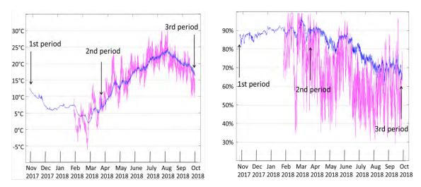
Figure 4. Temperature (on the left) and relative humidity (on the right) recorded during 13 months from October 2017 inside the Chapter Hall (blue line) and outdoors (magenta line)
