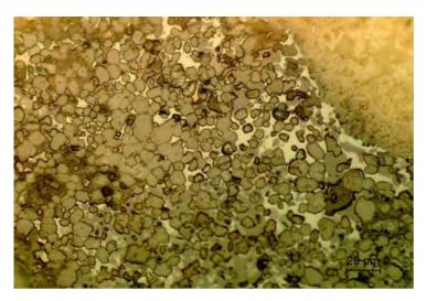
Figure 12. Detailed view of a clinker grain filled with small round beige C2S crystals showing parallel striations for some of them. Optical microscope view (G=X20) of the ochre render.
