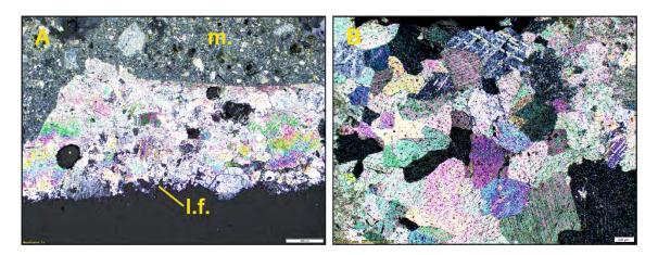
Figure 3. A. Microscopic character of the Slivenec lm. fragment (l.f.) found in the MPHBP1 sample with a fine grained mortar matrix (m.). B. Microscopic structure of the Slivenec lm. from the Radotín-Špička quarry. Both in CPL.
