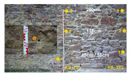
Figure 6. Test area at the historic wall with sampling points for salt and moisture investigations
