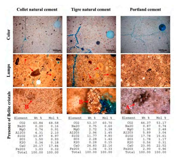
Figure 4. Analysis of Collet, Tigre and Portland cement samples. Alite (A), belite (B). [7]
