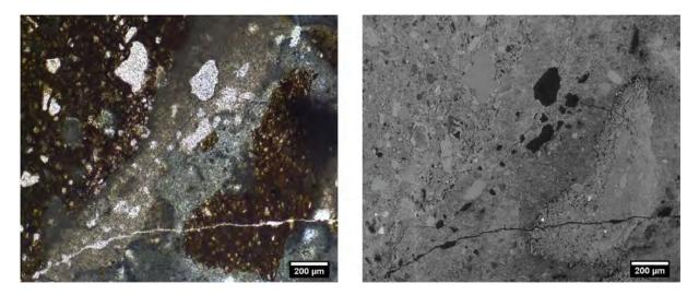
Figure 3. Inhomogeneous binder between brick fragments (very dark brown) in the sample CUT1 (left). Polarizing microscope image, parallel polarizers. Area of the left image (right). SEM image.
