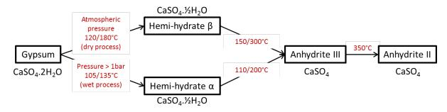
Figure 1: Calcium sulphate phases obtain by gypsum calcination at different temperatures.
