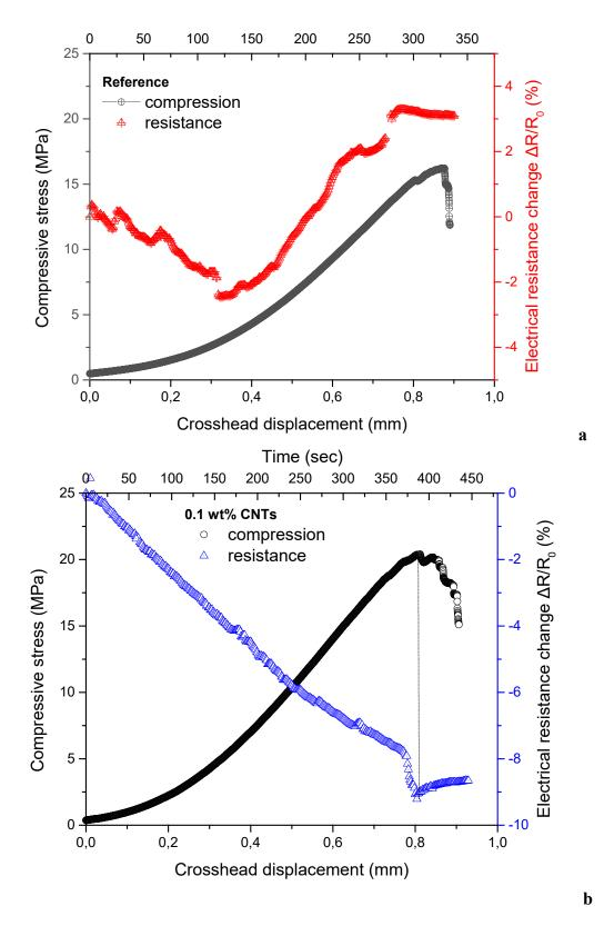
Figure 6. Representative graphs of the piezoresistive response of two ternary mixtures, i.e. LMCR (a) and LMC2 (b) during monotonic compression, after 28 days setting/hydration time.
