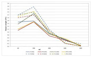
Figure 6. Flexural strength of the mortar compositions at elevated temperatures (28 and 90d)
