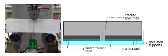
Figure 1. (Left) Crack control during 3-point bending test (left) and absorption by capillary through the crack test setup (right).
