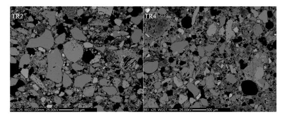
Figure 4. Micrograph of the lime mortar sample indicating numerous pores and different size and shape of aggregates
