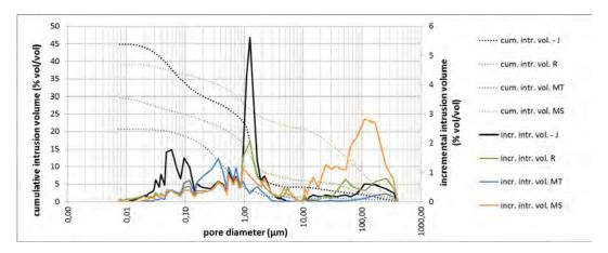
Figure 5. Pore size distribution (dotted line) and open porosity (continuous line) of the repair mortars as measured by MIP'
