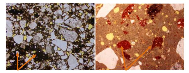
Figure 14. Crushed red bricks (see arrow) can often be found in mortars for renders or pointing. Here it is illustrated by a modern NHL3,5-mortar made for the re-rendering of Stockholm royal castle and a historic render on När church. In both samples it is mainly there for aesthetic reasons as the aggregate is visible due to the surface working method and the render is left without lime wash. Illustration: Kristin Balksten.
