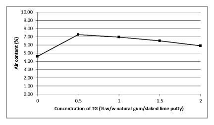
Figure 4. Air content of mortars vs. concentration of tragacanth gum (TG)
