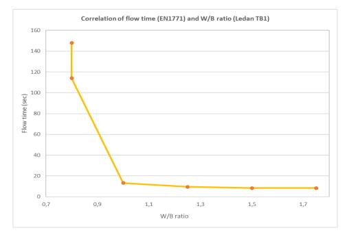
Figure 5. Correlation of flow time according to EN 445:2007 and W/B ratio of Ledan TB1 mixtures, prepared by the three Laboratories.
