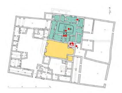
Figure 5. Plan of Topographical Unit 28 in yellow the church and in green the monastery and the localisation in red spots of the seven mortar samples (modified by Piero Gilento and Sara Peñalver Martin, 2018).
