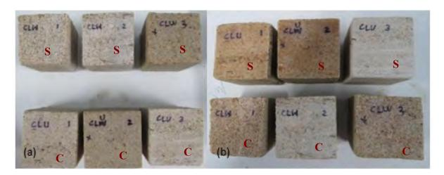
Figure 7. Specimens (a) before and (b) after salt weathering cycles
