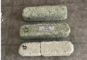
L-NZ after 9 cycles of  $Na_2SO_4$  crystallization
