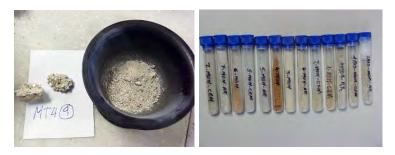
Figure 7. Finely grinded mortar samples for analysis by XRD.
