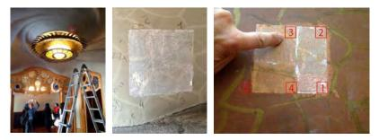
Figures 7a, 7b and 7c. Selective samples showing the different layers along the interventions.
