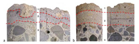
Figure 4. Finishing mortar (1), bonding mortar (2) core (3), a: sample M1, b: sample M2
