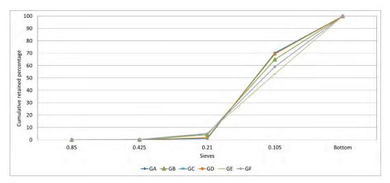
Figure 2. Grain size curves of gypsum plaster.
