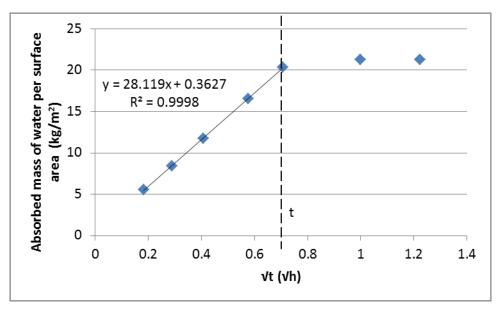
Figure 6. Principle of determining capillary water absorption coefficient presented on an example of mixture designated 1/3-40 at the age of 60 days (RH=100%)
