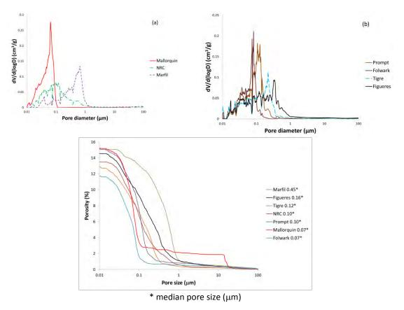
Figure 4. Pore size distributions of mortars; (a) & (b) - derivative, (c) - cumulative
