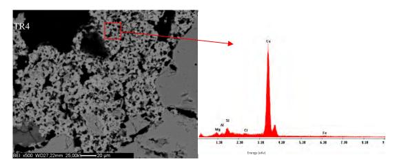
Figure 5. Micrograph showing interconnected pores and a carbonated matrix
