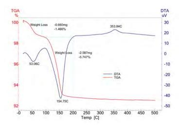
Figure 5. TGA and DTA curves of GB gypsum plaster.
