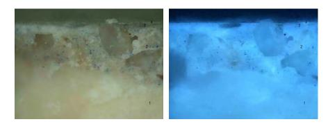
Figure 15a and 15b. OM Cross section (10X/0,30) with incident light and UV light of the coloured stucco, where it is perceived: 1-white base stucco; 2-lime mortar with blue pigment; 3-finishing layer hot-ironed; 4-acrylic paint overlaid.
