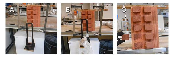
Figure 4. Shear adhesion test on moulded samples: (A) application load device on a sample; (B) successive 250 g loads applied on the device; (C) a moulded samples after rupture.
