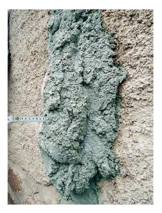
Figure 3. Hot applied mortar (HAM) in mixture H3, with pumice, allows a thick package of mortar applied in one step because of very fast setting
