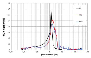
Figure 8. Pore size distribution of 28-day-old mortar samples with and without nanoparticles.
