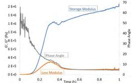
Figure 8: Storage modulus, loss modulus and phase angle against time for 10% Argical M1000 at 40 °C
