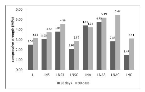
Figure 1. Compressive strength values (MPa) of nano-modified hydrated lime systems.
