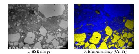
Figure 11. External and internal layers of MRBH7-13B.
