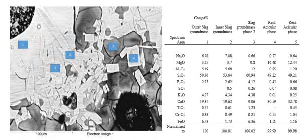
Figure 4e. SEM image of part of a slag grain in Type B mortar sample TWO.08. Numbered areas relate to EDS analyses in adjacent table. Scale bar 100µm; SEM image John Hughes.
