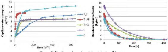
Figure 5. Capillary absorption (a) and drying (b) curves.
