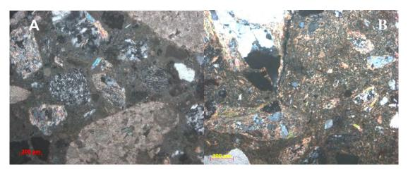
Figure 4: thin section images 5x, XPOL. A) Sample 10127 bedding mortar of the "loggia building" similar to those of the convent; B) sample 9105, painted plaster of the loggia building characterized by high presence of very fine crystals of (possible) clay minerals.
