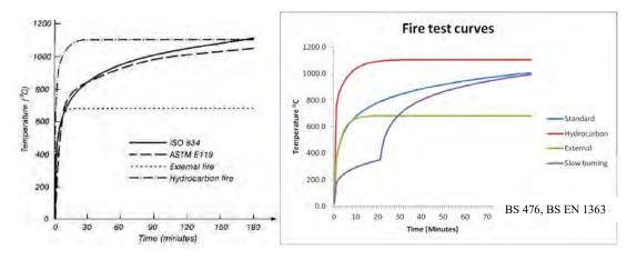
Figure 1. Temperature / time development standard curves during fire action [5]
