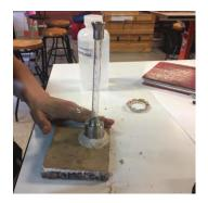
Figure 20. Water absorption test with Karsten tube. TECTRAD / INAH 2018
