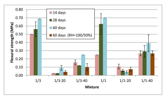
Figure 3. Development of flexural strength of samples through time
