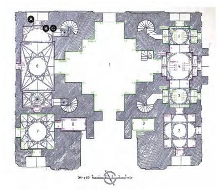
Figure 2: Ground plan of the mausoleum Ishrat Khana and sample locations, later modified [1]
