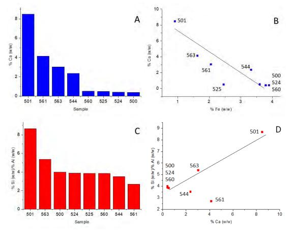
Figure 6. Comparison of mortar samples in terms of elemental composition. A: % content of Ca (w/w); B: correlation between the content of Ca and Fe; C: Si/Al ratios; D: correlation between Si/Al ratio and Ca content
