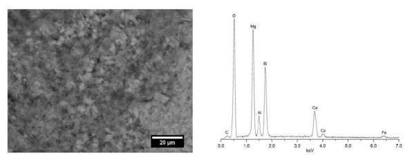
Figure 5. SEM image of a fragment of sample CUT1 (left). Corresponding spectrum of EDS measurement (right).
