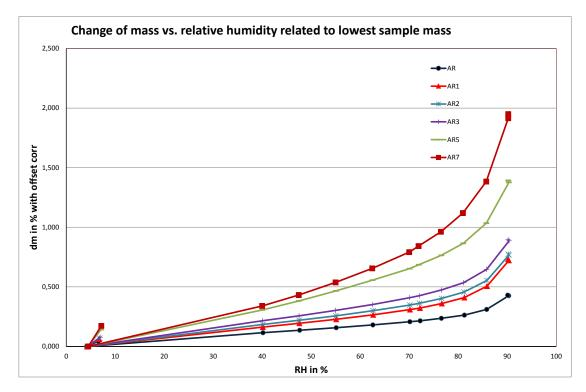
Figure 10. Water vapour absorption of samples as a function of relative humidity.
