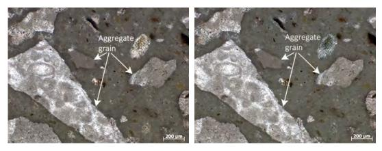
Figure 6: Sample S1 under optical microscope. Magnification 50x, PPT (left). Magnification 50x, XPT (right).
