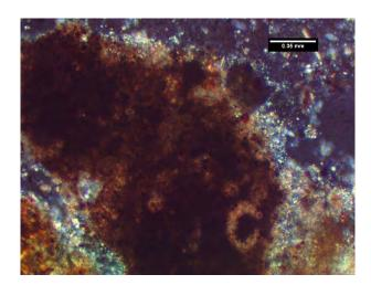
Figure 24. Sample B3. Trasmited light, crossed nicols. Visible reaction rim around a ceramic fragment.
