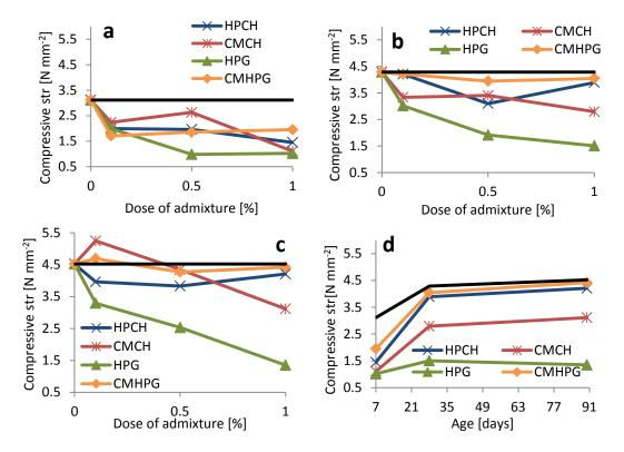
Figure 4. Compressive strength of studied specimens in the age of 7 days (a), 28 days (b), and 90 days (c) and time evolution of strength of samples with 1% of admixture (d).
