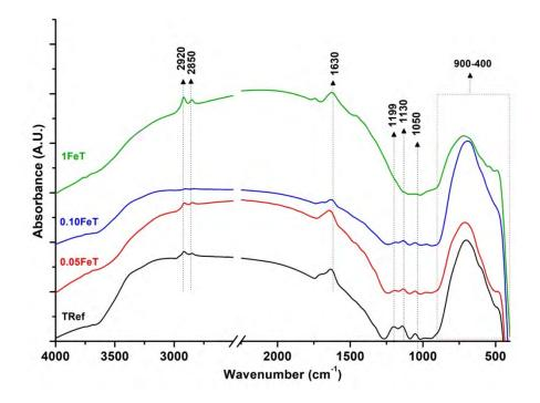
Figure 1. FTIR spectra of the synthesized photoactive Fe-doped TiO<sub>2</sub> nanoparticles along with the TRef sample.
