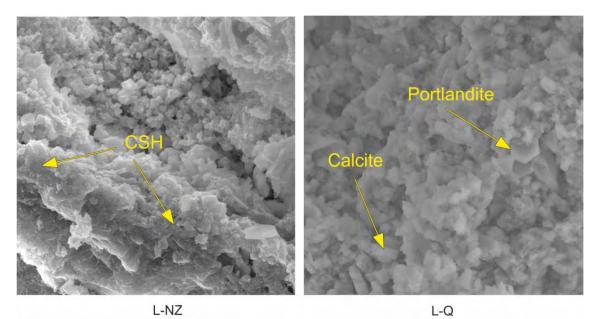
Figure 8. Detailed SEM images (magnification 10 000 ×) of L-Q and L-NZ render samples.
