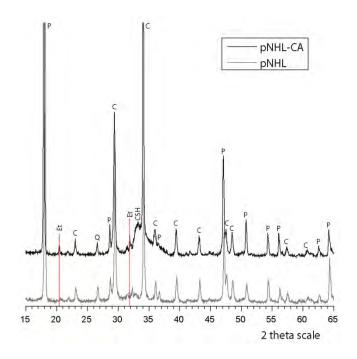
Figure 11. Diffractogram of the healing products produced in NHL-CA and control specimens after a 28 days healing period. [P: portlandite, C: Calcite, Q: Quartz, Et: Ettringite]
