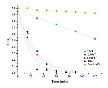
Figure 5. Photocatalytic efficiency of the synthesized nanoparticles.
