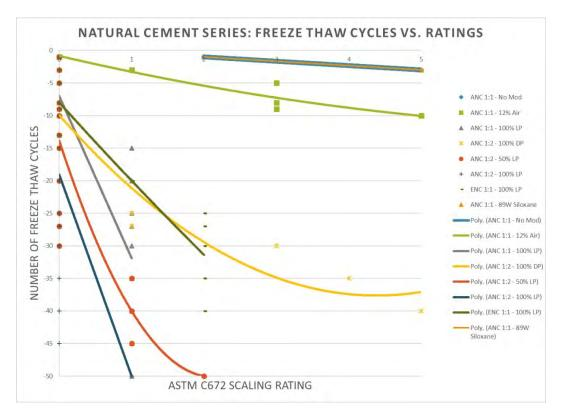
Figure 4. Natural-cement series: freeze-thaw cycles vs. scaling ratings
