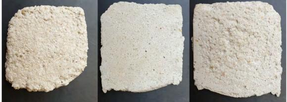
Figure 3. Three views of a mortar composed of marble passed through a 3 mm sieve (not intended to match Carrara marble). Left - the surface as applied off the spatula with rudimentary levelling. Centre – the same batch with all but the upper left corner polished. Right – the underside of one sample showing the coarse texture. It is noted that Carrara marble has grains in the range 300-500 microns, not those used here. No quartz flour was added to these mortars.
