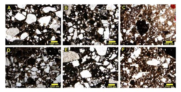
Figure 4. Petrographic observations (plain polars) of the multilayer wall mortar AD-124. A) Poorly sorted aggregates of the L1. B) Aggregated disposition of the L1.2. C) cocciopesto L2. D) Aggregates and lumps of L3. E) Poorly sorted aggregates of the L4. F) Clayed layer L5
