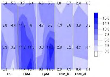
Figure 3. Moisture distribution in wt. % assessed by microwave probe.
