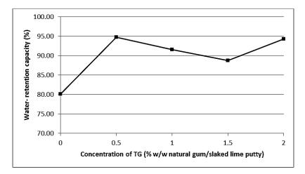
Figure 5. Water-retention capacity of the mortars vs. concentration of tragacanth gum (TG)
