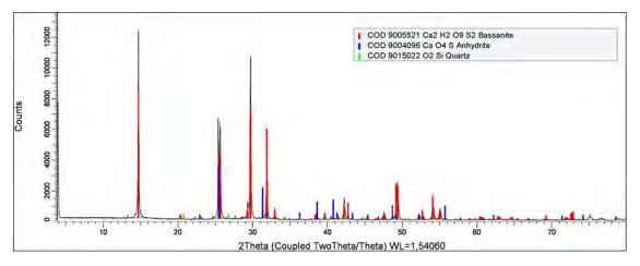
Figure 4. X-ray diffraction of GC gypsum plaster.
