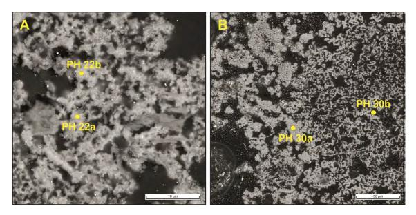
Figure 6. Character of the fine-grained mortar matrix observed in SEM with BSE detector (samples PH 22 – A and PH 30 – B), with marked positions of the micro-chemical analyses.
