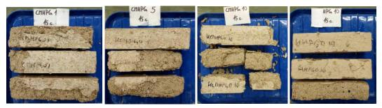
Figure 7. Highly altered samples after 15 freezing-thawing cycles (numbers represent admixture dosage in ‰).
