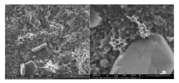
Figure 7. Portlandite crystals and needle-like CSH phases observed after 14 days healing period. NHL (left) and NHL-CA (right)
