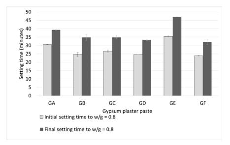
Figure 7. Initial and final setting time of the paste with w/g of 0.8.
