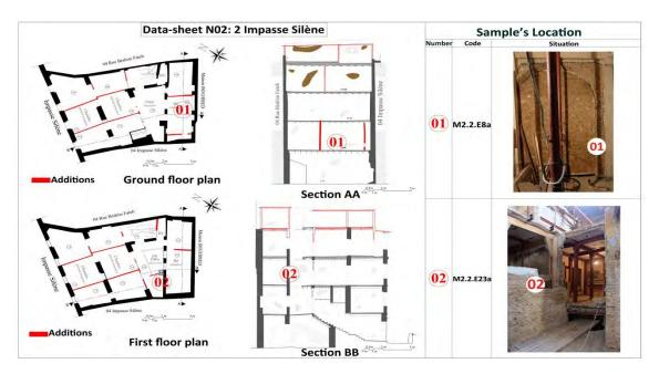
Figure 5. Data sheet of the house layout and the collected samples position
