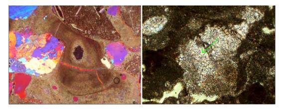
Figure 3. To left: Above is an example of lime use with partially burnt lime. The dark area in the centre of the picture is lime that is not burned. All lime in a shaft or lime kiln was not burned, so limestone lumps remained after quenching. The image covers 4.7 x 3.1 mm.
