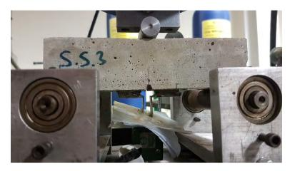
Figure 3. Testing arrangement on notched beams
