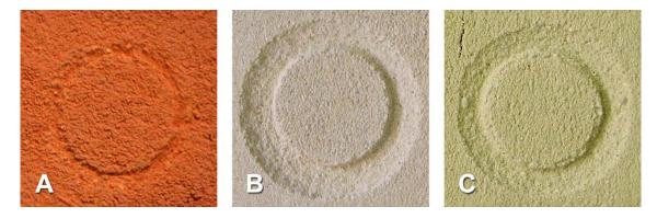
Figure 7. Aspect of dry abrasion over samples of 20 mm plaster layer applied over hollow bricks: (A) - Illitic mortar; (B) - Kaolinitic mortar; (C) - Montmorillonitic mortar.
