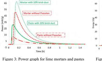
with and without brick dust (pozzolan). Measurements taken at 40 ° C
