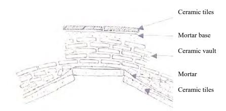
Figure 1. Detail extracted from this report [7] "Section of the disposition of different materials forming the vault in the studied area"
