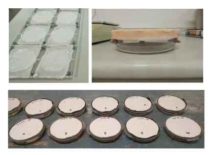
Figure 1. Samples in their test specimen recipients by UNE-EN 1015-19 [11]
