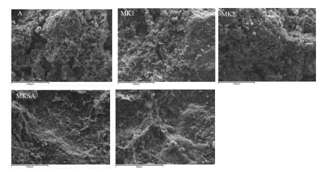
Figure 6. SEM images of the specimens (scale-100µm for A, MK10, MK20, MKSA and 80µm for SA).
