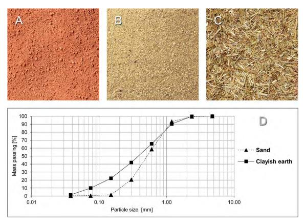
Figure 3. Clayish earth (A), sand (B), oat fibres (C) and dry particle size distribution of the sand and clayish earth (D) used in the mortar formulation.
