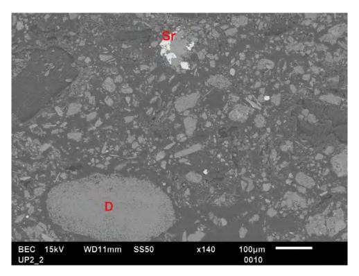
Figure 10: SEM backscattered image of plaster B, a rounded carbonate aggregate consist of dolomite (D), above a limestone aggregate with light celestine (SrSO<sub>4</sub>)
