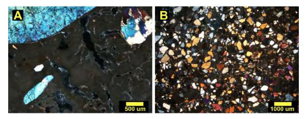
Figure 2. Petrographic observation of floor mortars (crossed polars). A) AD-192 mortar with scarce quartz inclusions in binder. B) Quartz aggregates and lumps in the AD-114 mortar
