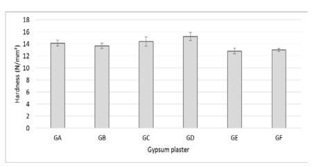
Figure 8. Hardness of plasters for w/g ratio of 0.8.
