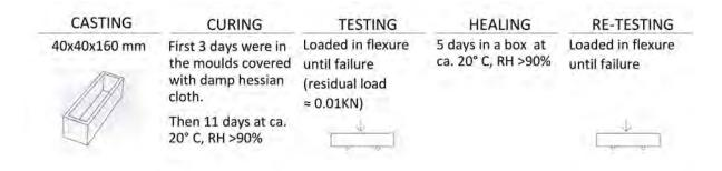
Figure 3. Experimental program for studying self-healing of lime-based mortars
