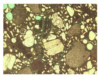
Figure 1. Optical transmission micrograph of Artopierre mortar. Image width is 4 mm.
