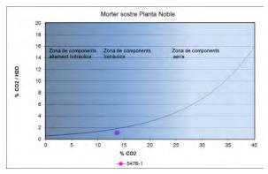
Figure 10.  $CO_2$  to structurally bound water ratio in relation to %  $CO_2$
