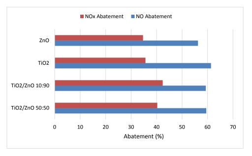
Figure 5. NO abatement values of  $\text{TiO}_2,$  ZnO and the two heterostructures.
