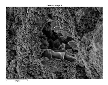
Figure 7. SEM image of a charcoal aggregate embedded in the carbonate-based binder of sample SM-28-3.
