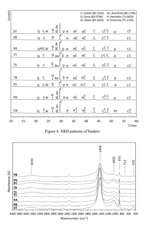
Figure 5. FTIR spectrum of binders
