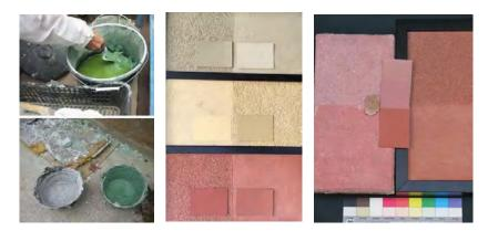
Figures 8a, 8b and 8c. Making up of coloured stucco palettes with chromatic controtype.
