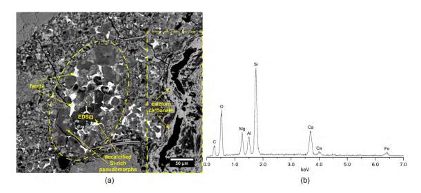
Figure 5: SEM-EDS analysis of specimen ATB: (a) residual cement grain (marked by oval) showing pseudomorphs of belite and alite that are surrounded by finely crystalline ferrite. Precipitation of calcium carbonate lining a crack can be seen on the right (marked by rectangular). (b) Exemplary EDS analysis of a pseudomorph of former calcium silicate constituent indicating the depletion in calcium.
