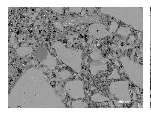
Layer1: finishing mortar M1
