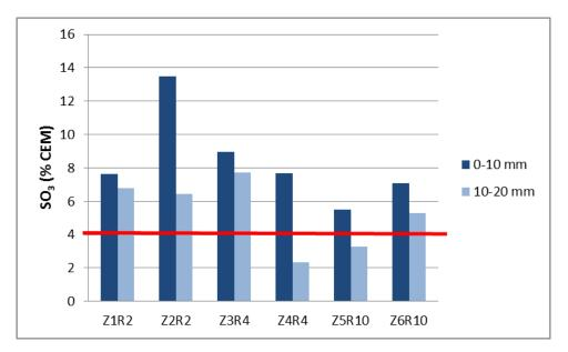
Figure 13. Sulphate concentration (% CEM) per zone elevation on the façade ( $R2 = 2^{nd}$  floor,  $R10 = 10^{th}$  floor) and depth. [10]
