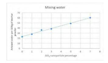
Figure 2. The quantities of mixing water used for mortars of various nanoparticle concentrations
