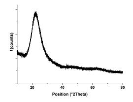
Figure 4. X-Ray diffraction diagram of employed SiO<sub>2</sub> nanoparticles. Peak height is approx. 2000 counts.
