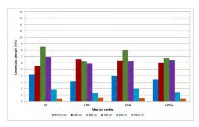
Figure 7. Compressive strength of the mortar compositions at elevated temperatures (28d)
