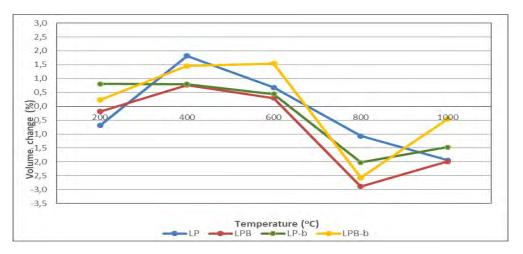
Figure 5. Volume change of the mortar specimens at elevated temperatures (28d)
