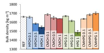
Figure 2. Bulk densities of the specimens 90 days old.Flexural and compressive strength
