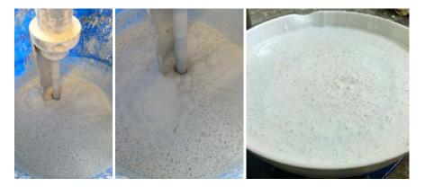
Figure 3. Extreme foaming of ready-mixed grouts (Ledan TB1) in the high speed mixer (left and middle image) and after Hobart mixing of standard grout quantity (image on the right).
