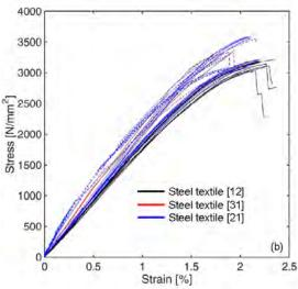
Figure 2. Stress-strain tensile response curves of dry textile
