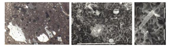
Figure 7. Gypsum plasters from Kalavasos-Ayios Dhmitrios. Thin section and photos from SEM
