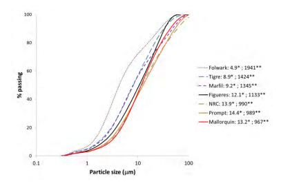
Figure 2. Particle size distribution \*  $D_{50}$  (mm); \*\* Specific surface area (m<sup>2</sup>/kg)
