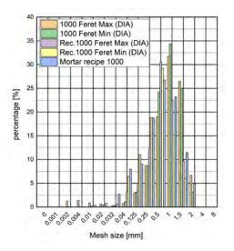
Figure 15. Comparison between the recipe and the reconstructed mortar. (Fraunhofer IBP, 2019)
