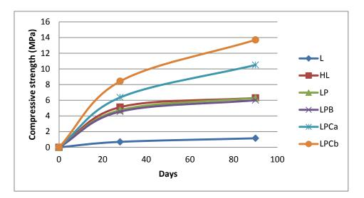
Figure 7. Rate of strength development of experimentally studied mortars (B/A=1:2.5-1:3)
