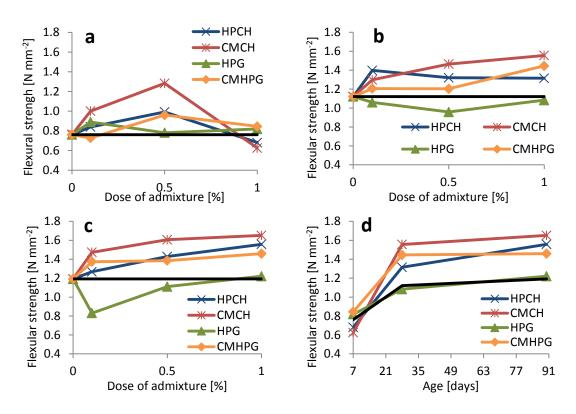
Figure 3. Flexural strength of studied specimens in the age of 7 days (a), 28 days (b), and 90 days (c) and time evolution of strength of samples with 1% of admixture (d).
