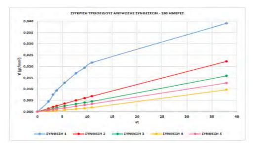
Figure 3 Capillary absorption of the mortar specimens at 180d age
