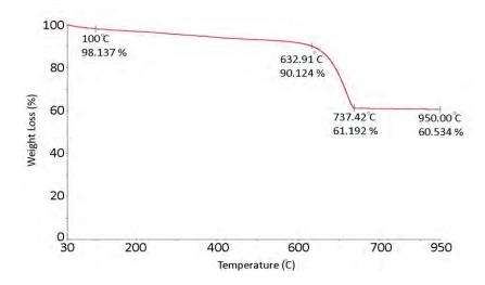
Figure 7. TGA spectra of binder (XT)
