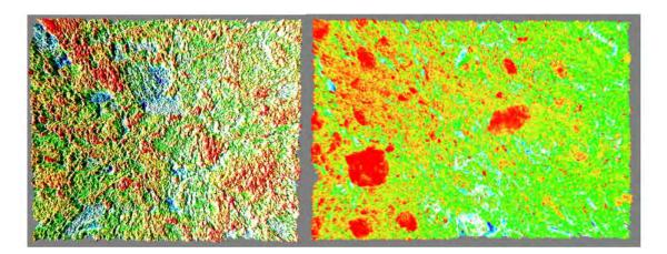
Figure 8. Comparison of two samples of Idanha-a-Velha, where on the left microphotograph is a lime mortar, while on the right a clay plaster is presented. In both cases, a surface scanner and a thermal spectral treatment have been developed.
