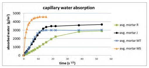
Figure 6. Capillary water absorption of the repair mortars (each point in the curve is the average value of 3 specimens)
