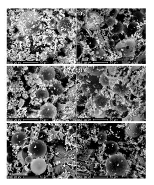
Figure 2. Broken section; backscattered electron image (BSI) of grout (a) C, (b) AL, (c) C\_Q, (d) EA\_Q, (e) AL\_C\_Q, (f) AL\_EA\_Q
