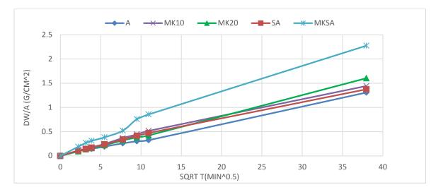
Figure 3. Capillary absorption of specimens at 28 days.
