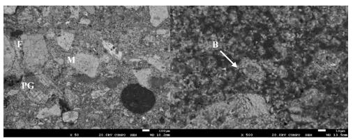
Figure 18. Microphotography by SEM. Identification of Feldspars (F), plagioclase (PG) and a lump of calcined marl (M). We can also see unhidrated belite cristals (B) inside a lump of calcined marl.
