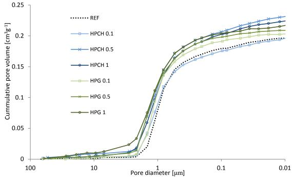
Figure 5. Cummulative pore volume curves of 28 days old specimens with HP derivative.
