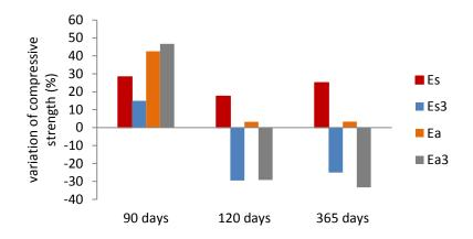
Figure 2. Variation of compressive strength (%) of nano-modified calcareous clay, in respect to the reference.
