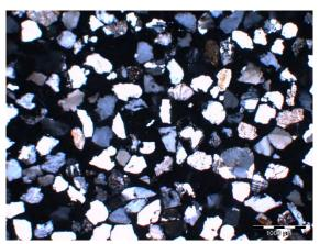
Figure 4f – Cast sample of aggregate. XPL.
