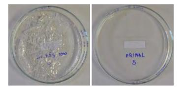
Figure 3. Silres BS OH 100 on the left and Primal E330S on the right after drying in a petri dish
