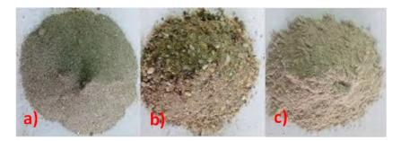
Figure 2. Component materials: a) aggregate F, b) aggregate C, c) natural zeolite
