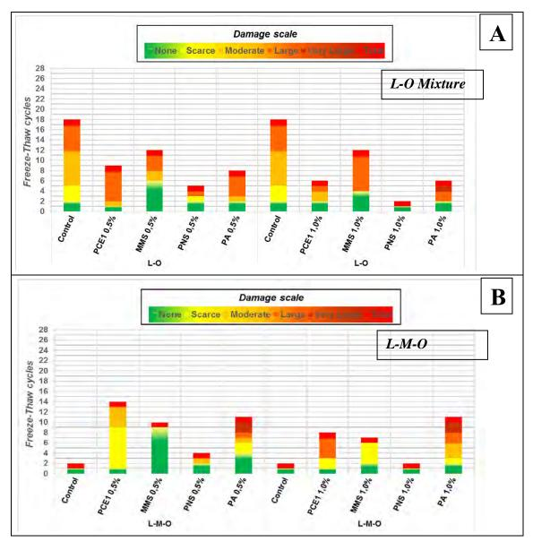
Figure 10. Alteration degrees of grouts after freeze-thaw cycles.
