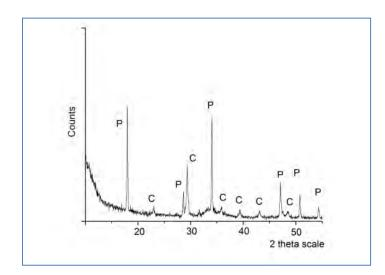
Figure 2. Representative X-ray diffraction pattern of the produced particles of the bottom-up methodology
