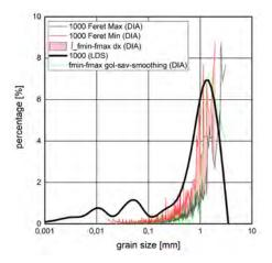
Figure 12. Comparison the results of the grain size distribution between DIA and LDS (Fraunhofer IBP, 2019)
