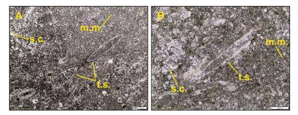
Figure 4. A. Microscopic character of the Dvorce-Prokop lm. fragment found in the sample PHA 3b-s. B. Example of microscopic structure of the Dvorce-Prokop lm. from the historic quarry in Prague-Bráník with marked micritic matrix (m.m.), sparitic cement (s.c.) and tentaculite shales (*Styliolina* sp.) (t.s.). Both in PPL.
