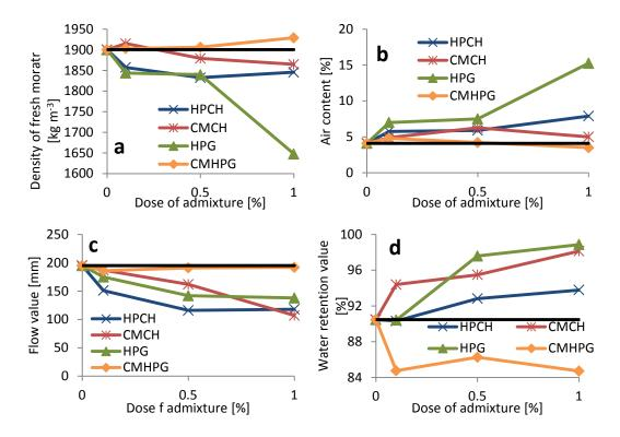
Figure 1. Fresh state properties of the NHL 3.5 mortars with admixtures.
