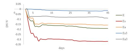
Figure 6. Volume change of binders from demolding up to 45 days.
