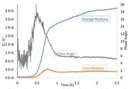
Figure 9: Storage modulus, loss modulus and phase angle against time for 10% Brick Dust at 40  $^{\circ}C$
