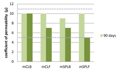
Figure 3. Variation of water vapour inflow and outflow at 90 days
