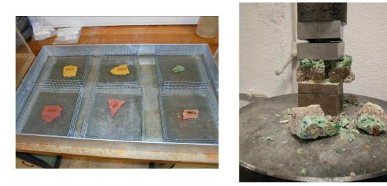
Figure 6. Physical and mechanical testing: a) Water absorption by capillarity; b) Compressive strength
