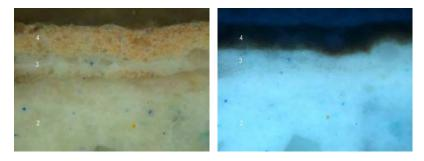
Figure 16a. Stratigraphic cross section of the wall's coating: 2.-original lime and blue and green pigment's stucco; 3-superimposed white primer layer; 4-current finish ocher painted. Figure 16b. Same as before, with UV light for organic compounds.
