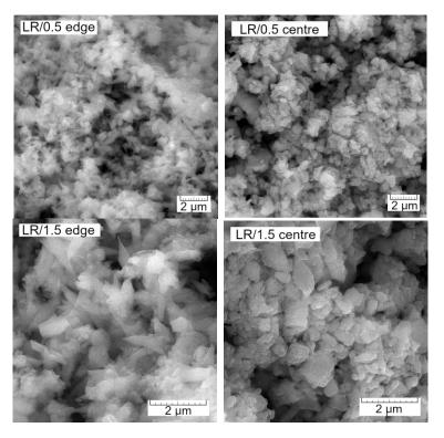
Figure 8. SEM photomicrographs of LR paste with 90 days of age taken close to the exposed surface (edge) and in the centre of the specimen.
