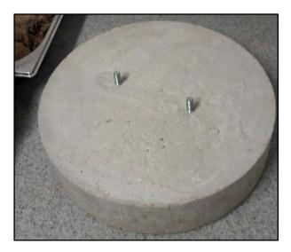
Figure 2. Cast concrete slab prior to use in the modular slab experiment.
