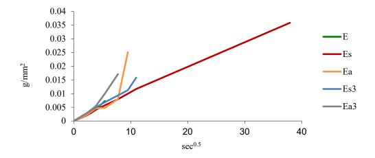
Figure 4. Influence of nanoparticles on capillarity of nano-modified calcareous clay at 90 days.
