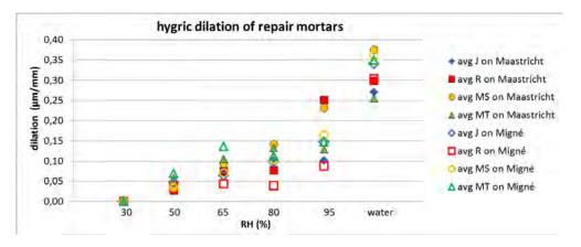
Figure 8. Hygric dilation of repair mortars prepared on Maastricht and Migné limestone)
