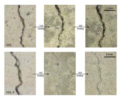
Figure 4. 200  $\mu m$  crack healing observation at the stereomicroscope
