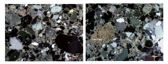
Figure 2. (a)- Images of transmitted light microscopy showing quartz (Q) and feldspar (F) aggregates and a carbonated matrix (b)- Micrograph showing the presence of lime lump
