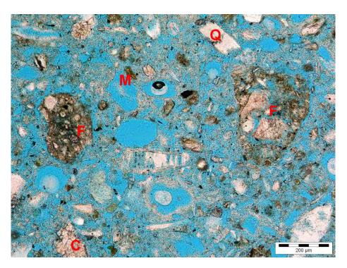
Figure 6: Thin section of plaster A under plane-polarized light, the binder is gypsum, aggregates are quartz (Q), soil fragments (F), coarse grained calcite (C) and brown micas (M)
