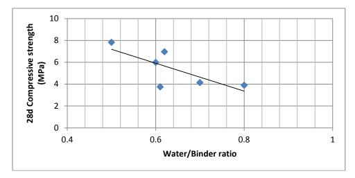
Figure 2. Relationship of 28-d compressive strength to Water/Binder ratio, Binding system= Hydraulic lime NHL3.5, Binder/Aggregate ratio (B/A)=1:2.5-3.0
