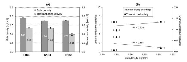
Figure 5. (A) Bulk density and thermal conductivity; (B) Bulk density vs. linear drying shrinkage and vs. thermal conductivity.
