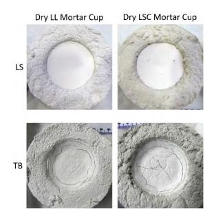
Figure 4. Reference mixtures LS and TB after drying in lime (LL) and lime-cement (LSC) mortar cups.
