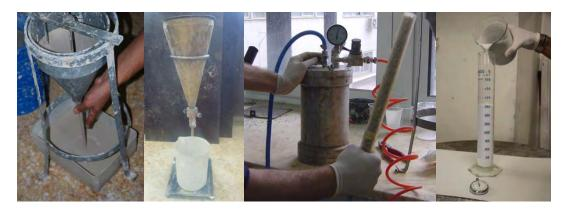
Figure 2. Fresh state properties testing. ASTM and EN flow cones (left), sand column test (middle), volume stability test (right).
