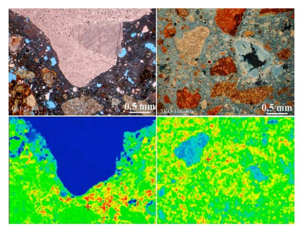
Figure 6: OM image (upper) and FTIR image (lower) of a lime-pozzolana mortar,  $2^{nd}$  century, Ostia Antica (Italy) (Left) and a lime-ceramic mortar, late Antique, Školarice, Slovenia (Right). Note differing locations and density of reaction products (red/orange in the FTIR maps) and clearly identifiable reaction rings in the right sample. Bands as described in text.
