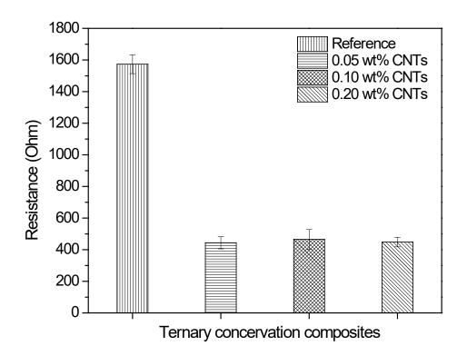
Figure 4. Electrical properties of water saturated ternary mixtures after 7 days setting/hydration time.
