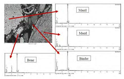
Figure 4a. SEM image of an area of Type A mortar sample TWO.04, with associated EDS spectra for two *maerl* fragments of varying textures, one probable bone fragment and the supporting matrix. Scale bar 500µm; SEM Image John Hughes.
