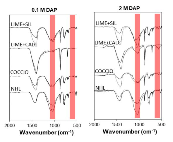
Figure 2. FT-IR spectra of untreated samples (dashed lines) and samples treated for 24 hours (solid lines). The position where HAP bands are expected is highlighted in red.
