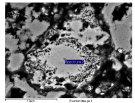
Figure 7. DRX spectrum of the binder Figure 8. Grain of the original binder showing a hidrated ring around an unhydrated core (image with back scattered electrons)
