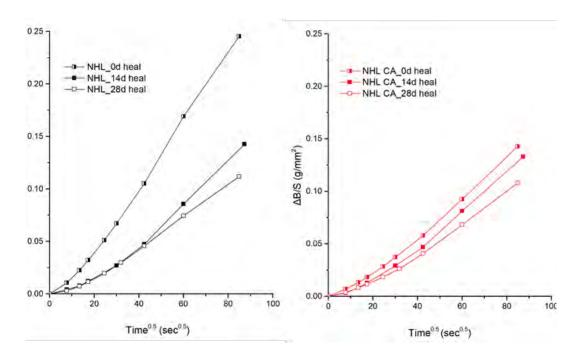
Figure 5. Water absorption by capillary through the crack after 0, 14 and 28 days healing period
