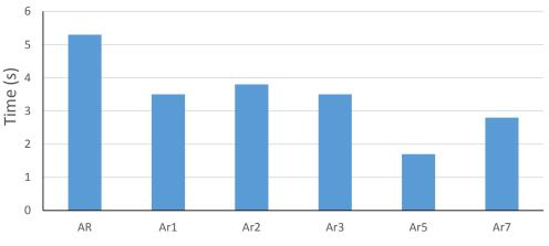
Figure 9. Water droplet absorption time for each mortar sample.
