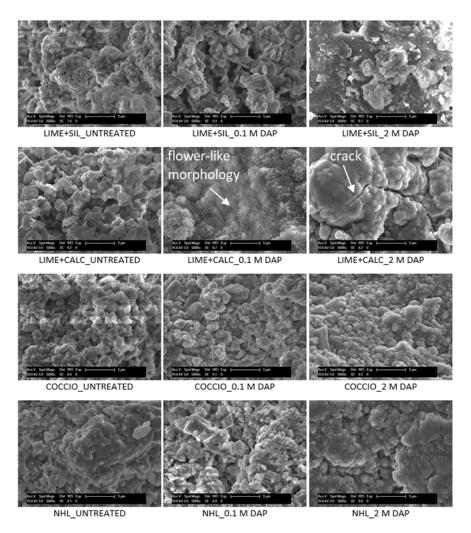
Figure 1. SEM images of untreated and treated samples (scale bar = 5  $\mu$ m).
