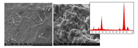
Figure 9. Crystalline formations observed in NHL-CA specimens after 28 days healing period
