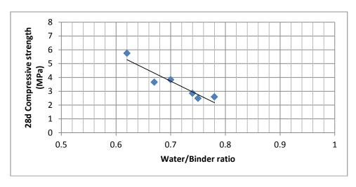
Figure4. Relationship of 28-d compressive strength to Water/Binder ratio, Binding system= Hydrated lime + pozzolan + brick dust (10-15% w/w of total binder), Binder/Aggregate ratio (B/A)=1:2.5-3.0
