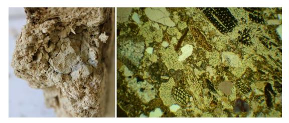
Figure 12. Clay mortars with organic fibers in an early 19<sup>th</sup> century render on a wooden house in Visby. Often it is of great importance to compare the mortar sample with the thin section to be able to make a correct interpretation. The width of the sample covers 2.65 mm. Illustration: Kristin Balksten [14].
