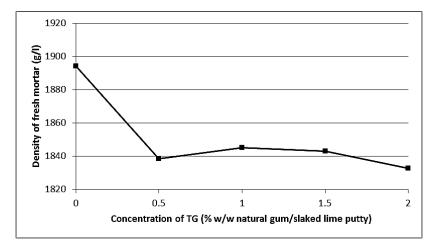
Figure 3. Density of the fresh mixtures vs. concentration of tragacanth gum (TG)
