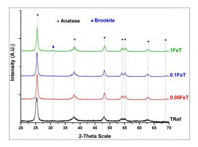
Figure 2. XRD patterns of the synthesized photoactive Fe-doped TiO<sub>2</sub> nanoparticles along with the TRef sample.
