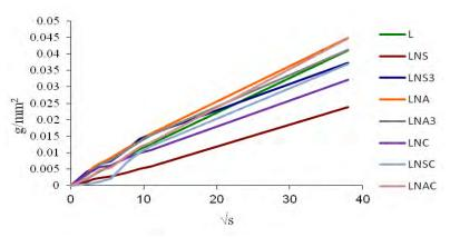
Figure 5. Capillary water absorption evolution of lime pastes at 28 days.
