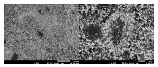
Figure 21. Microphotography by SEM. Detail of a lump of calcined marl with unhidrated belite crystals inside.
