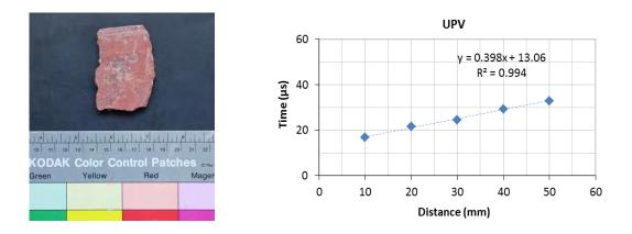
Figure 7. Determination of the UPV in sample IP2: image of the test specimen used (IP2.1) and graphical representation of the results
