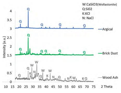
Figure 2: Representative Diffraction Patterns of raw materials
