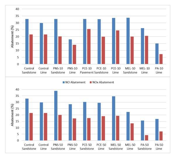
Figure 7. Effect of the different dispersing agents: NO and NOx abatement of the coatings prepared with TiO<sub>2</sub>/ZnO 10:90 (top) and 50:50 (bottom) photocatalysts.
