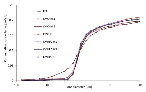
Figure 6. Cummulative pore volume curves of 28 days old specimens with CM derivative.
