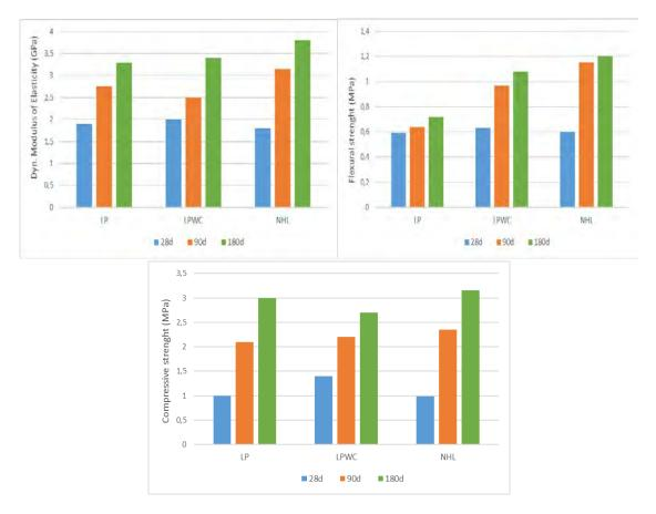
Figure 7. Mechanical properties of the grout compositions at the age of 28, 90 and 180 days
