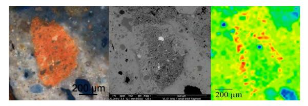
Figure 1. Left and Center: SM and SEM images of a ceramic aggregate; Right: FTIR image of the overlapping zones of carbonate and silicate. Scale: Red to Blue: 1.0-0.0. Roman hypocaust floor, Vindobona (Austria). (Previously Published in Weber & Baragona 2019 [3])
