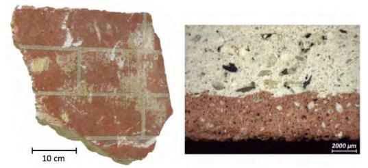
Figure 3: "False brick" render and cross section observed under microscope at the interface scratch coat/finishing coat (left) and on the finishing coat imitating brick (right). Building 1 rue Royale, Versailles, (1743).
