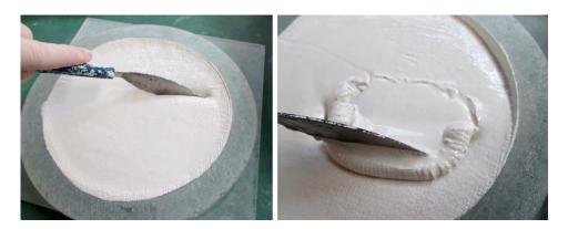
Figure 2. Checking the thickness of compact layer.
