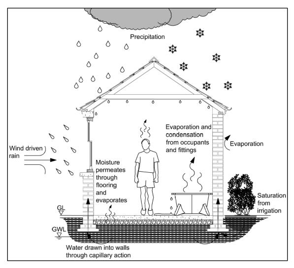
Figure 1. Moisture movement in and around buildings.
