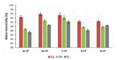
Figure 3. Water retentivity of the fresh mortar with the standard grain size distribution (CP).
