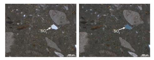
Figure 8: Sample S33 under optical microscope. Magnification 50x, PPT (left). Magnification 50x, XPT (right).
