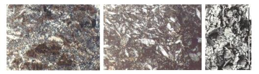
Figure 6. Gypsum plasters from Kalavasos-Tenta. Thin Sections and photo from SEM
