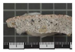
Figure 2. Cross-section of No. 2002, composed of a preparatory and a top layer. (Fraunhofer IBP, 2017)
