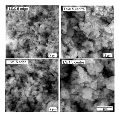
Figure 7. SEM photomicrographs of LS paste with 90 days of age taken close to the exposed surface (edge) and in the centre of the specimen.
