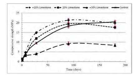
Figure 5. Compressive strength of NHL5 and NHL5-limestone-filled mortars over 180 days. COV 10% limestone=3-15%; 20% limestone=3-8%; 30% limestone 1-12%; 100%NHL5=4-14.
