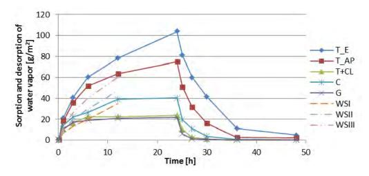
Figure 6. Sorption and desorption curves and sorption limits (WSI, WSII and WSIII) defined by DIN 18947 [22].
