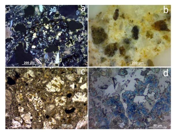
Figure 4 Typical residues in the samples between 1900 and 1908; a: large unhydrous cement grain consisting predominantly of C<sub>2</sub>S with few C<sub>3</sub>S crystals (A-1903, XPL), b: unhydrated cement grains in sample A-1907 matrix (IL/DF), c: cement residues in a terrazzo sample (H-1908, PPL), d: cement residue with coarse aluminate (grey), prismatic ferrite (white) and partially hydrated C<sub>3</sub>S and C<sub>2</sub>S (blue; H-1908, RL, Nital etch).
