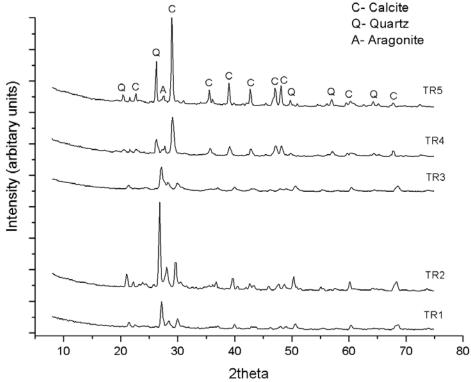
Figure 3: X-ray diffractogram of the historic mortar samples
