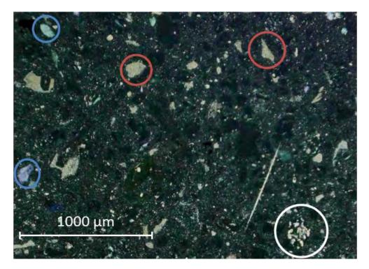
Figure 12: Observation under polarised light / crossed nicols of the finishing coat of the "Théâtre de la Renaissance », Paris, 1873. Quartz (blue circles), micritic calcite (red circles) and anhydrite II (white circle) can be observed.
