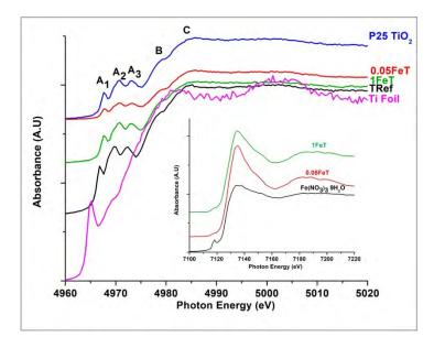
Figure 4. Ti K-edge (a) and Fe K-edge (b) XANES spectra for TRef, 0.05FeT, 0.1FeT and 1FeT nanoparticles. XANES spectra of Ti foil, TiO2-P25 and Fe(NO<sub>3</sub>)<sub>3</sub> 9H<sub>2</sub>O were used as references.
