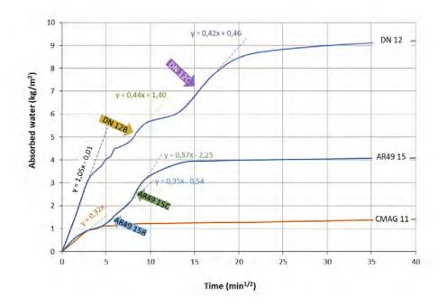
Figure 6. Absorbed water during time in multilayer samples
