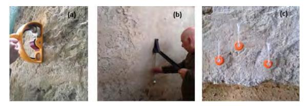
Figure 9 – *In situ* tests: (a) Pendular sclerometer in Bragança Terraces Residence wall section facing south; (b) Sphere impact test at a wall facing East inside Jogo da Pela Tower and (c) Karsten tubes test at a wall section facing East at Bragança Terraces Residence
