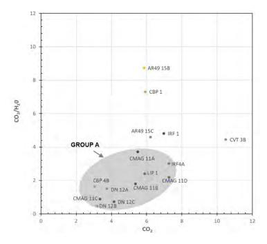
Figure 5.  $CO_2$  to structurally bound water ratio in relation to %  $CO_2$
