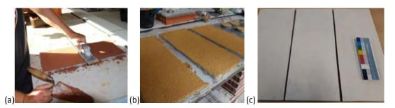
Figure 3.Finishing of planar specimen of T\_AP plaster (a) and planar specimens of T+CL plaster (b) and planar specimens of G plaster(c).
