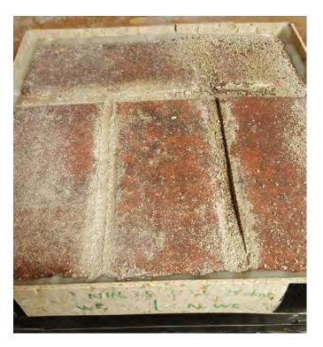
Figure 6. NHL 3.5 mortar with and without silane cream water repellent, after testing of 50 freeze-thaw cycles. The left side is treated with silane cream, the right side is untreated, 2017. Photograph by Chad Lausberg
