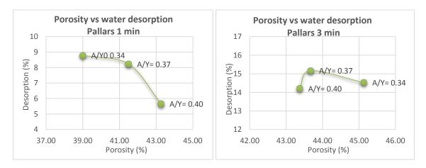
Figure 6. Pallars's gypsum graphics "Porosity vs water desorption" in a mixing time 1 and 3 minutes.
