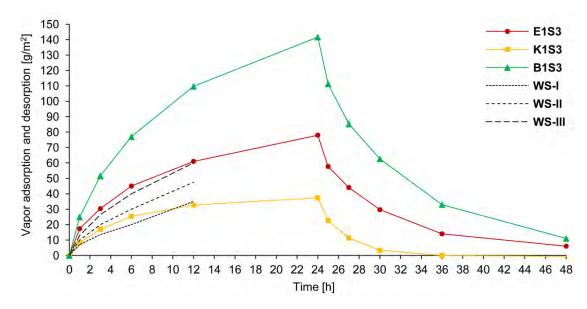
Figure 9. Vapour adsorption and desorption of plasters and vapour adsorption classes defined in DIN 18947 [3] (WS-I, WS-II and WS-III).
