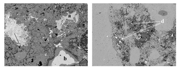
a: calcium aluminium  $C_4A$  type, b: calcium silicate  $C_2S$ , c: grain with  $C_2A$ , C-A-(S) and ferrite, d: decalcified  $C_2S$  in a cement grains
