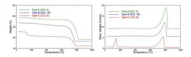
Figure 6. TGA (left) and DTG (right) curves of representatives of three categories of the binder enriched samples based on their thermal decomposition behaviour.
