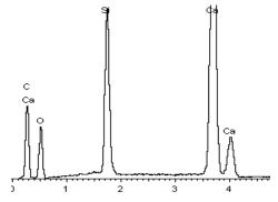
Figure 10. Elemental composition of the calcium silicate in Figure 9- probably belite.
