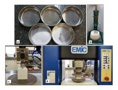
Figure 1. Gypsum plaster tests: a. Grain size tests: sequence of sieves and retained material; b. setting time using the Vicat apparatus; c. Hardness; d. compressive strength.
