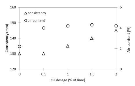
Figure 2. Influence of flax oil on consistency and air content of fresh mortar mix.
