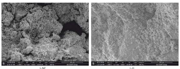
Figure 7. SEM overview of microstructure of L-Q and L-NZ render samples
