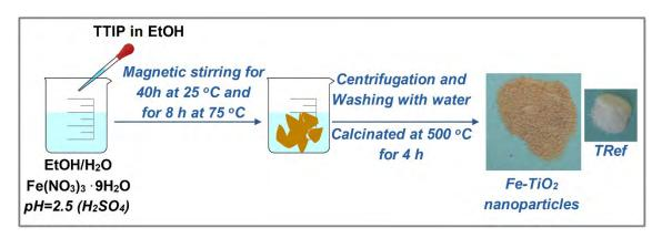
Scheme 1. The experimental procedure of the incorporation of Fe-ions within the TiO<sub>2</sub> matrix first and further their incorporation into the lime paste.
