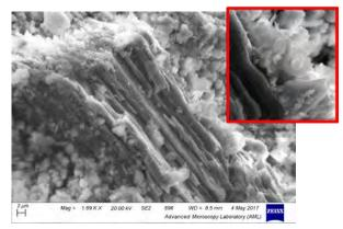
Figure 9. Calcium silicate clinker in a 30% limestone-filled paste with abundant plates (tending to hexagonal) and lower crystallinity phases at the interface.
