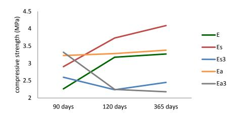
Figure 1. Evolution of compressive strength (MPa) of nano-modified calcareous clay, over time.
