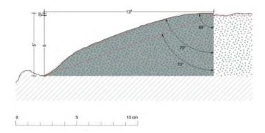
Figure 11. Cross section of an historical edge repair mortar. (Fraunhofer IBP, 2017)
