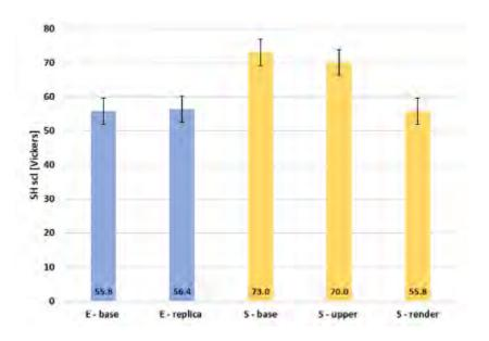
Figure 11 - Pendular sclerometer results in Bragança Terraces Residence
