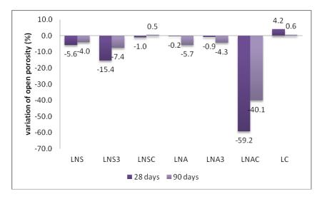
Figure 3. Open porosity variation (%) of nano-modified hydrated lime systems, in respect to the reference.
