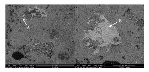
Figure 13. Microphotography by SEM. Identification of unhydrated belite (B) and alite (A) crystals.
