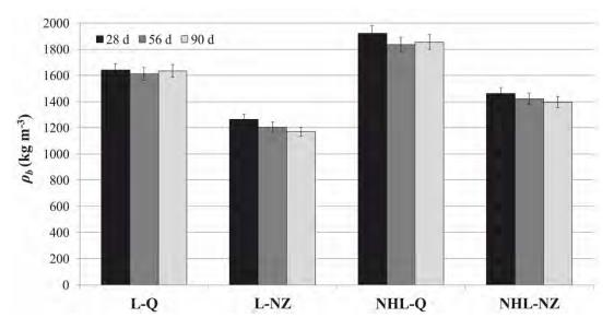
Figure 2. Bulk density of renders over time.
