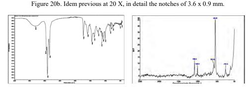
Figure 21a. FTIR spectroscopy of the organic compounds. Figure 21b. Raman spectroscopy for detecting soaps and pigments.
