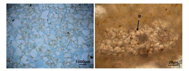
Figure 15. Thin section photomicroscograph. Incident light. The absence of lumps of calcined marls are observed. Thin section photomicroscograph; Trasmited light. Detail of unhidrated belite crystals (B).
