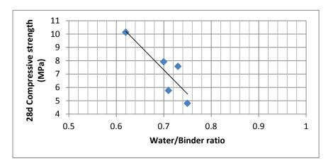
Figure6. Relationship of 28-d compressive strength to Water/Binder ratio, Binding system= Hydrated lime + pozzolan + white portland cement (20% w/w of total binder), Binder/Aggregate ratio (B/A)=1:2.5-3.0
