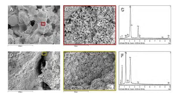
Figure 10. SEM/EDS analysis of sample F03 (fractured surface): (A) general sample view; (B) detail of the area marked in A corresponding to the lime paste; (C) EDS spectrum of the dolomitic lime binder paste; (D) aggregate interface showing hydromagnesite presence; (E) detail of the area marked in D showing hydromagnesite lamellar crystals; (F) EDS spectrum of hydromagnesite founded in E
