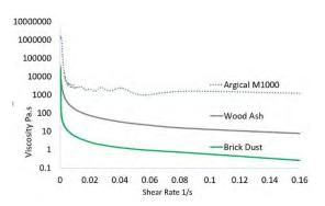
Figure 13: Viscosity against shear rate for Argical M1000, brick dust and wood ash
