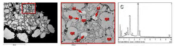
Figure 5. SEM/EDS analysis of sample B06: (A) general view of polished surface; (B) detail of the area marked in A showing quartz (qz) and feldspar (fp) aggregate grains and lime nodules (cl); (C) EDS spectrum of lime nodule in A
