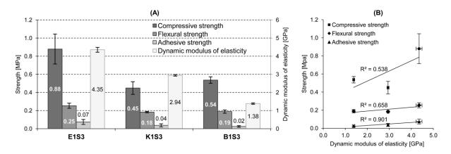
Figure 6. (A) Compressive, flexural and adhesive strength and dynamic modulus of elasticity; (B) Dynamic modulus of elasticity vs. compressive, flexural and adhesive strength.
