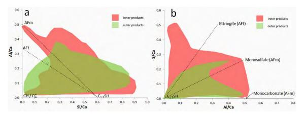
Figure 5 Atomic ratio plots showing the distribution of hydrate phases formed in the inner (red) and outer (green) products (sample A-1869; for explanation see text).
