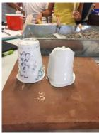
Figure 9 Lime paste test to verify correct texture for mortar mixture. TECTRAD INAH 2019
