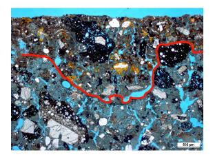
Figure 3. Thin section of mortar 1000 with the two layers. (Fraunhofer IBP/F. Schlütter, 2017)
