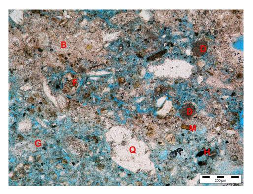
Figure 9: Thin section of plaster B in more detail under plane-polarized light, brownish areas (B) contain additional lime in contrast to light areas where only gypsum (G) is present as a binder, aggregates are quartz (Q), micas (M), dolomite (D), soil fragment (F), H = remains of charcoal
