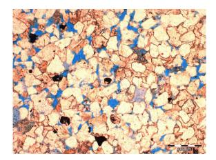
Figure 4e - Porous sandstone texture in PPL.
