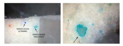
Figure 18a. OM with presence of known blue pigment and presence of green particles based on silicon. Figure 18b. OM at 80X of the translucent silicon green.
