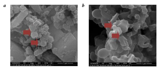
Figure 3. (a) Plate-like and of undetermined shape nanoparticles of Ca(OH)<sub>2</sub> (Exp01); (b) Hexagonal, spherical and of undetermined angular shape nanoparticles of Ca(OH)<sub>2</sub> (Exp02)
