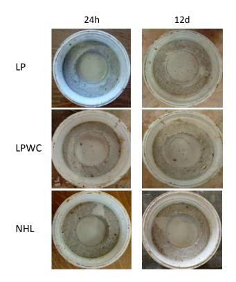
Figure 5 Drying shrinkage of the grout mixtures 24h and 12 days after their manufacture
