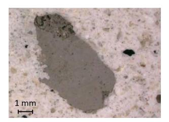
Figure 11: Microscope observation of a dolomite gain in the scratch coat of the "Moulin de Claye", Saint Rémylès-Chevreuse (1930).
