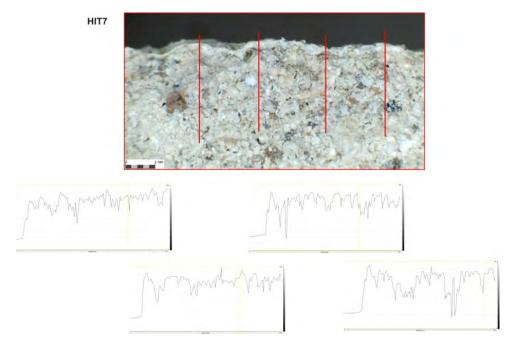
Figure 12. Vertical and random chromatografies of sample HIT7, where grey tones are showed in the graphics and the presence of carbonation hardness is reflected in a sudden drop of values.
