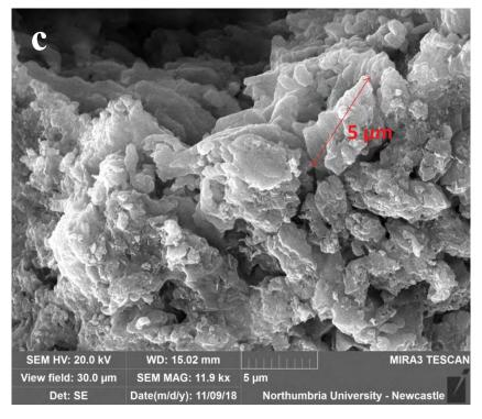
Figure 2. SEM photomicrograph of broken surface of a hard lump contained in the mortar.
