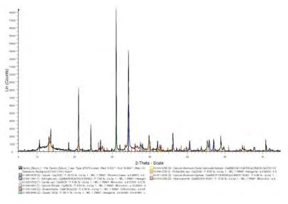
Figure 7. XRD analysis of a non-carbonated greyish concrete sample.
