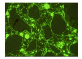
Figure 18. As mentioned, the pore structure is important for the function of use. A fluorescence photograph of a structure where the large dark green fields are aggregate, the speckled paste and the light green dots are air voids. Using this technique, the spacing factor, size and amount can be calculated. 4.8 x 3.1 mm. Illustration: Bo Nitz.
