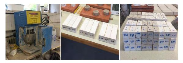
Figure 3. Preparation of test pieces for the mechanical tests according to the Standard Norm UNE-EN 13279-2.
