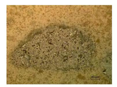
Figure 11. Large well crystallized clinker grain filled with small round beige C2S. Optical microscope view (G=X20) of the ochre render.
