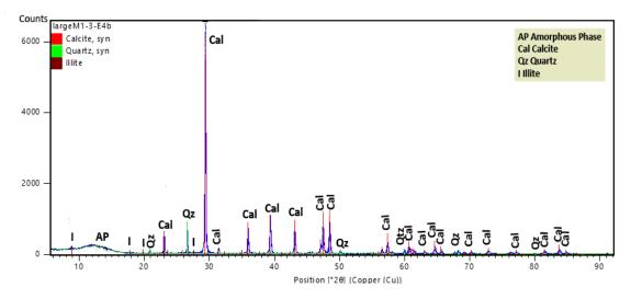
Figure 9. XRD pattern of mortar sample M1-3-E4b (ceiling).
