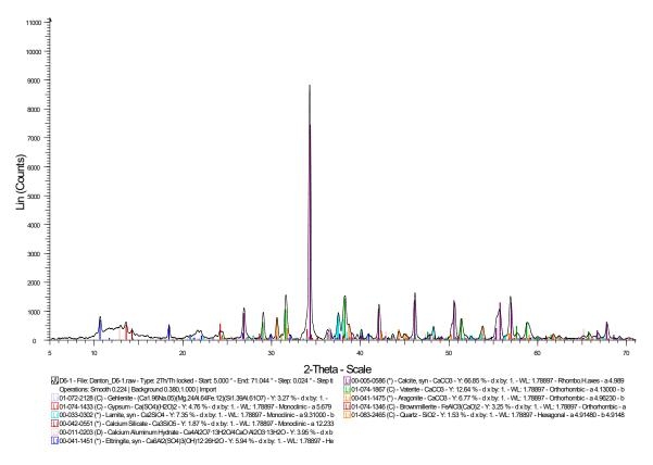
Figure 10. XRD analysis of a carbonated ochre render sample.
