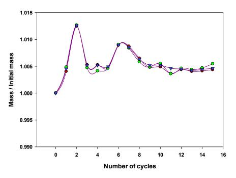
Figure 6. Mass loss of the specimens on salt weathering with sodium chloride solution
