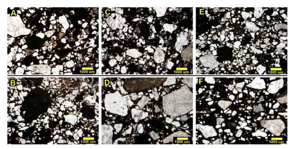
Figure 5. Petrographic observations (plain polars) of the two layer wall mortars. A) L1 layer of the AD-058 mortar. B) L2 layer of the AD-058 mortar. C) L1 layer of the AD-132 sample. D) L2 layer of the AD-132 sample. E) L1 layer of the mortar AD-134. F) L2 layer of the mortar AD-134
