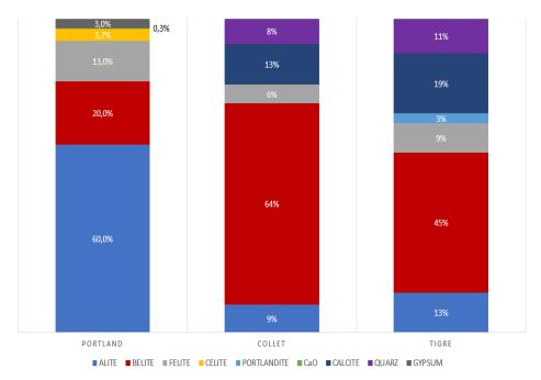
Figure 1. Mineralogical composition of unhydrated Portland and Natural cements .
