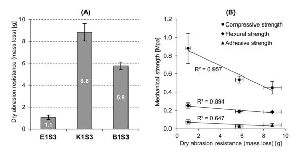
Figure 8. (A) Dry abrasion resistance (mass loss); (B) Dry abrasion resistance (mass loss) vs. compressive, flexural and adhesive strength.
