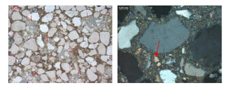
Figure 1. Left: Microphotograph of the microstructure of repair mortar R, showing the presence of large voids and locally lack of compactness (after 28 days of curing in outdoor conditions; parallel polarized light. Right: Microphotograph of a detail of the binder of mortar R, showing the presence of limestone powder (after 28 days of curing in outdoor conditions; crossed polarized light).
