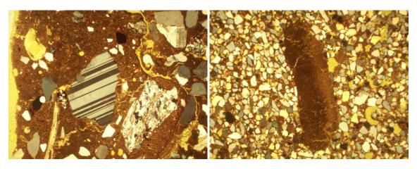
Figure 10. Difference in mineralogy, shape of the grains and sand curve is illustrated by samples with a medieval lime mortar and a 19<sup>th</sup> century lime mortar. The width of each sample is equivalent to 4.5 mm. Illustration: Kristin Balksten.
