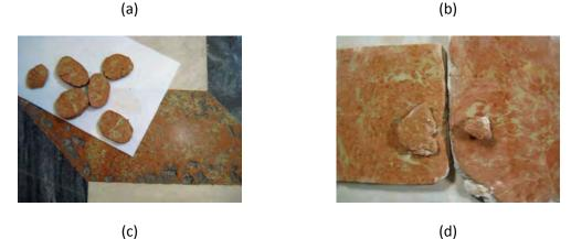
Figure 5. Preparation of stucco marble pastes: (a) mixing the gypsum plaster with the kneading water; (b) selecting different colours to obtain a similar esthetical effect; (c) final mixes before curing; (d) two pieces of limestone above the two recipes of stucco marble selected
