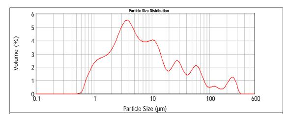
Figure 2. Particle size of metakaolin used.
