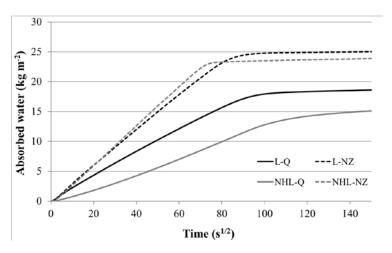
Figure 5. Cumulative mass of capillary water action versus time for studied renders.
