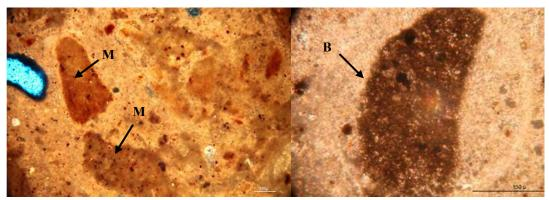
Figure 6. Thin section photomicroscograph. Trasmited light. Detail of a lump of calcined marls (M) and the unhidrated belite crystals (B).
