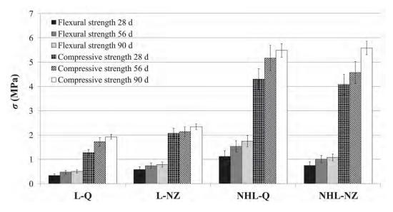
Figure 3. Flexural and compressive strength of renders over time.
