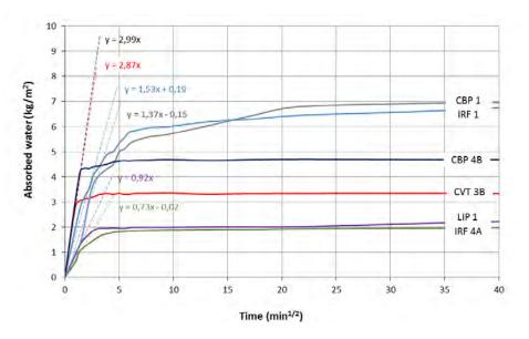
Figure 7. Absorbed water during time in single layer samples
