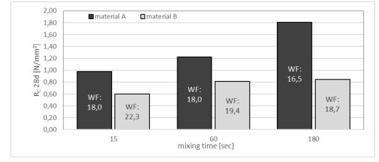
Figure 3. Compressive strength  $R_c$  after 28 d curing as a function of mixing time and water content [%] (water values inside the bars, standard deviation of strength see Table 5).
