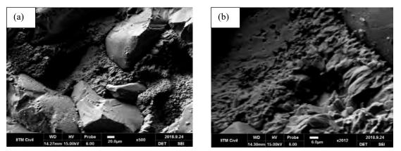
Figure 4. a) SEM image of coral stone at 500 X showing sand grains and pore filling Calcite b) SEM image at 2000X showing Magnesium Calcite formation
