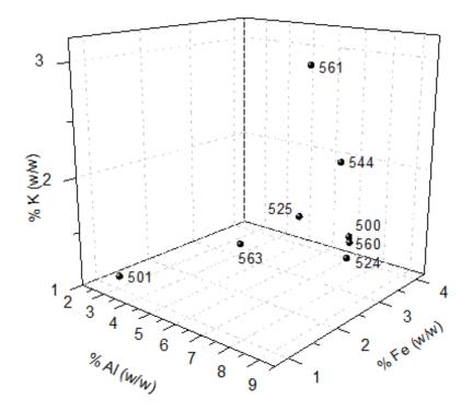
Figure 7. Clustering of samples in a tridimensional space on the basis of their concentration of elements typical of soil (Al, K and Fe).
