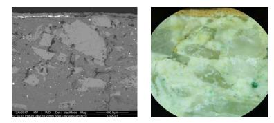
Figure 17a. Same sample as before, SEM observation, where the light points correspond with pure silicon. Figure 17b. OM at 80X of the same sample: lime stucco with blue pigment micro-nodules and presence of green pigment.
