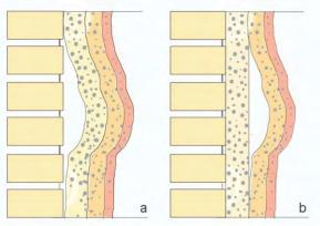
Figure 2. Schematic design of the mortar substrate's detachments. a. detachment between the mortar layers and the masonry, b. detachment in the interface of the mortar layers
