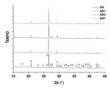
Figure 5. Selected XRPD diffraction patterns for the test samples. Maximum peak heights are approx. 200000 counts for all mortars. The main Bragg peaks for phases are indicated (P = portlandite, Q = quartz, CS = calcium silicates, V= vaterite, C = calcite, A = aragonite).
