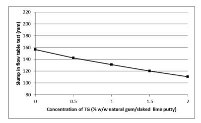
Figure 2. Slump results in flow table test vs. concentration of tragacanth gum (TG)
