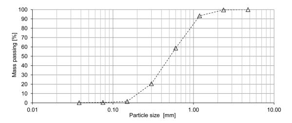
Figure 2. Particle size distribution curve of sand S by dry sieving.
