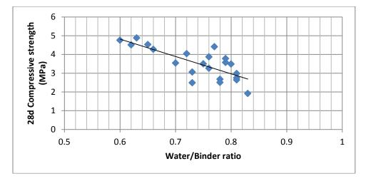
Figure3. Relationship of 28-d compressive strength to Water/Binder ratio, Binding system= Hydrated lime + pozzolan, Binder/Aggregate ratio (B/A)=1:2.5-3.0
