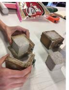
Figure 14 Plywood molds for mortars. TECTRAD INAH 2019
