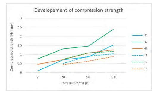
Figure 11. Diagram of compressive strength measurement of HAM and Hot-mixed mortars
