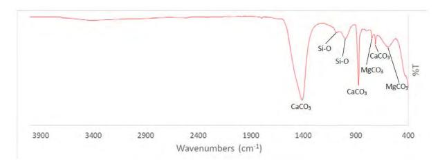
Figure 4. Infrared spectrum of a hard lump.
