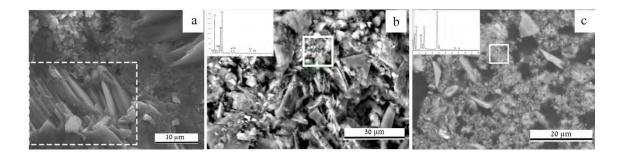
Figure 3. a) SEM image of mortar sample from the Alhaman at Kom El-Dikka (portlandite plates are marked) and b) ESEM image of mortar sample from the *Natatio* at Labraunda ESEM image of mortar sample from Snow Well at Augusta Emerita (EDS are from the square from the binder)
