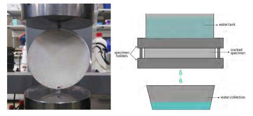
Figure 2. Splitting test of cylindrical specimens for water permeability measurements (left) and water permeability test setup (right).
