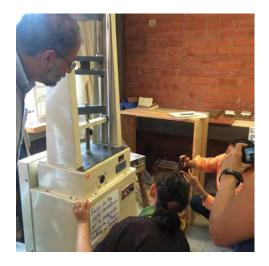
Figures 18 & 19. Compression strength tests as an indicator between lime and formulated lime mortars. TECTRAD INAH 2017.
