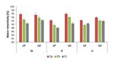
Figure 4. Water retentivity of the fresh mortars with different grain size distributions.
