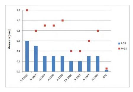
Figure 1. Distribution of average (AGS) and maximum (MGS) grain sizes of residual cement grains in the samples compared to that of modern Ordinary Portland cement (OPC)
