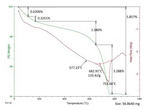
Figure 10. Thermal degradation curve of brick sample M2-2-8a
