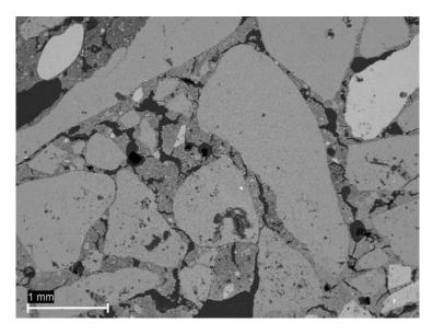
Figure 5: Shrinkage cracks in the matrix of the test mortar sample (SEM-BSE)
