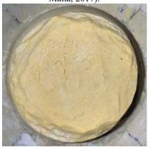
Figure 5: Shrinkage testing. A CaLoSiL-based microgrout exhibiting cracking after application and setting in a Globigerina cup (Department of Conservation and Built Heritage, University of Malta, 2017).
