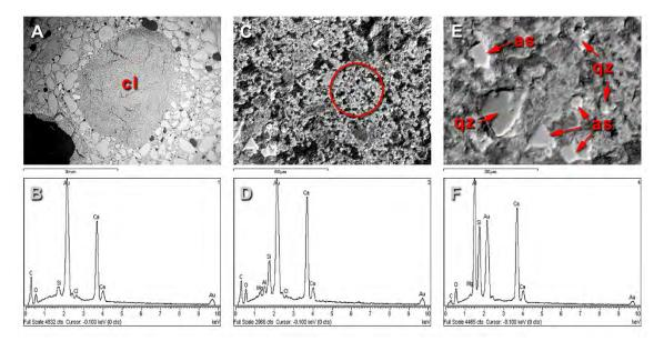
Figure 8. SEM/EDS analysis of sample C08 (polished surface): (A) General view showing the aggregates distribution and a lime nodule (cl); (B) EDS spectrum of the calcite nodule founded in A; (C) close up view showing the lime paste; (D) EDS spectrum of the binder zone marked in C; (E) details of the paste showing quartz aggregates (qz) and calcium aluminium silicates (as); (F) EDS spectrum of the calcium aluminium silicates founded in E
