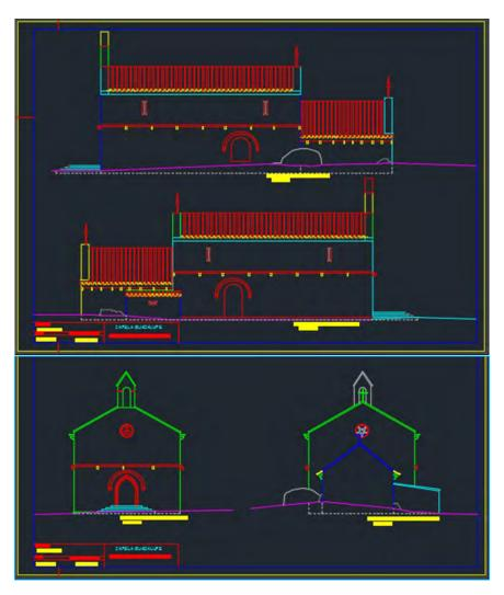
Figure 6. Architectural plants of the 4 facades of Guadalupe Church demonstrating different terrain elevations with lower height on the chapel that on the main entrance. ©João Sandes
