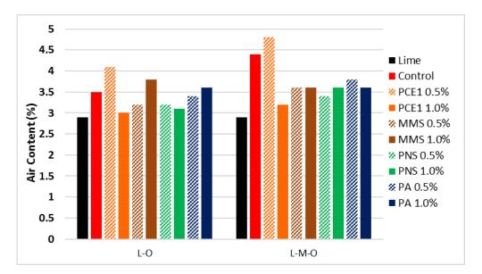
Figure 2. Air content in the different mixtures
