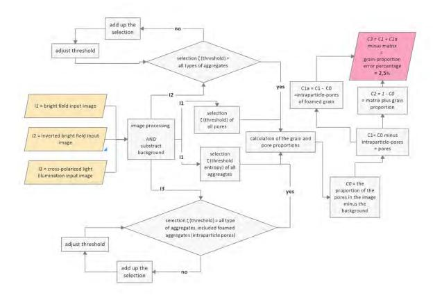
Figure 10. Procedure of the DIA. (Fraunhofer IBP, 2019)
