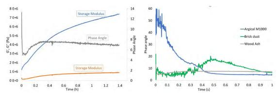
Figure 10: Storage modulus, loss modulus and phase angle against time for 10% Wood Ash at  $40^{\circ}$ C
