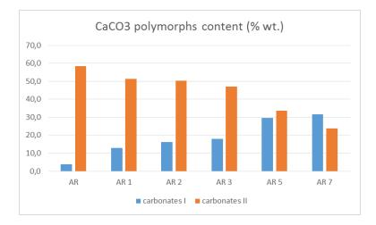
$\label{eq:second} Figure \ 6. \ Representation \ of \ individual \ CaCO_3 \ polymorphs. \ Carbonates \ I - metastable \ modifications, \ carbonates \ II - calcite.$
