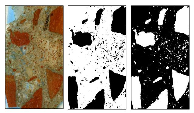
Figure 4. Section of the thin section of sample CA2 (left), brick fragments marked in black (center), binder marked in black (right). Image width approx. 17 mm.
