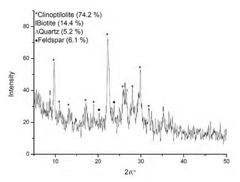
Figure 1. Mineralogical composition of zeolite (XRD analysis)
