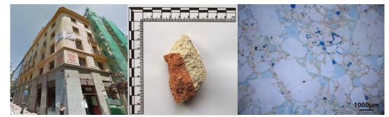
Figure 8. Facade of the bluiding. Thin section photomicroscograph. Incident light. Absence of lumps of calcined mars.
