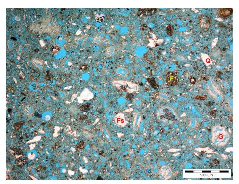
Figure 5: Thin section of plaster A under plane-polarized light, the binder is gypsum, partly recrystallized (G), aggregates are quartz (Q), feldspars (Fs) and soil fragments (F)
