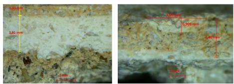
Figure 20a. OM cross section of the sgraffito at 10X: Layers of rendering, first layer and coloured finish layer.
