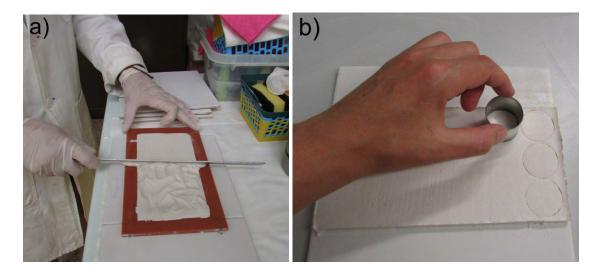
Figure 1. Preparation of the samples: a) spreading of the paste using a frame to obtain an even thickness; b) cutting of the fresh paste with a ring to obtain circular tablets.
