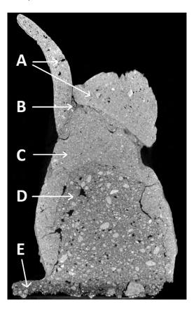
Figure 6. CT model cross section of the fruit piece No. 118. It shows the structure of stucco pieces including: A – small decorations, B – adhesive mortar I (fine), C – outer stucco layer, D – inner modelling mortar, E – adhesive mortar II (coarse).
