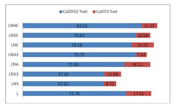
Figure 4. Calcite and calcium hydroxide content wt% of nano-modified hydrated lime systems, in respect to the reference at 28 days.
