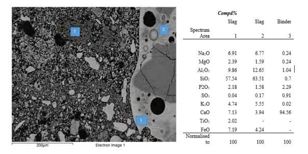
Figure 4d. SEM image of Type B mortar sample TWO.08. Numbered areas relate to EDS analyses in adjacent table. Scale bar 200µm; SEM image John Hughes.
