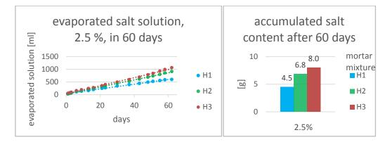
Figure 10a+b: diagram with evaporated salt solution after 60 days and table with the accumulated salt content
