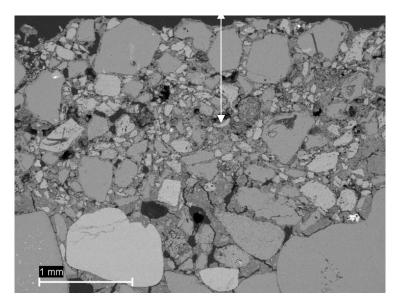
Figure 6: Finishing coat (arrow) at the top of the render layer (SEM-BSE)
