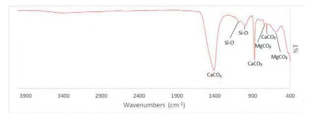
Figure 5. Infrared spectrum of a soft lump.
