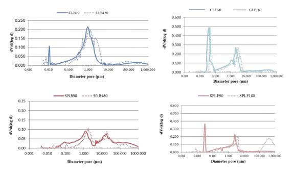
Figure 4. Pore size distribution of the different mortars at 90 and 180 of curing time by [13].
