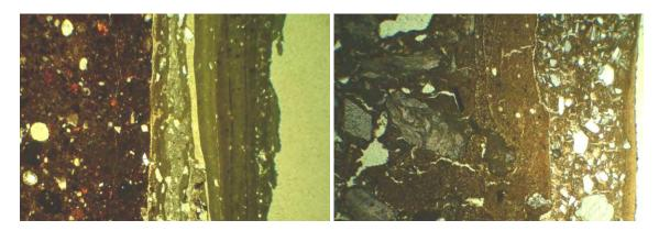
Figure 17. Mortars covered with a variation of paint layers; oil paint, lime wash, lime wash containing dolomite, and tempera. Also, adhesion between layers and compatibility can be considered from this kind of thin section analysis. The width of each sample is equivalent to 2.65 mm. Illustration: Kristin Balksten.
