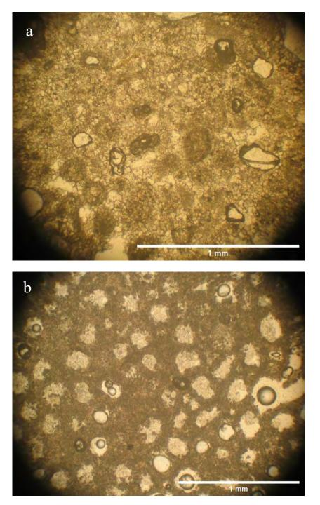
Figure 1. Optical microscope images of (a) crystalline oolitic dolostone and (b) part-burned dolostone showing oomoldic porosity.
