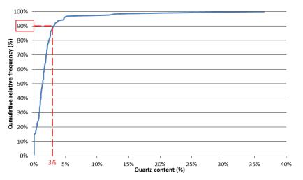
Figure 7: Cumulative relative frequency of analysed coats as a function of their quartz content.
