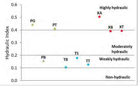
Figure 9. Hydraulic indexes of binders
