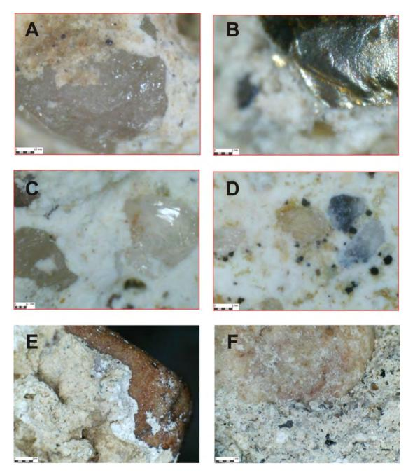
Figure 8. Different aggregates identified in the mortars of *Los Hitos*: A) Quartz in sample HIT3; B) Mica in sample HIT5; C) White and rose quartzes in sample HIT11; D) Small sizes aggregates with feldspar in sample HIT12; E) Piece of quartzite in sample HIT19; F) Sand and graves in concrete of simple HIT37.
