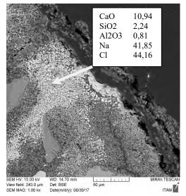
Figure 4. SEM micrograph – detail of NaCl deposits in the microstructure of the sample LpM (upper part), arrow points to area of EDS analysis
