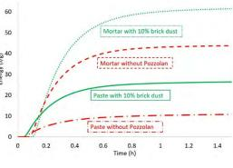
Figure 4: Energy graph for lime mortars and pastes with and without brick dust. Measurements taken at 40 ° C
