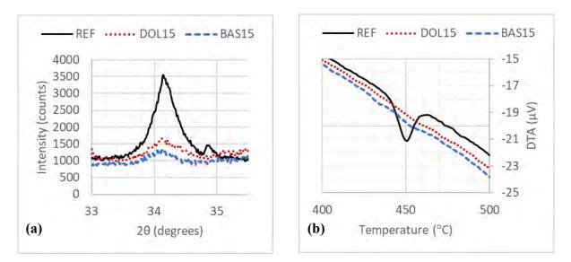
Figure 2: (a) XRD patterns of all mixtures showing the decrease in the intensity of the main portlandite peak ( $2\theta = 34.09^\circ$ ) with olivine basalt and dolerite addition; (b) DTA curves of all mixtures showing the elimination of portlandite (endothermic reaction at temperature ca. 400-500 °C) with olivine basalt and dolerite addition. All measurements shown were carried out 90 days after casting.
