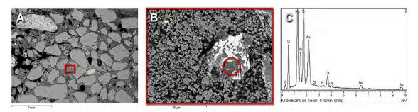
Figure 9. SEM/EDS analysis of sample F03 (polished surface): (A) general view showing aggregates and the porosity; (B) detail of the area marked in A with a particle of clinker silicate; (C) EDS spectrum of the clinker silicate marked in B
