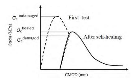
Figure 4. Schematic Stress- CMOD graph before and after healing after [27].
