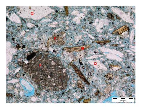
Figure 12: Detail of figure 13, thin section of relief plaster C under plane-polarized light, the binder is gypsum, aggregates are quartz (Q), soil fragments (F), and here frequently micas (M)
