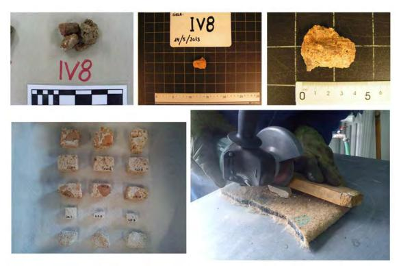
Figure 3. Sequence of preparing the IV8 sample.
