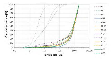
Figure 1. Particle size distribution of the raw materials.
