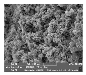
Figure 10. SEM image of the binder of sample SM-28-7. Needle-like crystals of aragonite are found within rombohedral calcite crystals.
