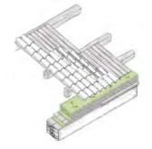
Figure 8. Ring beams reinforced with interposition in bed-joints of galvanized steel fiber strips
