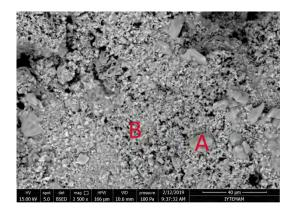
Figure 3. SEM images (2500x) of binder (B) and small size of aggregates (A) of the mortars
