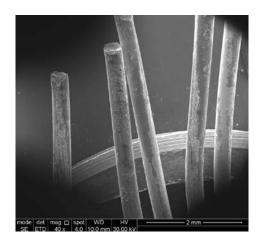
Figure 3. SEM image of the single filament
