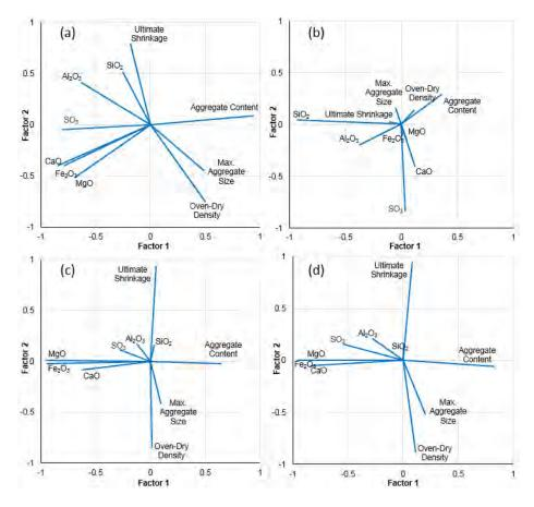
Figure 2. Factor loading plots for analysis 2, (a) no rotation, (b) Equimax rotation, (c) Varimax rotation, (d) Quartimax rotation.
