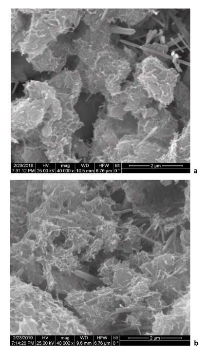
Figure 3. SEM photomicrographs of the binder matrix formed during setting in the reference mixture (a) and the LMC2 mixture, containing 0.2 wt% CNTs (b). The curved fibrous formations in the lower picture – having very similar morphology to the C-S-H hydration products – are attributed to CNTs. These are absent in the upper picture that depicts the hydrated matrix at the same magnification.
