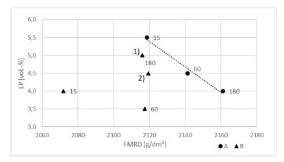
Figure 2. Plot of fresh mortar bulk density against air content for materials A and B at the different mixing times (repeat determination: measuring points 1) and 2)).
