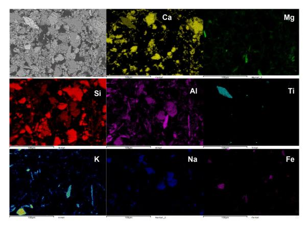
Figure 7: Detail of a marl fragment as aggregate in plaster A, thin section analysed by SEM/EDX, SEM backscatter image top left, elemental composition by EDX mapping
