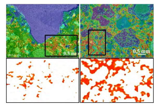
Figure 5: FTIR maps of the band corresponding to bound water (1720-1600 cm-1) overlaying scaled OM images of lime-pozzolana mortar. Left: 2nd century C.E., Right: 1930's restoration. Ostia Antica (Italy). Area of black rectangle is 1.5 mm2. The pixel density of the restoration mortar is 7.5 x that of archeological mortar. Scale (both): Red to Blue: 3.0-0.0.
