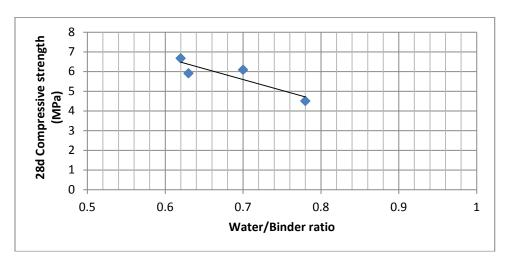
Figure 5. Relationship of 28-d compressive strength to Water/Binder ratio, Binding system= Hydrated lime + pozzolan + white portland cement (10% w/w of total binder), Binder/Aggregate ratio (B/A)=1:2.5-3.0
