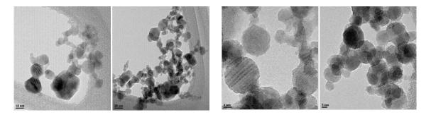
Figure 2. TEM micrographs (Left: TiO2/ZnO 50:50; rigth: TiO<sub>2</sub>/ZnO 10:90), showing a mixed morphology between the spherical one of TiO<sub>2</sub> and the elliptical one of ZnO.
