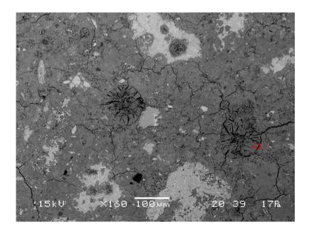
Figure 14. SEM view of the structural concrete revealing the presence of massive ettringite in the pores and in the cement matrix (G=X160).
