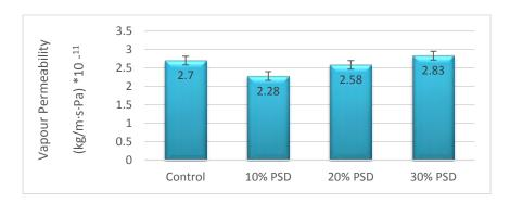
Figure 14. Water vapour permeability of NHL5 and NHL5/limestone mortars at 90 days. COV=8 (control); COV=3-8 (10-20%); COV=6 (30%).
