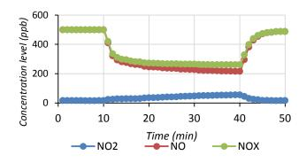
Figure 5. Profiles of NO, NO<sub>2</sub> and NO<sub>x</sub> abatements for mortar with 1 % percentage of 45PC6 superplasticizer and nanosilica-free (91 days hardening)
