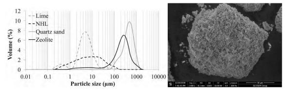
Figure 1. Particle size distribution of initial materials and SEM image of NZ aggregate.
