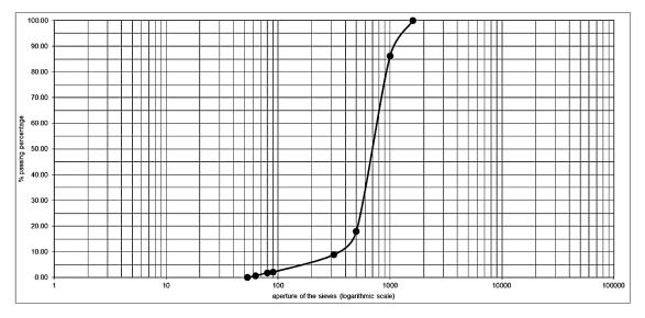
Figure 1. Granulometric curve of aggregate (the marble sand from Macael)
