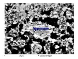
Figure 13. DRX spectrum of th binder Figure 14. Grain of the original binder showing a hidrated ring around an unhydrated core (image with back scattered electrons)
