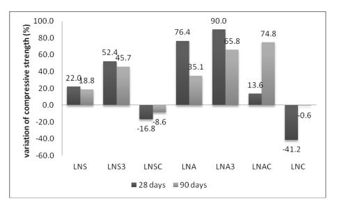
Figure 2. Variation of compressive strength (%) of nano-modified hydrated lime systems, in respect to the reference.
