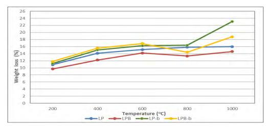
Figure 4. Weight loss of the mortar specimens at elevated temperatures (28d)
