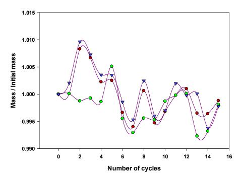
Figure 5. Mass loss of the specimens on salt weathering with sodium sulphate solution
