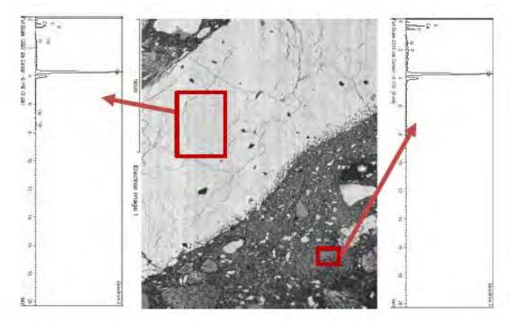
Figure 4b. SEM image of an area of Type B mortar sample TWO.08, with associated EDS spectra for an area of shell and supporting carbonate matrix. Scale bar 1mm; SEM image John Hughes
