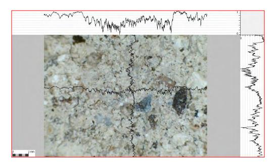
Figure 9. Colorimetry graphic of sample HIT1, showing saturation ratios where the presence of gravel is indicate through pronounced peaks.
