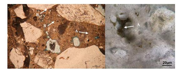
Figure 9. Thin section photomicroscograph. Trasmited light. Detail of unhidrated belite (B) and alite (A) crystals.
