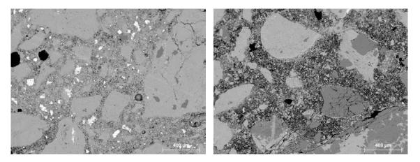
Figure 10. Microstructure and porosity within the finishing layer, sample M3, left: external area, right: near cracked interface with concrete
