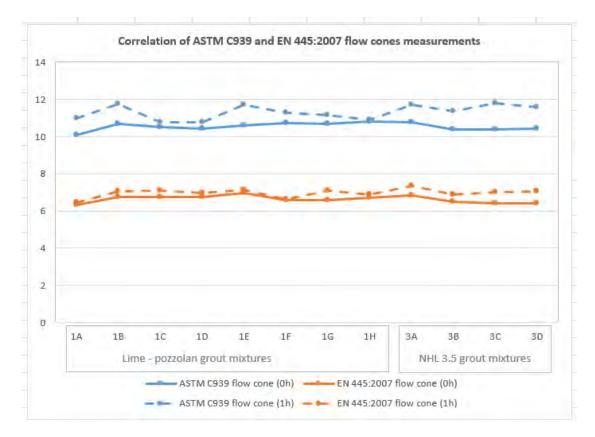
Figure 4. Correlation of ASTM C939 and EN 445:2007 flow cones measurements in the lime-pozzolan and NHL 3.5 grout mixtures.
