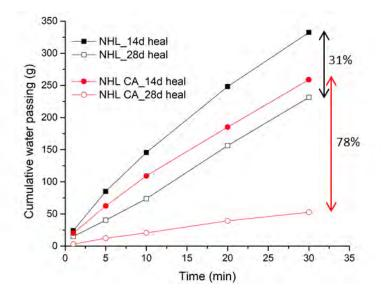
Figure 6. Cumulative water passing through the crack for the two mortar mixtures after 14 and 28 days healing period
