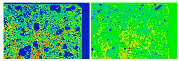
Figure 3 : Experimental Lime-Pozzolana Mortar. FTIR spectra associated with a reaction rim identified with SEM-EDX: Left image indicates highest density of the band, centered on 1663 cm<sup>-1</sup>. Scale: Red to Blue: 4.0-0.0. Right image indicates the highest density of the band centered on 955 cm<sup>-1</sup>. Scale: Red to Blue: 2.6-0.0.
