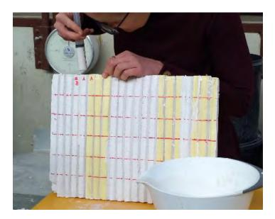
Figure 3. Flow on plastered tile with open and closed V-shaped channels.
