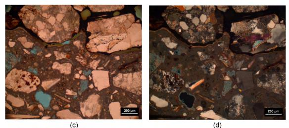
Figure 3: Exemplary micrographs of thin sections: (a) near-surface part of ATB showing a dark-brownish matrix with high content of aggregates as well as irregular formed voids (PPL), (b) same spot of sample ATB in XPL highlighting PCD, (c) near-surface part of B showing a dense dark-brownish matrix in contact with the above located bituminous mortar (PPL) and (d) same spot in XPL highlighting pore lining (calcite).
