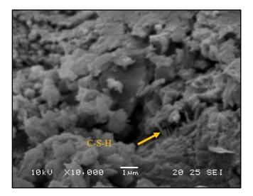
Figure 6. SEM image of the concrete sample showing signs of formed C-S-H.
