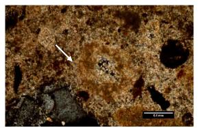
Figure 17. Thin section photomicroscograph. Trasmited light, crossed nicols. Detail of a lump of calcined marls with unhidrated belite crystals inside.
