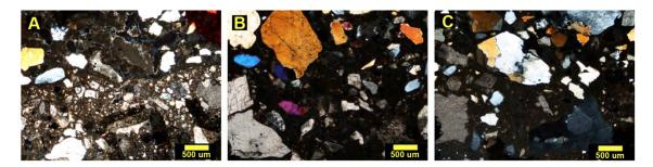
Figure 3. Petrographic observations (crossed polars) of marmolina layers. A) sample AD-124 with a:b>1. B) sample AD-134 with a:b <1. C) sample AD-243 a:b <1
