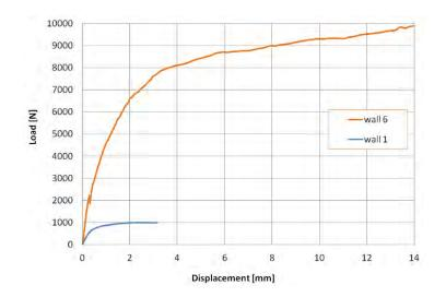
Figure 3. Load displacement behaviour of URM wall 1 and the lime render fibre-reinforced wall 6.
