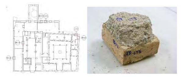
Figure 5. Plan of the building with marked areas where the samples were obtained from.
