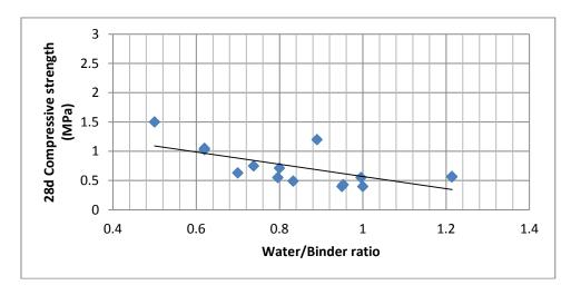
Figure 1. Relationship of 28-d compressive strength to Water/Binder ratio, Binding system= Hydrated lime CL90, Binder/Aggregate ratio (B/A)=1:2.5-3.0
