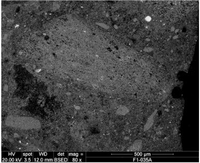
Figure 7. Microphotography by SEM. Detail of a lump of calcined marl.
