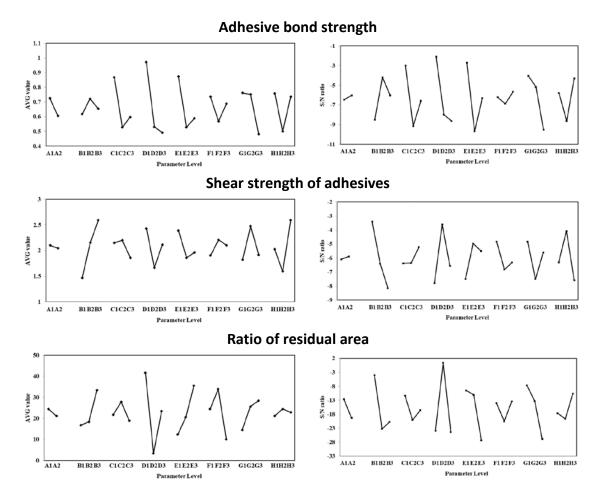
Figure 2. Factor response graph for average(AVG) values and the signal-to-noise (s/n) ratios for the adhesive bond strength, shear strength of adhesives and ratio of residual area
