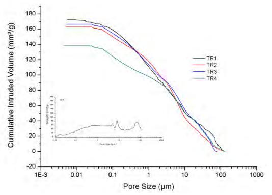
Figure 6. Cumulative and differential intrusion curve obtained from MIP analysis
