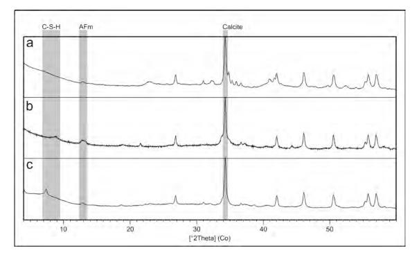
Figure 5. XRPD patterns of the binder fractions of selected hydraulic mortars, with highlighted the main diffraction peaks of the anthropogenic binding phases: a) theatre, cocciopesto mortar at the base of the foundation platform; b) *Thermae Felices Constantinianae*, coating mortar of a pool; c) Republican city walls, foundational concrete.
