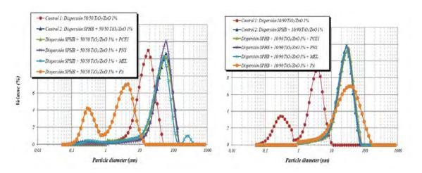
Figure 3. Particle size of the superhydrophobic-photocatalytic dispersions.
