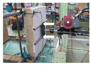
Figure 2. Test arrangement and loading of the adobe wall reinforced with plaster.
