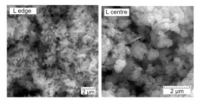
Figure 5. SEM photomicrographs of L paste with 90 days of age taken close to the exposed surface (edge) and in the centre of the specimen.
