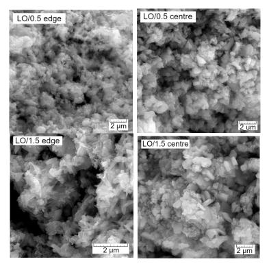
Figure 6. SEM photomicrographs of LO paste with 90 days of age taken close to the exposed surface (edge) and in the centre of the specimen.
