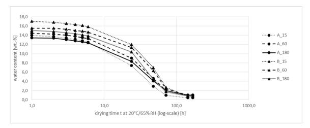
Figure 4. Drying properties (weight loss due to water release) under 20 °C and 65 % RH.
