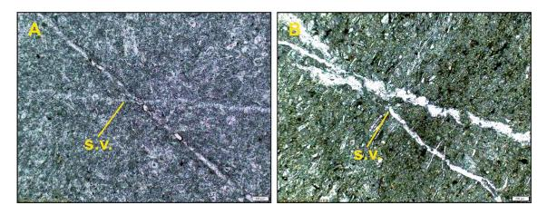
Figure 5. A. Microscopic character of the Zlíchov lm. fragment found in the sample PH 5. B with marked sparitic veins (s.v.). Example of microscopic structure of the Zlíchov lm. from the historic quarry in the Prokop Valley in Prague. Both in PPL.
