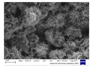
T35552 Date(m/d/y): 06/04/15 Digital Microscopy Imaging Figure 7. NHL5 paste at 28 days shows C-S-H evenly spread and hexagonal aluminosilicate hydrates.
