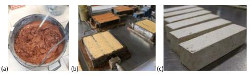
Figure 2. Production of the T\_E mortar (a), prismatic specimens of T\_AP and T+CL in the metallic moulds (b) and prismatic specimens of C mortar (c).
