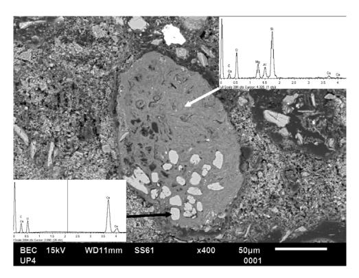
Figure 13: SEM backscattered image of a soil fragment, EDX measurements indicate clay minerals (probably montmorillonite) and calcite (bright spots)
