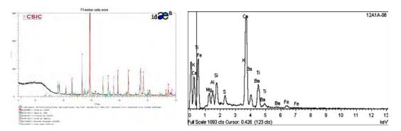
Figures 14a and 14b. X-ray Diffraction and X-ray Spectroscopy of the mass of the ocher lime mortar.
