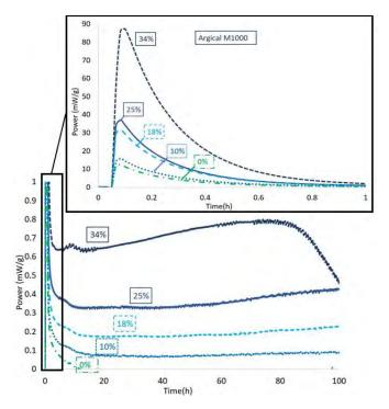
Figure 5: The reaction kinetics of CL90 lime pastes containing 0, 10, 18, 25 and 34% Argical M1000 at 40  $^{\circ}\mathrm{C}$
