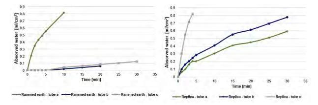
Figure 13 – Water absorption by three Karsten tubes at Bragança Terraces Residence: (a) south exposed rammed earth wall; (b) rammed earth replica
