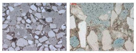
Figure 4. Left: Microphotograph of the aggregate (Kz = quartz sand) in mortar MS (after 28 days curing under outdoor conditions; parallel polarized light). Right: Microphotograph of a detail of mortar MS: in the binder  $C_2S$  and  $C_3S$  can be identified (after 28 days curing under outdoor conditions; parallel polarized light).
