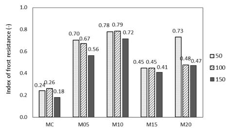
Figure 7. Index of frost resistance (ratio of final and initial flexural strength) of mortars after 50, 100 and 150 freezing cycles.
