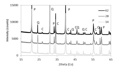
Figure 4. Diffractograms recorded in auxiliary mortars (without limestone flour as filler) containing 1% of flax oil. P = portlandite, Q = quartz, C = calcite.
