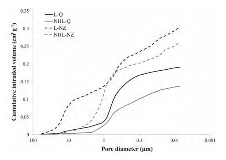
Figure 4. Cumulative pore volume in renders at 28 days.
