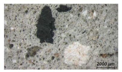
Figure 10: Microscope observation of a coal fragment (black grain on the left) and a gypsum rock fragment (white grain on the right) in the scratch coat of the "Séminaire Saint Rémy", Meaux, 1776
