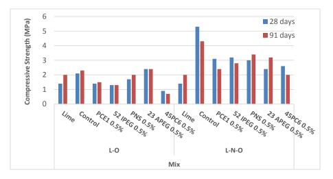
Figure 3. Compressive strength in the Hardened Mortars at different curing times (mixtures with 0.5% of superplasticizer)
