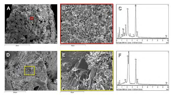
Figure 7. SEM/EDS analysis of sample C03 (fractured surface): (A) general view of the sample; (B) detail of the paste marked in A; (C) EDS spectrum of lime paste in B; (D) zone in the paste with gypsum; (E) close up view showing gypsum; (F) EDS spectrum of gypsum founded in E
