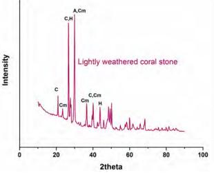
Figure 2. Diffractogram of lightly weathered coral stone sample
