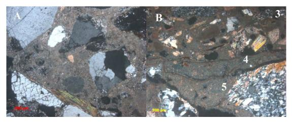
Figure 2: thin section images 5x, XPOL: A) Sample 23288, bedding mortar from the main church with B/A>1, aggregate without carbonates and grain size from medium to coarse. B) Sample 24150-19: layers of plaster: 3-*intonaco* with a well sorted sand of fine grain size; 4- whitewash layer; 5- *arriccio* with unsorted sand of coarse grain size.
