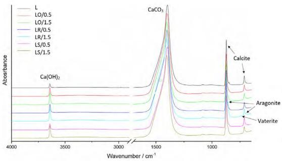
Figure 4. FTIR spectra of the samples with 90 days of age.
