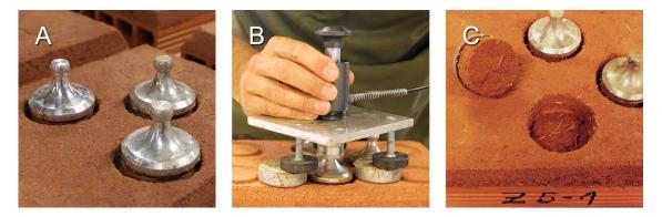
Figure 2. Pull-off test: A - Metallic devices glued to the plaster specimens; B – Pull-off equipment perpendicular to the specimen being tested; C – specimen after cohesive rupture
