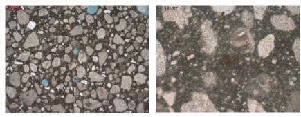
Figure 3. Microphotograph of mortar MT (after 28 days curing in laboratory conditions; parallel polarized light)
