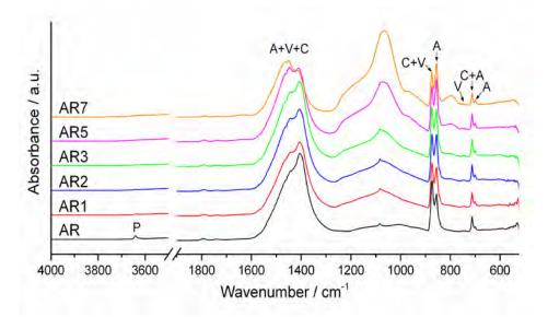
Figure 7. ATR-FTIR spectra of the samples. The peaks of calcite (C), vaterite (V), aragonite (A) and portlandite (P) are indicated.
