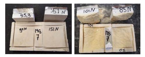
Figure 9. Left: Mortar MS applied on Migné limestone, after pull-off test (mortar tested 1 month after application): fracture at substrate/mortar interface; Right: Mortar MS applied on Maastricht limestone, after pull-off test (mortar tested 1 month from application): fracture in the substrate.
