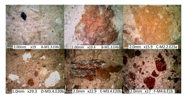
Figure 7. Visual aspects of the mortars. A-M1.3.E4b: yellow *patina* with quartz grains, lime lumps and ash. B-M1.3.E4b: layer of reddish bedding mortar covering the filling mixture. C-M2.2.e23a: coarse crushed brick fragment in a brown mortar matrix. D-M3.4.E20b: medium lime lumps and fine to coarse fired brick clasts, E-M3.4.E20b: shale and crushed brick fragment. F-M4.6.E1b: fine-grained quartz and lime nodules, subangular brick clasts.
