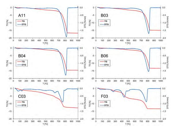
Figure 4. TG-DTG curves of samples A11, B03, B04, B06, C03 and F03
