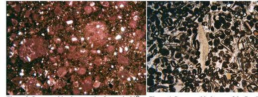
Figure 3. Petrographic photograph of an early 20<sup>th</sup> century repair mortar made with crushed Portland stone and fine quartz sand set a PC binder. 2X natural light. Field of view c. 7 mm.
