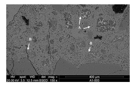
Figure 10. Microphotography by SEM. Identification of unhydrated belite (B) and alite (A) crystals.
