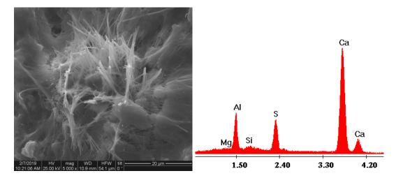
Figure 10. Ettringite crystals observed in NHL-CA specimens after 28 days healing period
