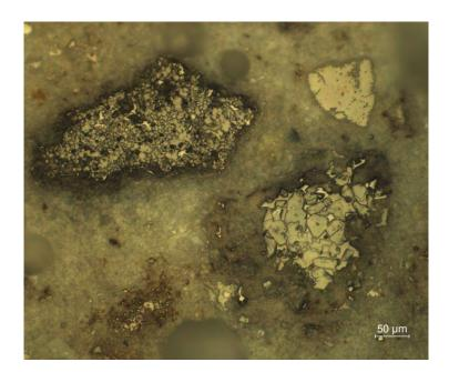
Figure 9. Combination of large crystallized grains filled either with small C2S or large C3S. Optical microscope view (G=X20) of the greyish concrete.
