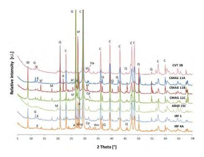
Figure 3. Binder rich fraction diffractograms for samples belonging to awarded buildings from 1903 (CVT3-B) to 1938 (IRF1, IRF4A). Notation: C-Calcite; Q-Quartz; M-Muscovite; G-Gypsum/Calcium carboaluminate; K-Kaolinite; Kf-K-feldspar; Cp – Clinker Portland; p-Plagioclase; Ha-Halite; Hm-Hematite; A – Aragonite
