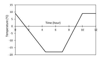
Figure 1. Time/temperature program for a single freeze/thaw cycle.
