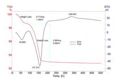
Figure 6. TGA and DTA curves of GC gypsum plaster.
