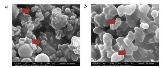
Figure 4. (a) Hexagonal, spherical and angular nanoparticles of Ca(OH)<sub>2</sub> (Exp03); (b) Spherical and angular nanoparticles Ca(OH)<sub>2</sub> and presence of aggregates (Exp04)
