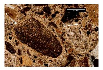
Figure 23. Sample B3. Trasmited light, crossed nicols. Presence of a large number of ceramic fragments (C). Presence of calcite nodels (L).
