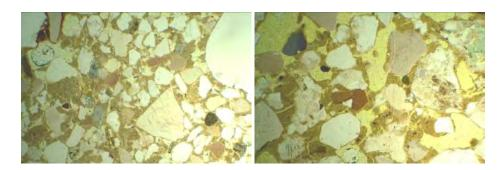
Figure 19. With fluorescent epoxy is used for preparing the thin section samples the air pores and capillary pores is clearly visible as light yellow in the photos. In these two samples the pores are connected with capillary pores, but only the example to the right has a collapsed pore system as the amount of binder is less than what it needs to fill up the sand. The width of each sample is equivalent to 2.65 mm. Illustration: Kristin Balksten.
