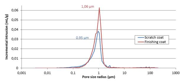
Figure 13: Pore size distribution and threshold radius of scratch and finishing coats from "Hôtel Amelot de Bisseuil", Paris, 1660.
