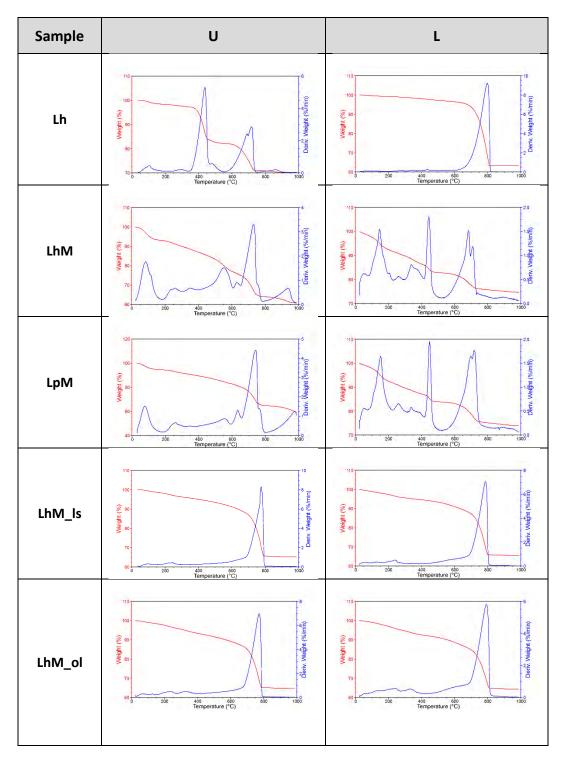
Figure 5. TGA/DTG (red/blue) curves of the binder fraction of samples extracted from upper (U-left) and lower (L-right) parts of the experimental wall.
