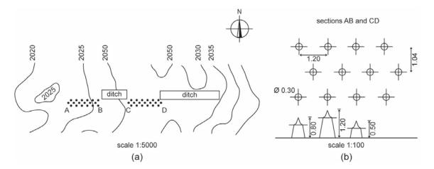
Figure 1: (a) schematic illustration of the anti-tank barriers and anti-tank ditches situated in the high moor at plateau Plamort and (b) detailed sketch of the individual anti-tank barriers. Values are in given in meters (adapted from [15]).
