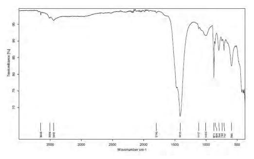
Figure 7: FTIR spectrum of the sample 24972. Peaks of calcite are: 1796, (peak at around 1396 cm<sup>-1</sup> is covered by carbonate double peaks of hydromagnesite), 873,712 cm<sup>-1</sup>. Peaks identifying hydromagnesite are: 3648, 3506, 3443, shoulder at 1473, 1415, 854, 794, 744, 590 cm<sup>-1</sup>.
