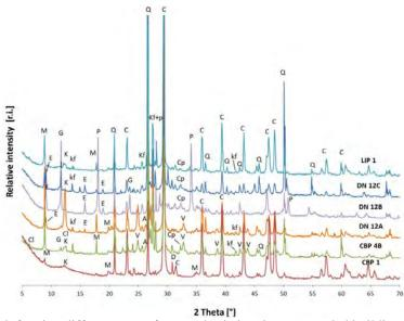
Figure 4. Binder rich fraction diffractograms for samples belonging to awarded buildings from 1939 (CBP1, CBP4B) to 1958 (LIP1). Notation: C-Calcite; Q-Quartz; M-Muscovite; G-Gypsum/Calcium carboaluminate; K-Kaolinite; Kf- K-feldspar; Cp - Clinker Portland; V-Vaterite; E-Ettringite; p-Plagioclase; D-Dolomite; A – Aragonite; P – Portlandite; Cl - Chlorite
