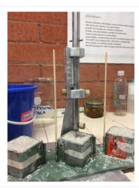
Figure 17 Stiffness range to measure lime mortar period of workability once pozzolans have been added. TECTRAD INAH 2019
