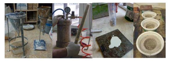
Figure 3. Fresh state properties of the grouts. Marsh cones, column sand test, syringe test, drying shrinkage with mortar cups (from the left to the right)
