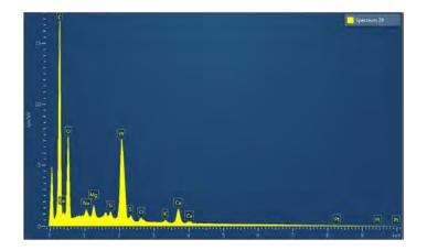
Figure 8. Point EDX measurement of a charcoal fragment in sample SM-28-3.
