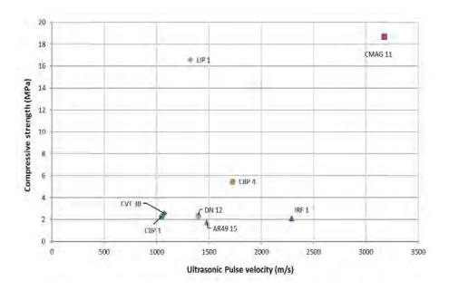
Figure 9. Compressive strength in relation to ultrasonic pulse velocity
