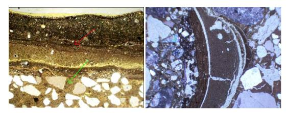
Figure 16. To the left: The sample above is from a French defense plant in Madagascar. The wall is made of bricks that have been plastered and decalcified. The green arrow points out the plaster and the red decolour. 4.8 x 3.1 mm. Illustration: Bo Nitz. To the right: Many layers of lime render, covered with two lime wash layers (each in many applications) and another two layers of lime renders. 4.8 x 3.1 mm. Illustration: Kristin Balksten.
