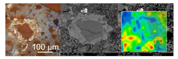
Figure 2. Left and Center: PLM and SEM images of a volcanic aggregate, surrounded by a dense ring of calcium carbonate; Right: FTIR map of the overlapping zones of carbonate and silicate (100%-50% opacity). Scale: Red to Blue: 1.0-0.0. Opus caementicium, Ostia Antica (Italy)
