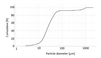
Figure 1. Grain size distribution of the limestone filler.
