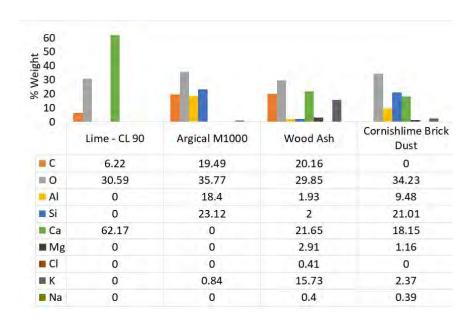
Figure 1: Elemental composition of the raw materials (Weight %)
