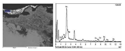
Figure 26a. Spectroscopy of the ocher lime mortar's mass. Figure 26b. Elemental composition of the golden leaf: 92,71 % Gold (Au)/ 3,30 % Silver (Ag)/ 3,39 % Copper (Cu).
