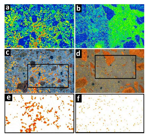
Figure 4: A comparison of two types of experimental mortar, with quantitative volumetric analysis provided by pixel-counting equivalent areas of the highest density of bound water of a FTIR maps overlaying scaled OM images. Scale (both): Red to Blue: 2.5-0.0. Area of black rectangle is 0.5 mm<sup>2</sup>. The pixel density of the left, lime-pozzolana mortar is 3.5 x that of the right, ceramic-lime mortar.
