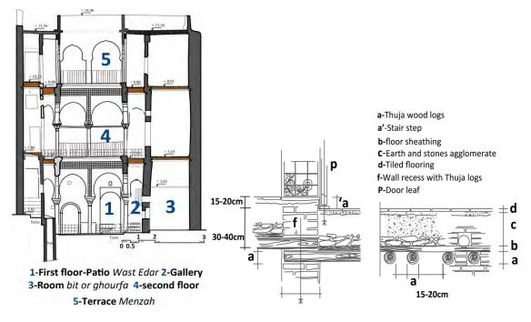
Figure 3. Left: Cross-section of a traditional house (Ali PACHA Agency). Right: Constructive system of ceilings/floors [9].
