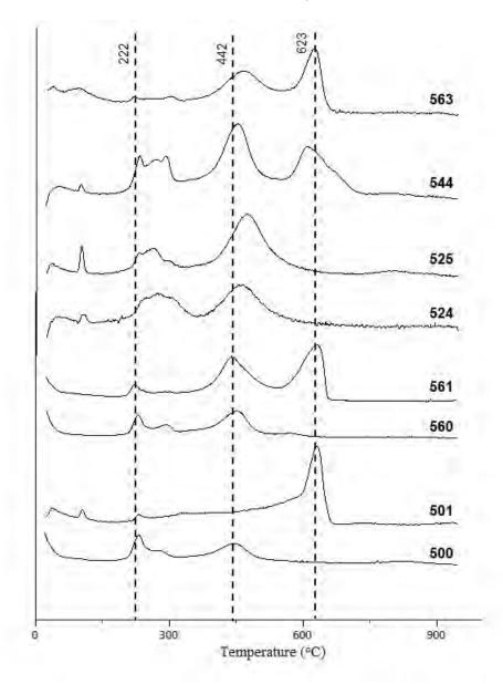
Figure 4. TGA differential curves
