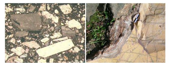
Figure 1 (left) - Single calcite crystals (finish coat of plaster Cividate C., *domus*) Optical microscopy on transverse thin section – XPL
