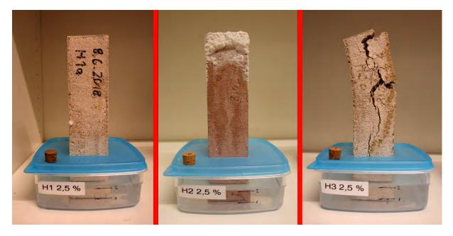
Figure 9. Mortar prisms of hot applied mortars with different mixtures in a 2.5% magnesium salt solution after 60 days
