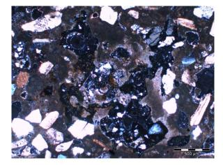
Figure 3c. Delicate network of calc-silica reaction products and altered biogenic grains in well-sorted mortar Type C sample TWO.03. XPL; Scale bar 500µm; photomicrograph M Thacker.
