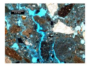
Figure 5. Microphotography with plain light where it can be seen quartz grains, fragments of metamorphic rocks and limestone grains. Also there can be seen retraction cracks and rounded pores.
