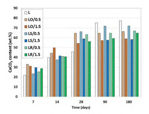
Figure 2. Evolution of the calcium carbonate content in the pastes measured with TG up to 180 days.
