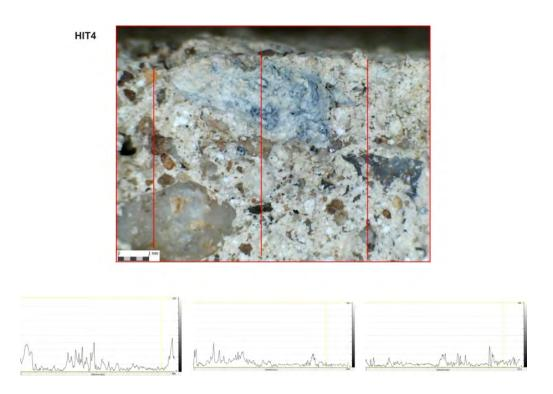
Figure 11. Graph of vector and vertical colorimetry analysis, in which three results are showing from three different vectors. Saturation peaks are produced by the presence of aggregates with high size in relation with the sands (maybe gravels or calcites).
