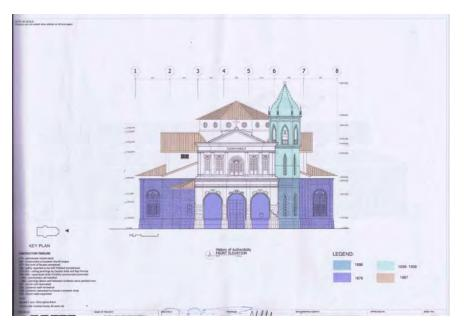
Figure 2. As-built façade of the church showing the construction timeline.
