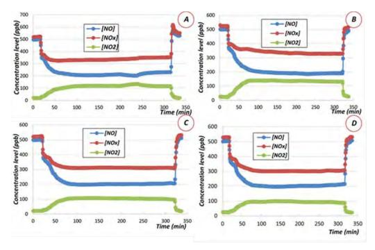
Figure 4. Profiles of NO, NO2 and NOx abatements for ZnO (a),  $TiO_2$  (b) and the heterostructures  $TiO_2/ZnO$  50:50 (c) and 10:90 (d).
