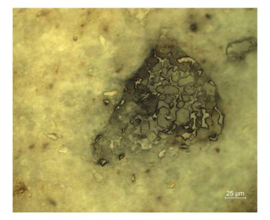
Figure 8. Large well crystallized clinker grain filled with large C3S. Optical microscope view (G=X40) of the greyish concrete.
