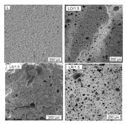
Figure 9. SEM photomicrographs of the pastes with 90 days showing the typical aspect of their texture at low magnification.
