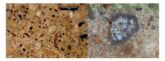
Figure 20. Thin section photomicroscograph trasmited light, crossed nicols. Detail of the lumps of calcined marls. Detail of the unhidrated belite crystals inside of a lump (B).
