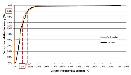
Figure 6: Cumulative relative frequency of analyzed coats as a function of their calcite and dolomite content.
