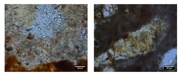
Figure 2. "Cloudy" structures around a pore filled with needles in sample VB1 (left). Polarizing microscope image, parallel polarizers. Diffuse dark areas at the edge of a pore of sample CA4B (right). Polarizing microscope image, parallel polarizers.
