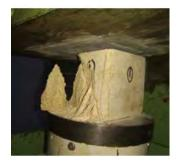
Figure 1. Failure of the coral stone cube under compression
