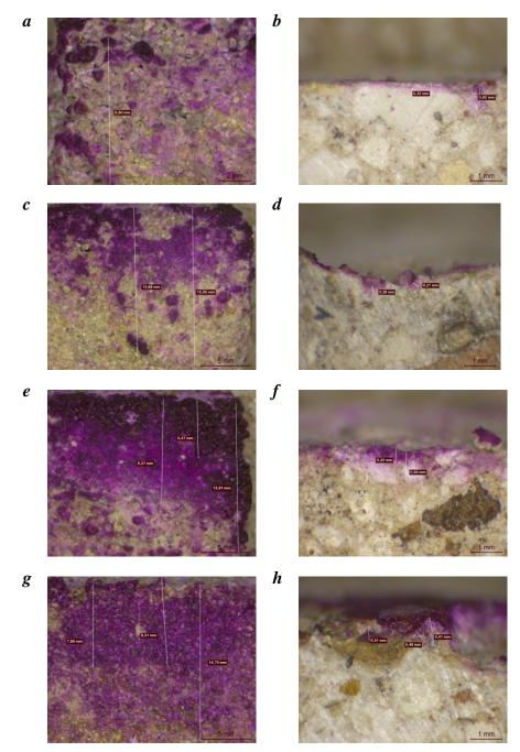
Figure 6. Evaluation of penetration ability on sandstone of a) Exp01, c) Exp02, e) Exp03 and g) Exp04 and on mortar b) Exp01, d) Exp02, f) Exp03 and h) Exp04
