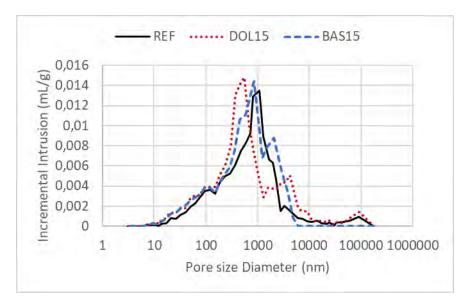
Figure 4: MIP pore size distribution for laboratory composites at 28 days of curing.
