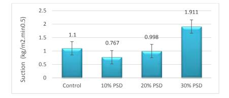
Figure 13. Capillary suction of of NHL5 and NHL5/limestone mortars at 90 days. *COV*=1.14 (control); *COV*=6.40 (10-20%); *COV*=8.19 (30%).
