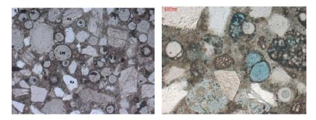
Figure 2. Left: Microphotograph of the aggregate (Ks= marble, Kz = quartz sand, LW = lightweight aggregate) in mortar J (parallel polarized light). Right: Microphotograph of mortar J showing a C<sub>2</sub>S cluster (after 28 days of curing under outdoor conditions; parallel polarized light).
