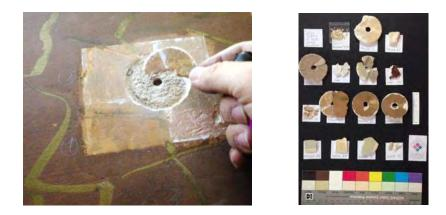
Figure 10. Detail of a sample extracted off the walls' coating in the main room of the Casa Batlló. Figure 11. Collection of the samples extracted in different points of the main floor.
