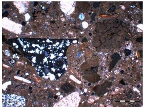
Figure 3a. Subrounded kiln relict maerl fragment close to optical continuity with general mortar matrix in mortar Type A sample TWO.02, with adjacent rounded and isotropic sandstone clast. XPL; Scale bar 1000μm; photomicrograph M Thacker.
