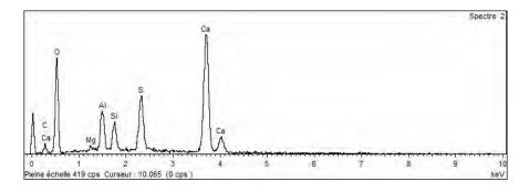
Figure 15. EDS analysis of point 2 identified on Figure 13 confirming the presence of ettringite.
