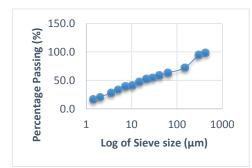
Figure 1. Particle size distribution of the limestone filler.
