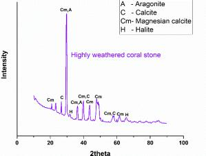
Figure 3. Diffractogram of highly weathered coral stone sample
