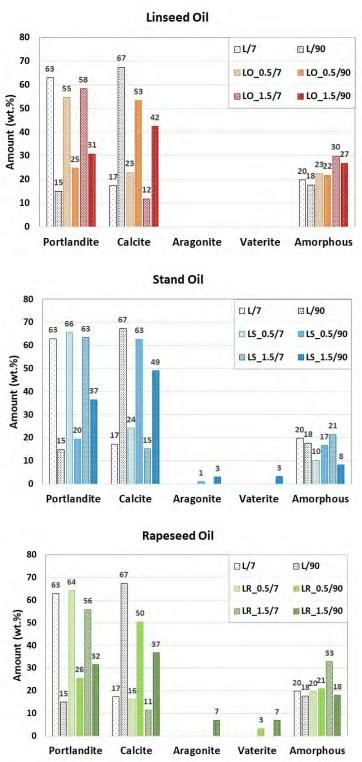
Figure 3. Results of the XRPD-QPA of the samples after 7 and 90 days of curing.
