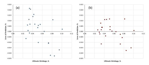
Figure 3. Error of predicted shrinkage using regression Equation 1 (a) and Equation 2 (b) plotted against actual ultimate shrinkage observed
