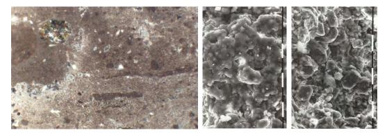
Figure 5. Clay plaster from a wall in Khirokitia. Thin section and photos from SEM
