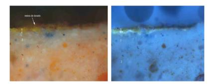
Figure 24a. Cross section= 2: lime mortar and red pigment; 3: Lime mortar of the joint; 4: primer layer; 5: golden leaf. Figure 24b. Idem before with UV light for detecting organic compounds and the nature of the gold.
