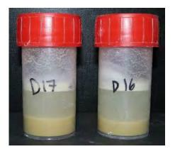
Figure 3: Separation of solid and liquid microgrout components after mixing (Department of Conservation and Built Heritage, University of Malta, 2017).
