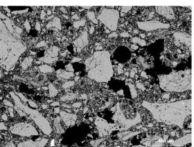
Layer1: finishing mortar M2
