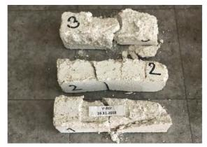
L-Q after 6 cycles of Na<sub>2</sub>SO<sub>4</sub> crystallization
