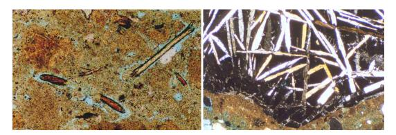
Figure 15. Examples of additives, delibarate and possibly not deliberate. Left, Lime plaster from 'Old Auchentroig', 1702, Buchlyvie, Stirlingshire, Scotland. Lime rich, low content of aggregate, with inclusion of animal hair as a tensile improver in the plaster. Image 2mm width, PPL. Right : Lime mortar, Charlestown, Fif Scotland, 1810, glass-spinaflex slag. Image 5mm width, XPL. Illustration: John Hughes.
