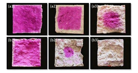
Figure 1: Illustration of the carbonation front over time (days) in prismatic specimens (cross section dimensions 40 x 40 mm) as measured with the phenolphthalein stain method: (a1, b1) REF; (a2, b2) DOL15; (a3, b3) BAS15. Top row: samples at 28 days after casting; bottom row: samples at 90 days after casting. Each individual sample is representative of the average state of all samples tested.
