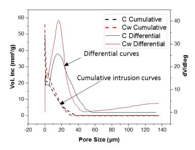
Figure 8. Curves from MIP data for natural coral stone sample in as received condition "C" and accelerated weathered sample "Cw"
