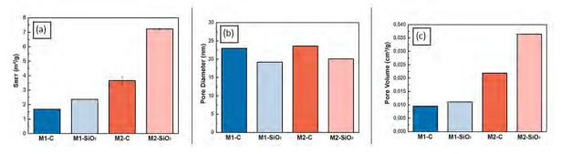
Figure 3. BET results of the mortar samples after 120 days of curing time. (a) surface area; (b) pore diameter; (c) pore volume
