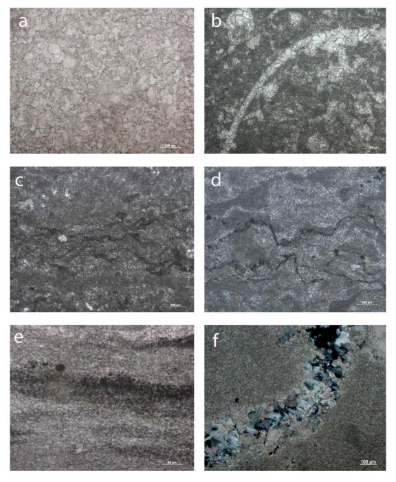
Figure 2. Micrographs of dolomitic rock samples. (a) sample C1; (b) sample C-02; (c) sample D-01; (d) sample E-dol; (e) sample G-01; (f) sample I-01 (all images are under XPOL, except 2a, PPL).
