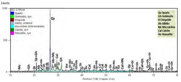
Figure 8. XRD pattern of brick sample M2.2.E8a.
