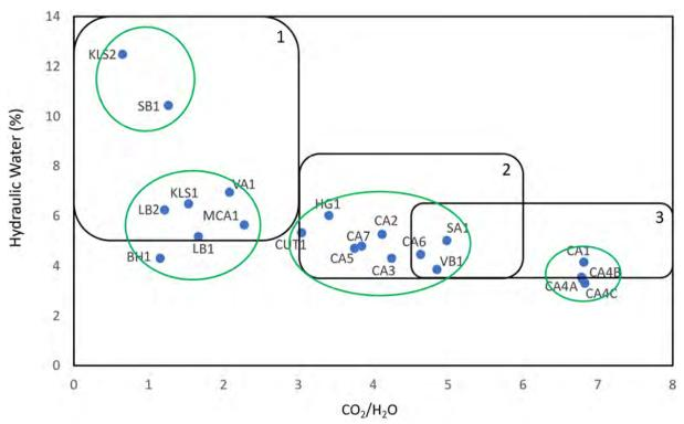
Figure 6. Hydraulic Water (%) against CO<sub>2</sub>/H<sub>2</sub>O ratio. Different categories (1-3) as suggested by Moropoulou et al. (2005) [18]. 1: mortars with natural pozzolana. 2: mortars with artificial pozzolana. 3: hydraulic lime mortars. Framed in green are the four categories into which the examined mortars were classified according to chemical parameters.
