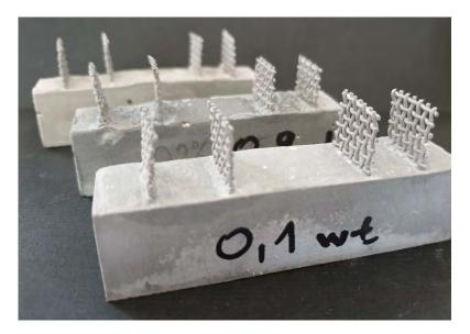
Figure 2. The prismatic specimens of nanomodified mixtures used for measuring the electrical resistance and piezoresistivity at monotonic compression.
