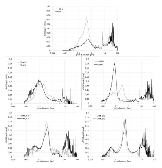
Figure 6. Pore size distribution curves for mortars taken from the upper and lower parts of the wall.
