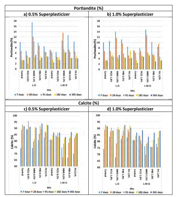
Figure 7. Percentages of Portlandite (Ca (OH)<sub>2</sub>) and Calcite (CaCO<sub>3</sub>) of grouts at different curing times.
