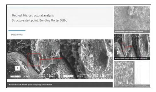
Figure 7. Example of the data regarding the microstructural characterization results of the SJB-J sample
