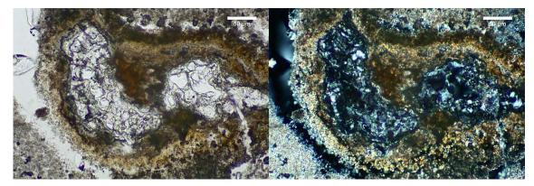
Figure 6: Siliceous, melted phases in a plaster (intonaco) of the Holy Cross Chapel, Scale bar 50µm. Sample 24'978. Left PPOL, right XPOL
