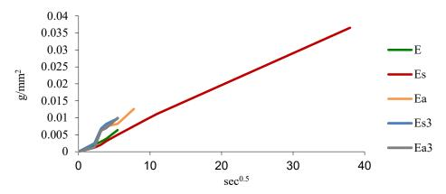
Figure 5. Influence of nano-particles on capillarity of nano-modified calcareous clay at 365 days.
