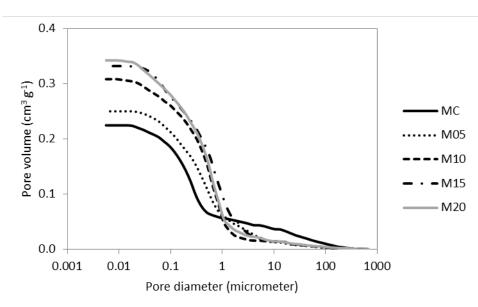
Figure 6. Pore size distribution of flax oil containing mortars.
