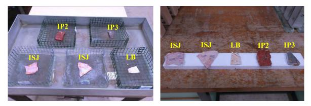
Figure 2. Determination of the capillary water absorption by contact and drying behaviour of the samples
