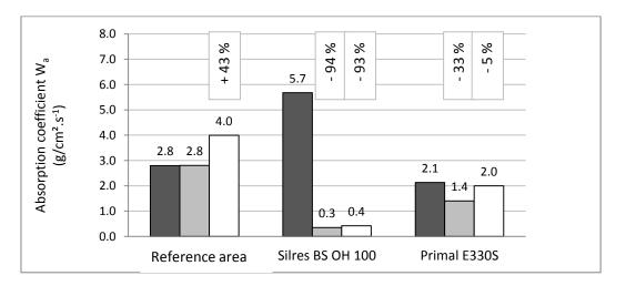
Figure 9. Water absorption coefficient  $W_a$  before consolidation (dark grey), 3 months (light grey) and 9 months after consolidation (white). Top bar chart - relative  $W_a$  change in comparison with  $W_a$  before consolidation.
