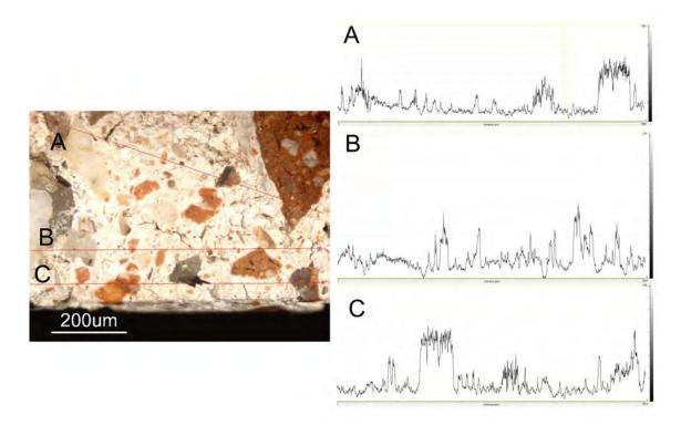
Figure 7. Detail of a linear granulometry from the IV2 sample, where the variation of the colour values shows a granulometric differences between the larger (vectors A and C) and smaller size (vector B) aggregates.
