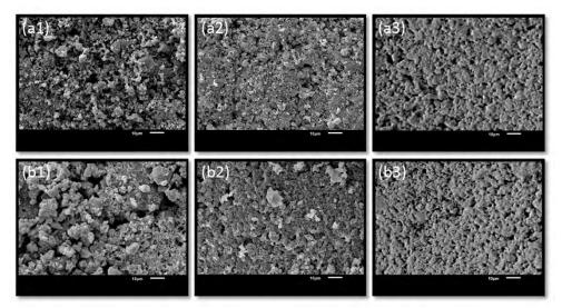
Figure 3: SEM images from the surface of the studied renders, showing their microstructural features: (a1, b1) REF; (a2, b2) DOL15; (a3, b3) BAS15. Top row: samples at 28 days after casting; bottom row: samples at 90 days after casting. Each individual sample is representative of the average state of all samples tested.
