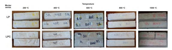
Figure 3. Macroscopic images of series LP and LPC at the elevated temperatures
