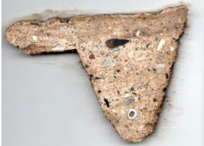
Figure 2a. Thick section mortar Type A x 2. Note: thin mortar 'tails' (with coherent rounded ends which may have abutted underlying constructional clay mortar in the masonry joint) and the more planar face of the former mortar surface. Field of view approx. 120mm; Photograph M. Thacker
