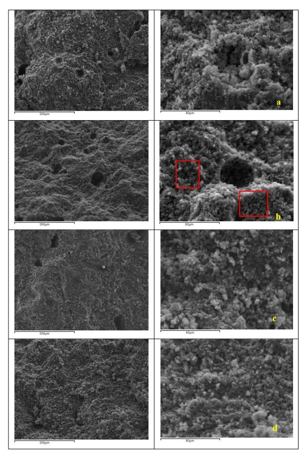
Figure 7. SEM micrographs of nano-modified lime pastes a) LNS3, b) LNA3, c) LNAC d) LNC at 90 days at different magnification
