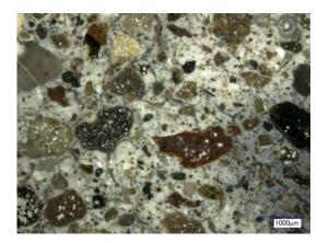
Figure 13. Cross section of the recreated mortar. (Fraunhofer IBP, 2018)
