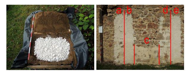
Figure 4. Wooden box covered with a thick plastic foil to prepare a hot mixed mortar in a sandquicklime sandwich technique
