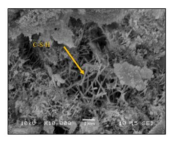
Figure 5. SEM image of the NHL5 limecrete sample showing signs of formed calcium silicate hydrate (C-S-H).
