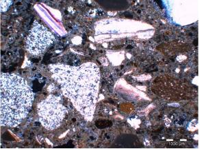
Figure 3d. Poorly-sorted mixture of lustrous marine shell and calc-arenite in mortar Type D sample TWO.09. XPL; Scale bar  $1000\mu m$ ; photomicrograph M Thacker.
