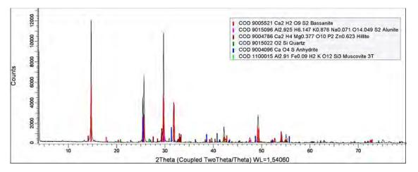
Figure 3. X-ray diffractogram of GB gypsum plaster.
