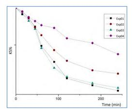
Figure 5. Relative kinetic stability of the four nanolime dispersions
