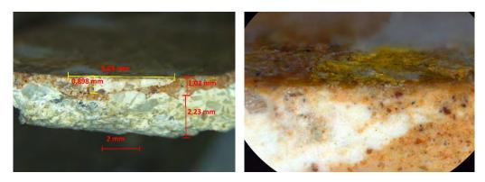
Figures 23a and 23b. Stucco with sgraffito's joint at 10X i 80X: white joint, golden leaf and red lime mortar.
