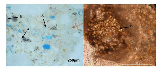
Figure 12. Thin section photomicroscograph. Incident light. Alite crystals (A) and large belite crystals (B).. Trasmited light. Detail of unhidrated belite crystals (B).
