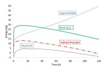
Figure 7: The energy kinetics evolutions of the pastes with different pozzolans 10% at 40  $^{\circ}$ C
