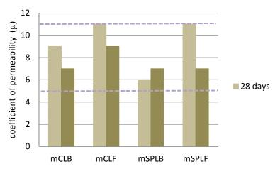
Figure 2. Variation of water vapour inflow and outflow at 28 days
