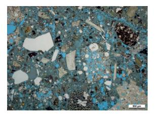
Figure 14. Thin section of the original repair mortar (Fraunhofer IBP/F. Schlütter, 2017)
