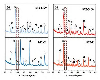
Figure 1. XRD patterns of external surface of mortars, after 120 days of curing. C= Calcite; P=Portlandite; Q= Quartz; H= Hematite; \*= C-S-H phases. The main peak of calcite is marked.
