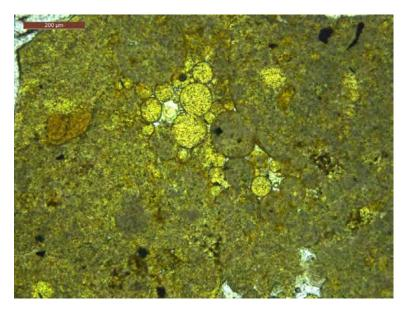
Figure 6. Reacted slag foam in sample PH2. Image taken in plain light.
