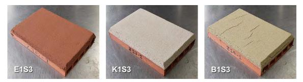
Figure 4. Samples of 20 mm plaster layer applied over hollow bricks: E1S3 - Illitic mortar; K1S3 - Kaolinitic mortar; B1S3 - Montmorillonitic mortar.
