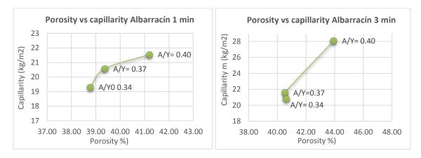
Figure 5. Albarracín gypsum graphics "Porosity vs capillary water transport" in a mixing time 1 and 3 minutes.
