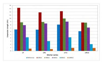
Figure 8. Compressive strength of the mortar compositions at elevated temperatures (90d)
