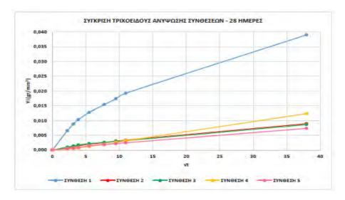
Figure 1 Capillary absorption of the mortar specimens at 28d age 1327
