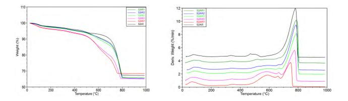
Figure 3. TGA (left) and DTG (right) curves for the studied samples.
