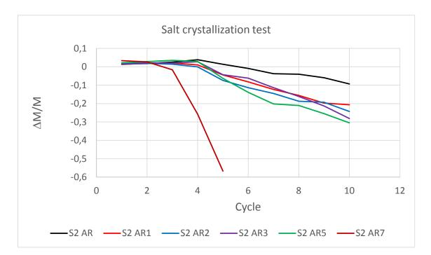
Figure 11. Weight variation of mortar samples during salt crystallization test.
