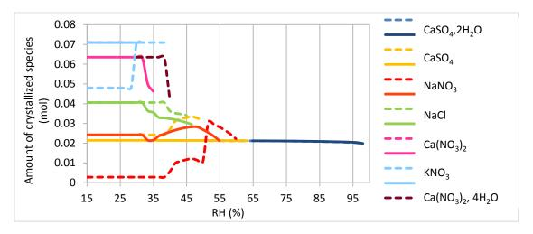
Figure 6: *In silico* simulation of the crystallisation of different salts species in function of RH, at 5°C (dotted line) and 20°C (full line)
