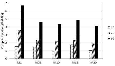
Figure 3. Evolution of compressive strength of mortars in time.
