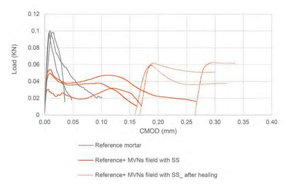
Figure 5. Load – CMOD diagram of samples with MVNs filled with sodium silicate (S) compared to the reference samples (R1).
