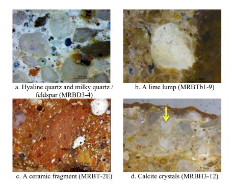
Figure 4. General aspects of the samples observed under the stereo microscope.
