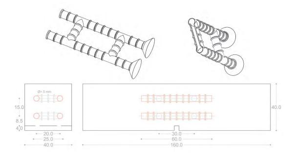
Figure 1. MVNs design and their position in a lime mortar specimen
