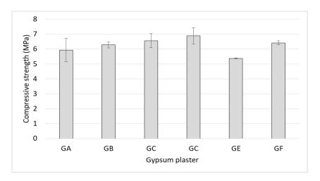
Figure 9. Compressive strength of plasters for w/g ratio of 0.8.
