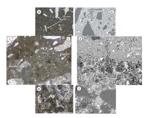
Figure 9: Sample 32. Layer I of sample S32 under optical microscope. Magnification 50x, PPT (a). Layer I of sample S32 under SEM (b). Border between layer I and layer II of sample S32 under optical microscope.
