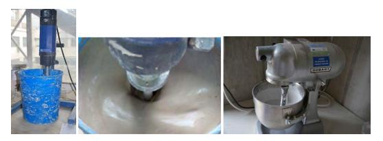
Figure 1. Mixing apparatus of grouts. High-speed mixer (left), Hobart mixer (right).
