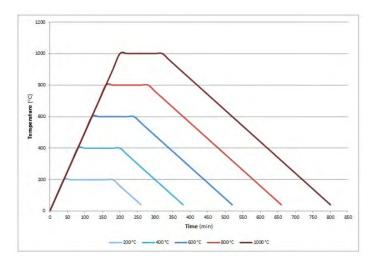
Figure 2. Heating scheme of the mortar specimens (rate, exposure time, cooling rate)
