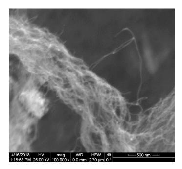
Figure 1. SEM photomicrograph of the CNTs in the solid state, prior to incorporation in the ternary mixtures.
