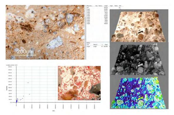
Figure 6. Characterization phases of the Idanha-a-Velha mortars. On the left, absolute granulometries obtained with Digimizer and JMicrovision. On the right side, 3D surface scanning with thermal and gray with ImageJ.
