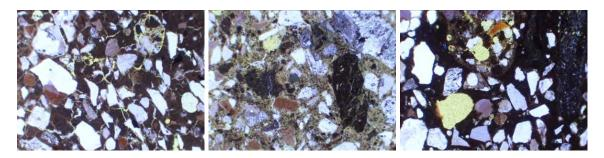
Figure 1. Three mortars made from the same sand and mixing ratio; 1:1 by volume. Wet slaked lime from different Silurian (1) and Ordovician (2-3) lime stone from 1) Hall Gotland, 2) Marieby Jämtland and 3)
