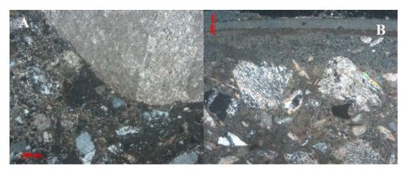
Figure 3: thin section images 5x, XPOL. A) Sample 12781, bedding mortar from the convent. An unsorted sand with carbonate phases is visible. B) Sample 315, the plaster consists of a single layer of *arriccio* covered by a whitewash layer.
