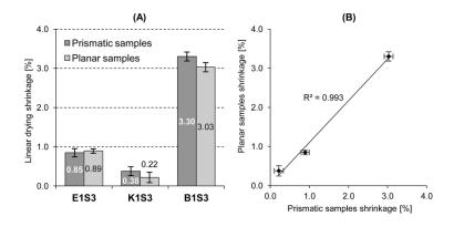
Figure 3. (A) Linear drying shrinkage assessed in prismatic and planar samples; (B) Prismatic samples shrinkage vs. planar samples shrinkage.
