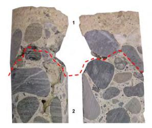
Figure 9. Finishing layer (1) and core (2), sample M3
