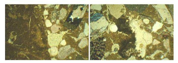
Figure 5. 19<sup>th</sup> century lime render from Visby showing the characteristic lime putty made from the fat Silurian lime of Gotland. In the putty there is often un-mixed lime lump (to the left), air voids and micro cracks (both pale yellow). Width of the image covers 2.65 mm. Illustration Kristin Balksten [14].
