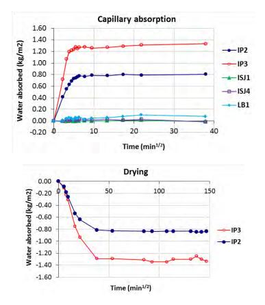
Figure 6. Capillary water absorption and drying curves
