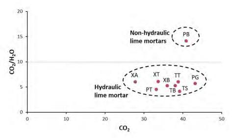
Figure 8. Hydraulic classification of mortars by CO<sub>2</sub>/H<sub>2</sub>O
