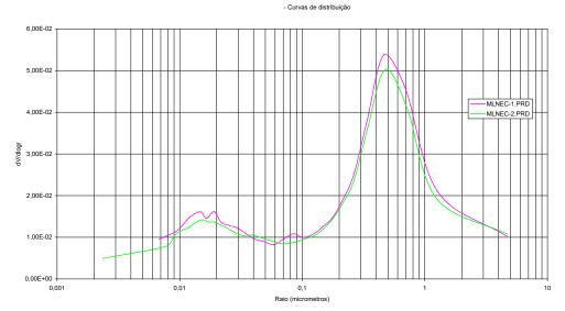
Figure 7. Pore size distribution of the marmorite of LNEC's façade [4]
