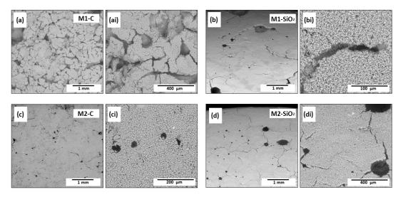
Figure 2. ESEM images of the four types of mortars, after 120 days of curing time. (a and ai): M1-C; (b and b1): M1-SiO<sub>2</sub>; (c and ci): M2-C; (d and di) M2-SiO<sub>2</sub>. To note the different presence of fissures in the mortars, depending on their composition.
