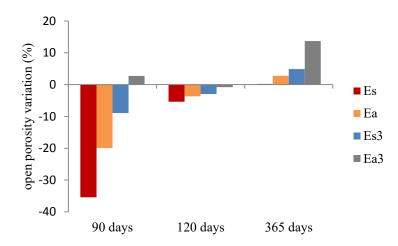
Figure 3. Open porosity variation (%) of nano-modified calcareous clay systems, with respect to the reference.
