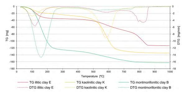
Figure 1. Thermogravimetric curves (TG) and Derivative thermogravimetric curve (DTG)
