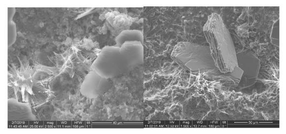
Figure 8. Portlandite crystals and needle-like CSH phases observed after 28 days healing period. NHL (left) and NHL-CA (right)
