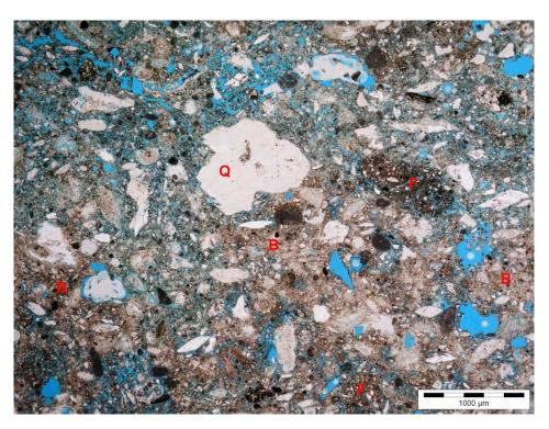
Figure 8: Thin section of plaster B under plane-polarized light, the overall binder is gypsum, brownish areas (B) contain calcite, further aggregates are quartz (Q) and soil fragments (F) besides feldspar and mica
