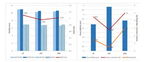
Figure 4. Fresh state properties of the grouts. Fluidity compared to W/B ratio (left), penetrability compared to volume change (right)
