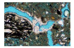
Figure 4. 16<sup>th</sup> Century lime mortar from Gylen Castle, Island of Kerrera, Inner Hebrides, Scotland. Example of secondary calcite crystallisation in pores. Image width 2mm. Illustration: John Hughes.
