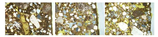
Figure 20. Mixing ratio 1:1, 1:2 and 1:3 by volume made from the same wet slaked lime putty and sand. All samples were worked on in the correct semi-dry consistency working all micro cracks together. On the surface there is lime wash. The 1:3-mortar has an open irregular pore structure and it is not compact enough to be frost resistant. The width of the sample show 4.5 mm. Illustration: Kristin Balksten [18, 19].
