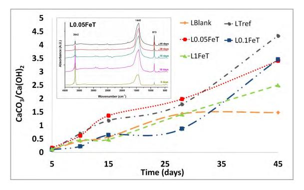
Figure 6. Evolution of the carbonation process of the pastes; in inset the FTIR spectra of L0.05FeT as a function of the curing time.
