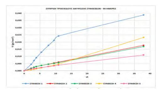
Figure 2 Capillary absorption of the mortar specimens at 90d age
