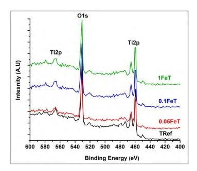
Figure 3. Wide-survey XPS spectra (a) and high resolution XPS spectra of Ti 2p (b), O 1s (c) and Fe 2p (d, e, f) of the TRef and Fe-doped nanoparticles.
