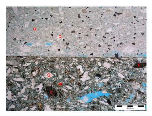
Figure 11: Thin section of relief plaster C (below) and the whitewash above under plane-polarized light, in both the binder is gypsum, aggregates are quartz (Q), soil fragments (F) and micas (M)
