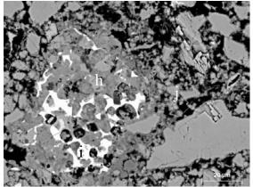
Layer 2: bonding mortar M1
