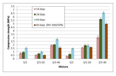
Figure 4. Development of compressive strength of samples through time
