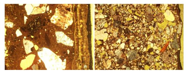
Figure 11. Difference in mineralogy, sand curve and hence, mixing ratio is illustrated by samples from Älvros church by a mortar from 1740 and a mortar from 2000. Here the difference in thickness of historic and modern lime wash can also be compared. The width of each sample is equivalent to 4.5 mm. Illustration: Kristin Balksten.
