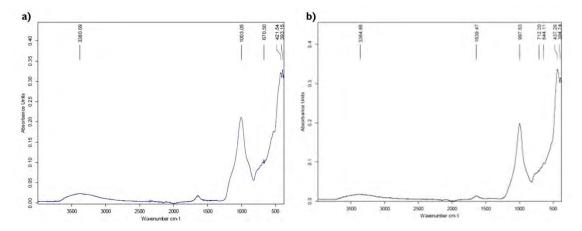
Figure 5. FTIR spectra of Labraunda mortars from a) Natatio b) the Andron building
