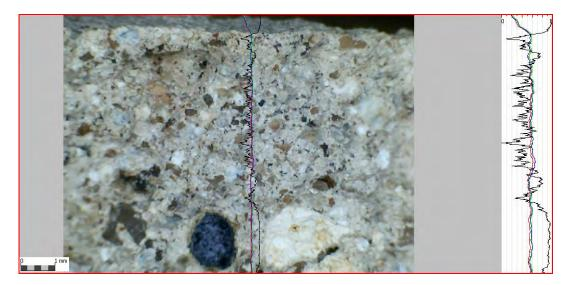
Figure 10. Colorimetry graphic of sample HIT4 shows saturation and hue, while lime-nodules and quartzes change the results of graphic (high-low peaks).
