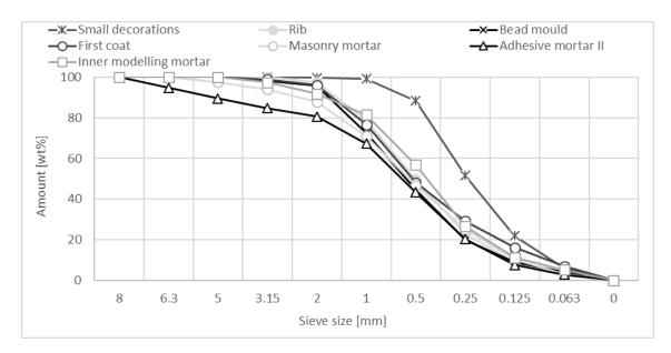
Figure 8. Particle size distribution of insoluble residue – examples of typical curves of the relevant sample groups.
