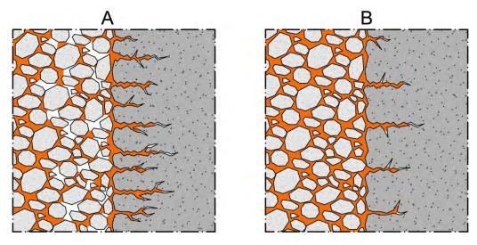
Figure 1. Schematic representation of a mortar applied to a more (A) or less porous (B) support
