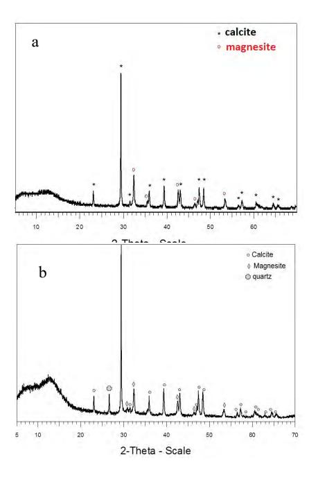
Figure 3. XRD spectra of (a) a hard lump and (b) a soft lump.
