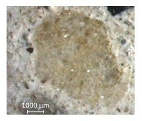
Figure 9: Microscope observation of a gypsum rock fragment (saccharoid gypsum) in the scratch coat of the "Hôtel Amelot de Bisseuil", Paris, France (1660).
