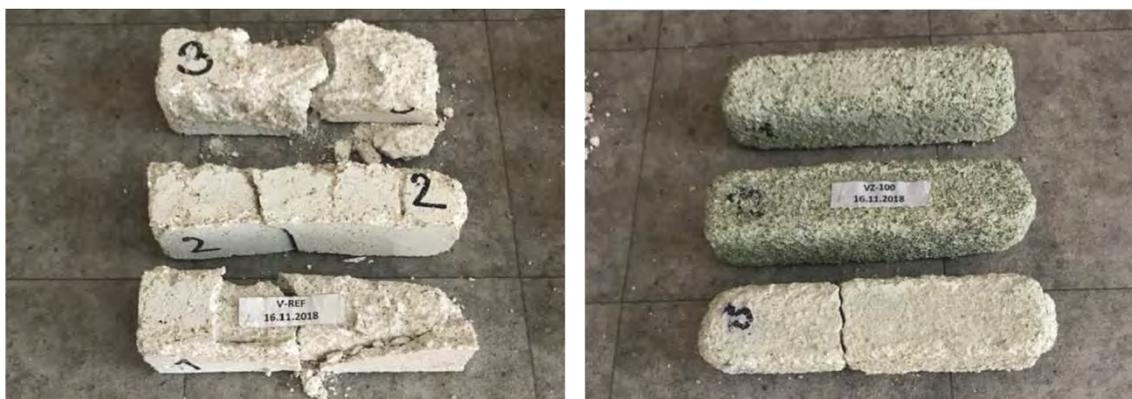
L-Q after 6 cycles of Na<sub>2</sub>SO<sub>4</sub> crystallization
