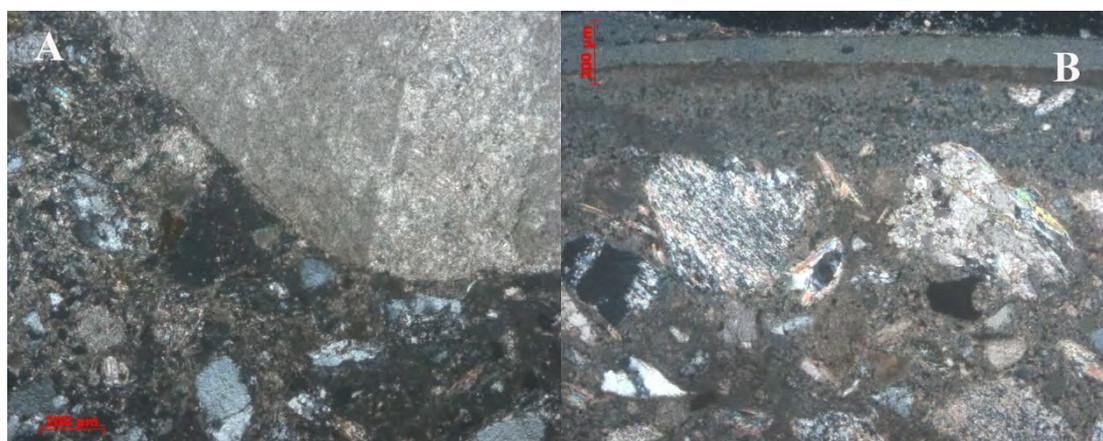
Figure 3: thin section images 5x, XPOL. A) Sample 12781, bedding mortar from the convent. An unsorted sand with carbonate phases is visible. B) Sample 315, the plaster consists of a single layer of *arriccio* covered by a whitewash layer.
