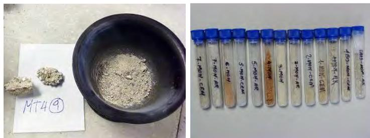
Figure 7. Finely grinded mortar samples for analysis by XRD.
