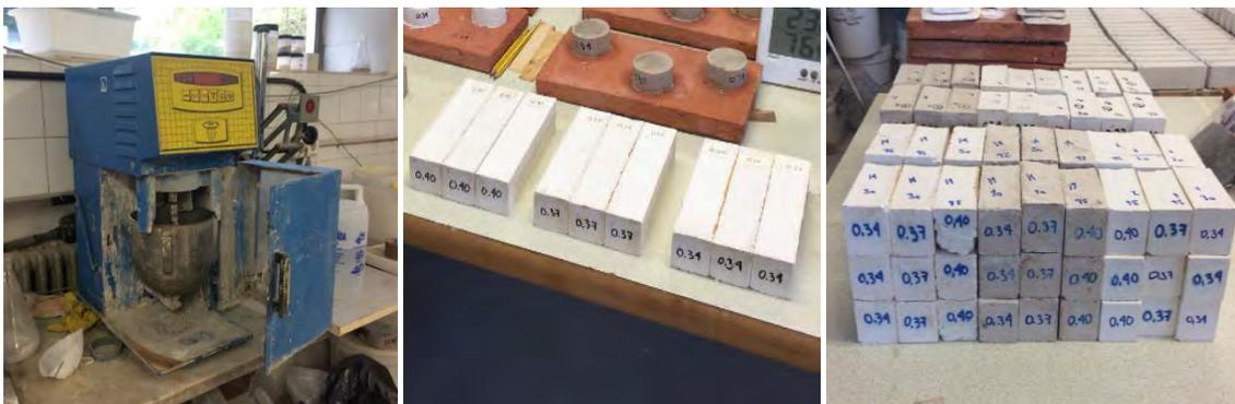
Figure 3. Preparation of test pieces for the mechanical tests according to the Standard Norm UNE-EN 13279-2.
