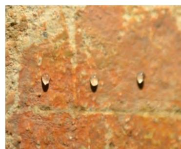
Figure 8. Water drop deposited nine months after consolidation for the test area consolidated with Silres BS OH 100
