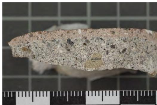
Figure 2. Cross-section of No. 2002, composed of a preparatory and a top layer. (Fraunhofer IBP, 2017)
