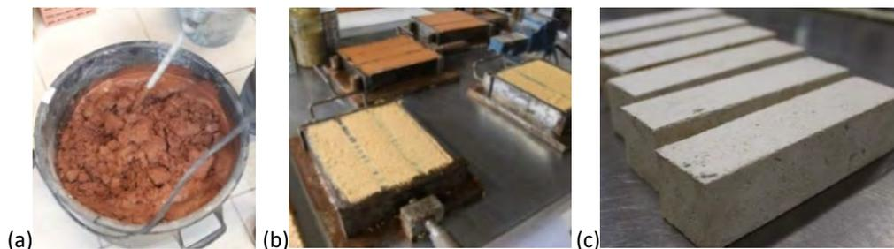
Figure 2. Production of the T\_E mortar (a), prismatic specimens of T\_AP and T+CL in the metallic moulds (b) and prismatic specimens of C mortar (c).
