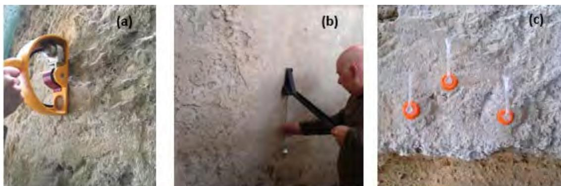
Figure 9 – *In situ* tests: (a) Pendular sclerometer in Bragança Terraces Residence wall section facing south; (b) Sphere impact test at a wall facing East inside Jogo da Pela Tower and (c) Karsten tubes test at a wall section facing East at Bragança Terraces Residence
