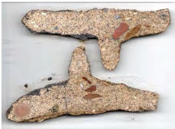
Figure 2a. Thick section mortar Type A x 2. Note: thin mortar ‘tails’ (with coherent rounded ends which may have abutted underlying constructional clay mortar in the masonry joint) and the more planar face of the former mortar surface. Field of view approx. 120mm; Photograph M. Thacker
