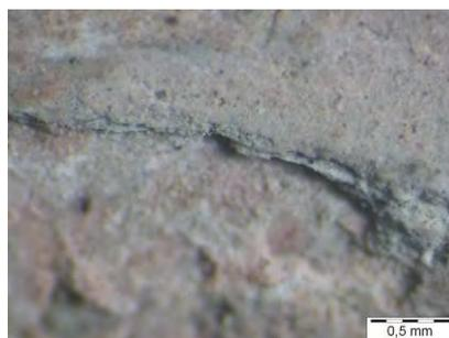
Figure 5. Sample IP3: image showing the difference between the texture of the plaster in the bulk and closer to/at the surface
