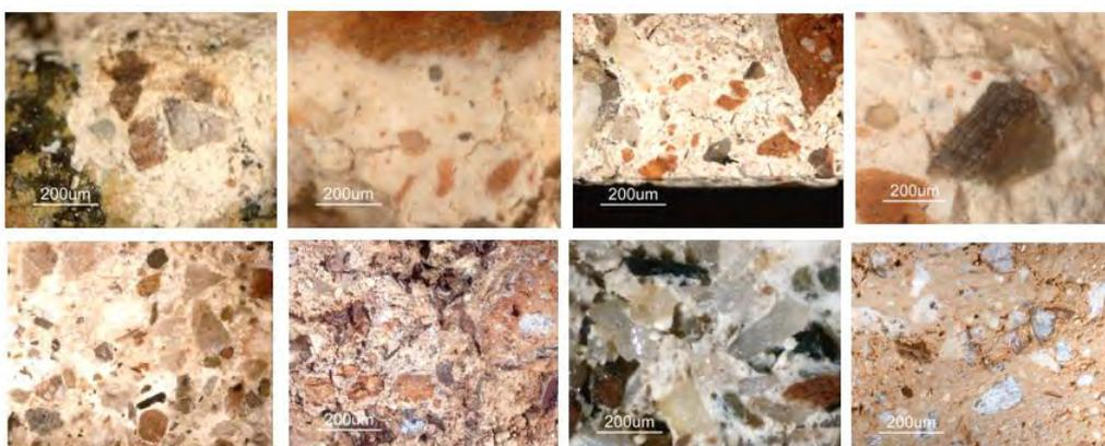
Figure 5. From left to right, and from top to bottom, microphotographs of the analyzed samples of *Sé-Cathedral*, where the difference between the mortars and the plasters is well appreciated.
