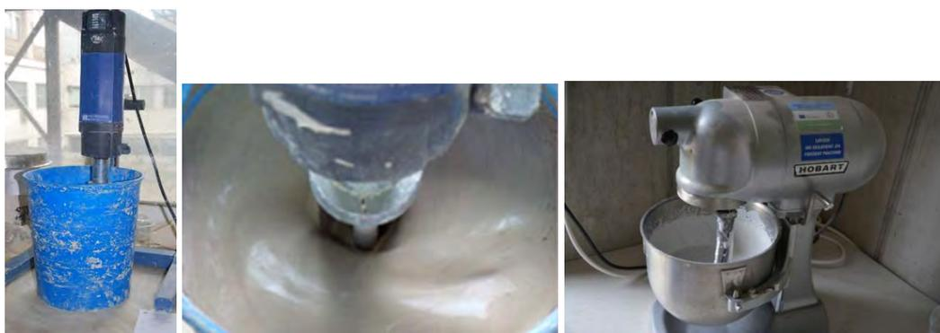
Figure 1. Mixing apparatus of grouts. High-speed mixer (left), Hobart mixer (right).
