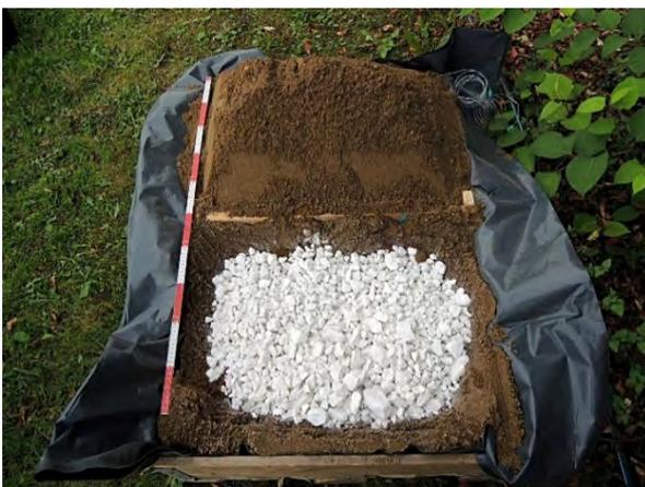
Figure 4. Wooden box covered with a thick plastic foil to prepare a hot mixed mortar in a sand-quicklime sandwich technique
