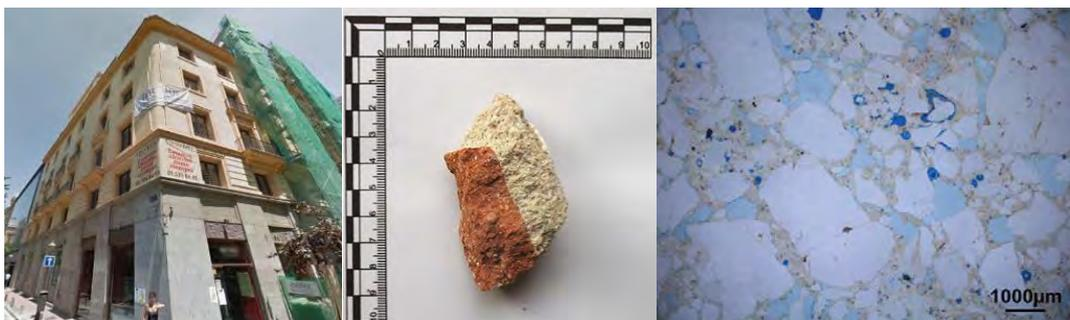
Figure 8. Facade of the building. Thin section photomicrograph. Incident light. Absence of lumps of calcined marls.
