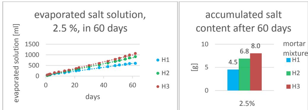
Figure 10a+b: diagram with evaporated salt solution after 60 days and table with the accumulated salt content
