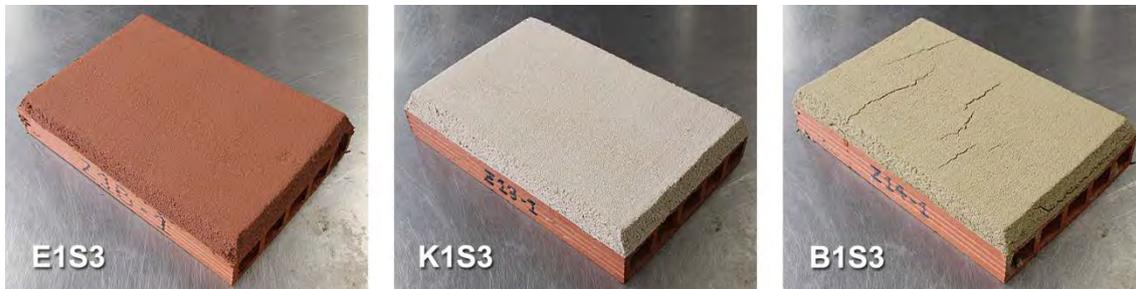
Figure 4. Samples of 20 mm plaster layer applied over hollow bricks: E1S3 - Illitic mortar; K1S3 - Kaolinitic mortar; B1S3 - Montmorillonitic mortar.
