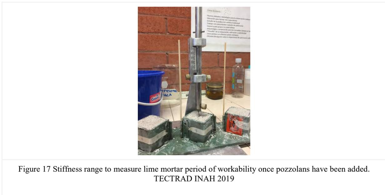
Figure 17 Stiffness range to measure lime mortar period of workability once pozzolans have been added. TECTRAD INAH 2019
