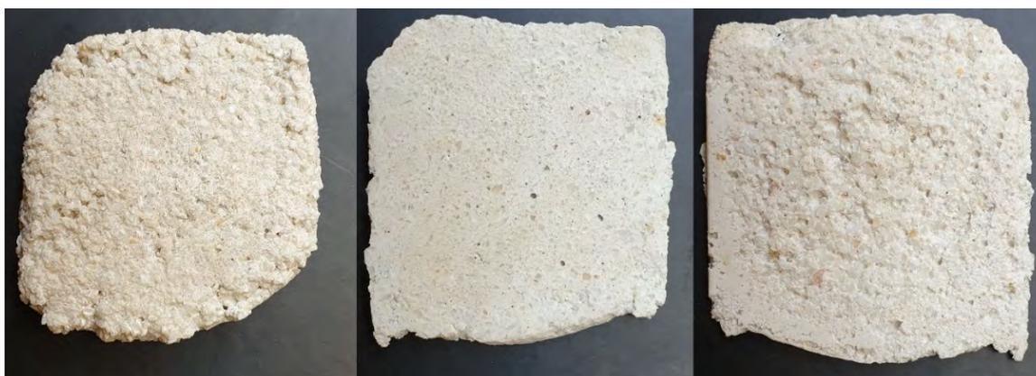
Figure 3. Three views of a mortar composed of marble passed through a 3 mm sieve (not intended to match Carrara marble). Left - the surface as applied off the spatula with rudimentary levelling. Centre – the same batch with all but the upper left corner polished. Right – the underside of one sample showing the coarse texture. It is noted that Carrara marble has grains in the range 300-500 microns, not those used here. No quartz flour was added to these mortars.
