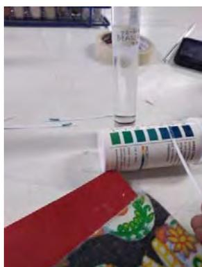
Figure 4. Pozzolan in limewater. Day 1 pH measure 12/13. TECTRAD/ INAH 2019
