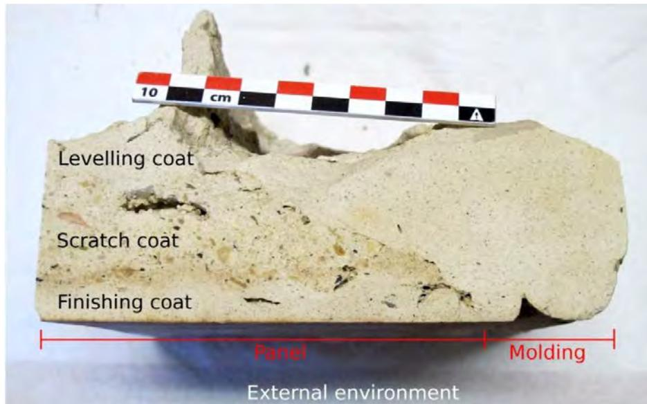
Figure 2: Cross section with different coat types. Render sampled from the building “Hôtel Amelot de Bisseuil”, Paris, France (1660).
