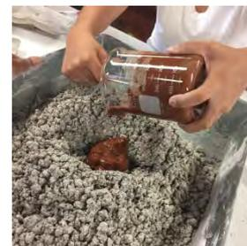
Figure 12 Dosage of pozzolanic additions into mortar. TECTRAD INAH 2019
