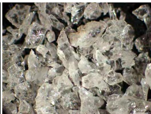
Figure 6 (right) - Quartz clasts obtained through the crushing of a quartz pebble
