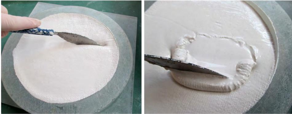
Figure 2. Checking the thickness of compact layer.
