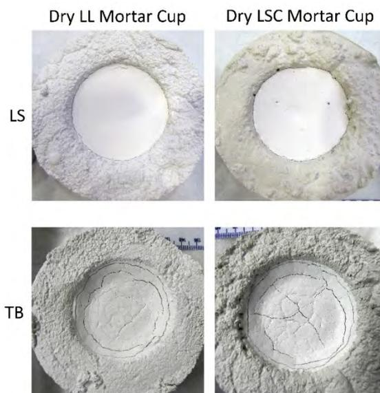
Figure 4. Reference mixtures LS and TB after drying in lime (LL) and lime-cement (LSC) mortar cups.
