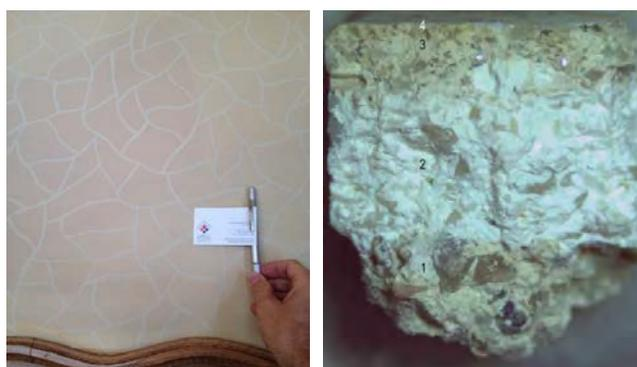
Figures 13a and 13b. Wall presently painted, and coloured lime stucco section.
