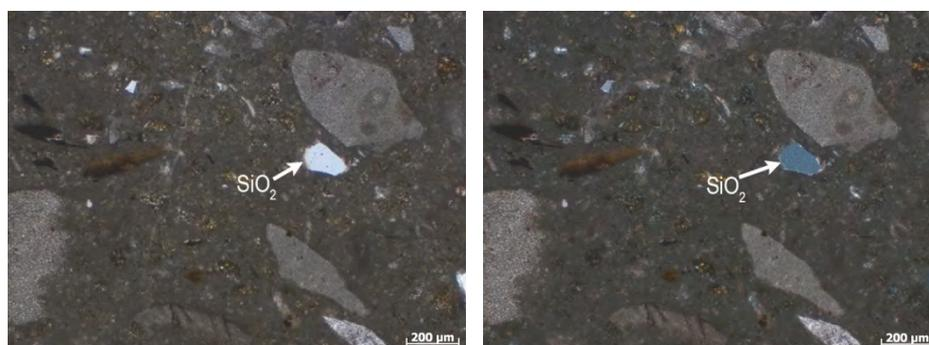
Figure 8: Sample S33 under optical microscope. Magnification 50x, PPT (left). Magnification 50x, XPT (right).
