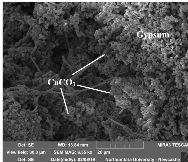
Figure 9. SEM image of the binder in sample SM-28-2.
