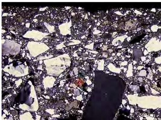
Figure 3 (left) - Single quartz crystals (finish coat of plaster - Milan, p.zza Fontana) -Optical microscopy on transverse thin section - XPL
