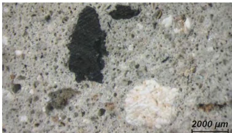
Figure 10: Microscope observation of a coal fragment (black grain on the left) and a gypsum rock fragment (white grain on the right) in the scratch coat of the "Séminaire Saint Rémy", Meaux, 1776
