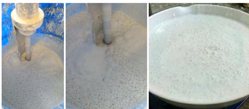
Figure 3. Extreme foaming of ready-mixed grouts (Ledan TB1) in the high speed mixer (left and middle image) and after Hobart mixing of standard grout quantity (image on the right).
