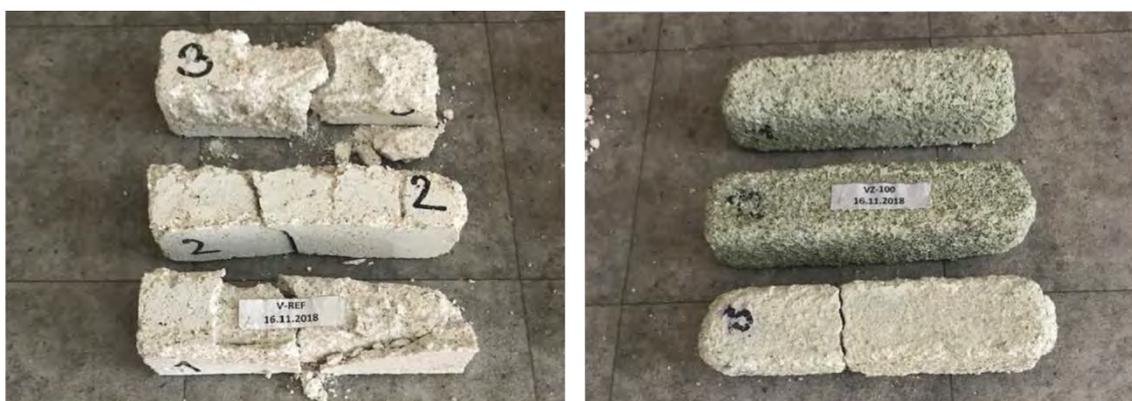
L-Q after 6 cycles of Na<sub>2</sub>SO<sub>4</sub> crystallization
