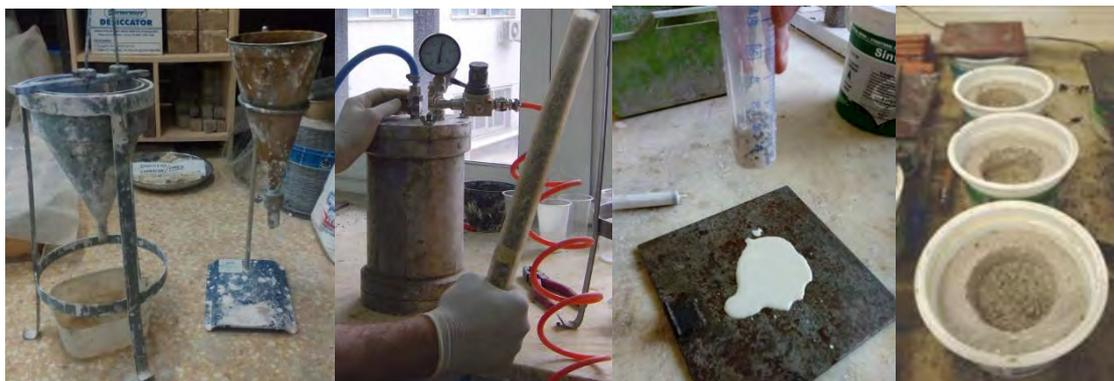
Figure 3. Fresh state properties of the grouts. Marsh cones, column sand test, syringe test, drying shrinkage with mortar cups (from the left to the right)
