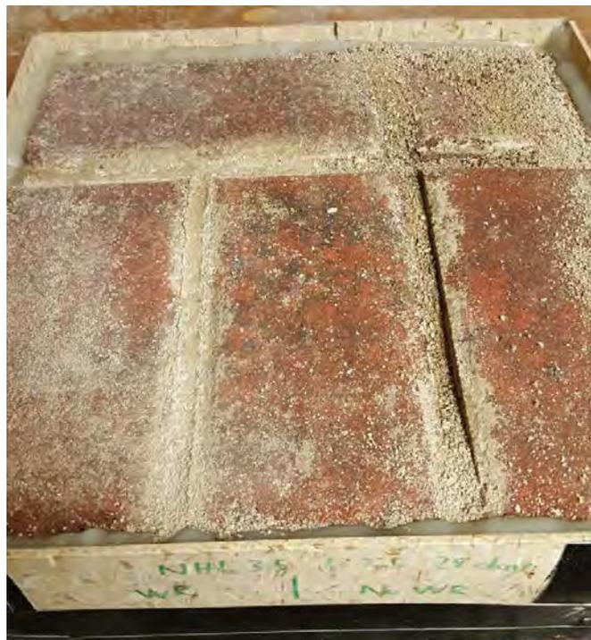
Figure 6. NHL 3.5 mortar with and without silane cream water repellent, after testing of 50 freeze-thaw cycles. The left side is treated with silane cream, the right side is untreated, 2017. Photograph by Chad Lausberg
