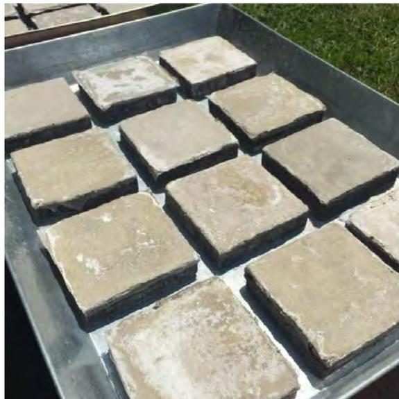
Figure 21. Salts crystallization resistance. Carmona TECTRAD INAH 2018
