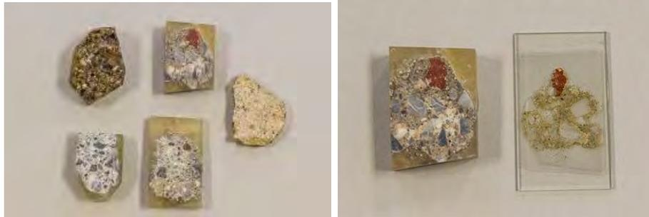
Figure 8. Polished binder samples up to thin section.
