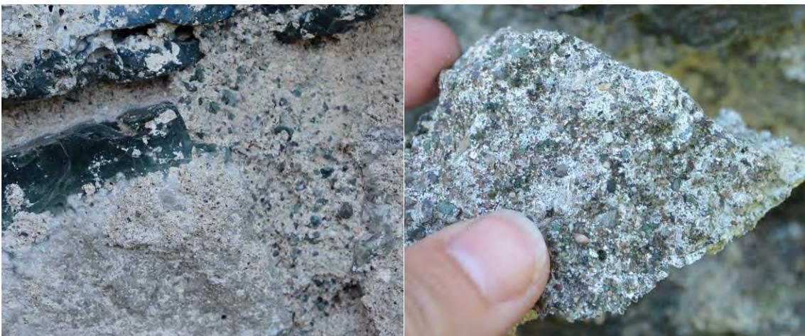
Figure 3 left. Cast slag blocks and slag mortar where the slag particles are rather big. Figure 3 right. A slag mortar with both sand and slag granulates.
