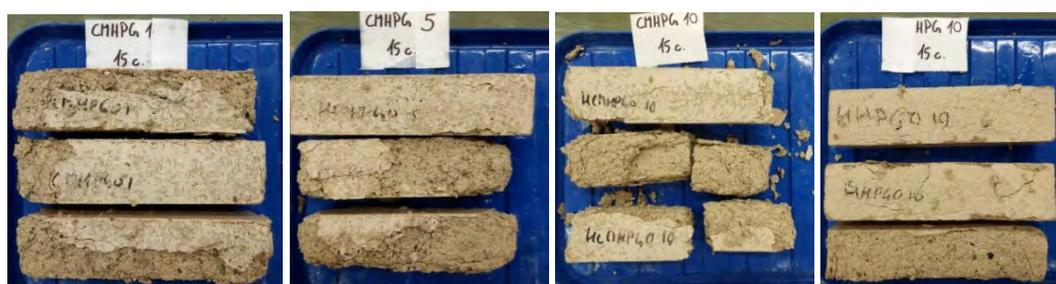
Figure 7. Highly altered samples after 15 freezing-thawing cycles (numbers represent admixture dosage in %).
