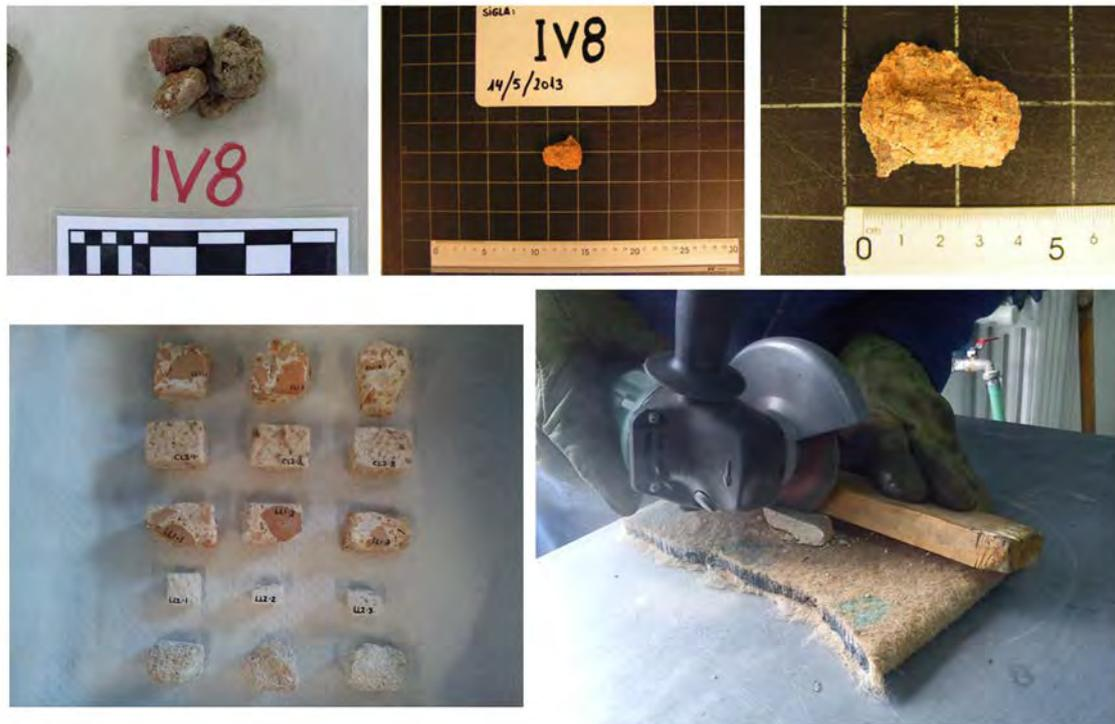
Figure 3. Sequence of preparing the IV8 sample.
