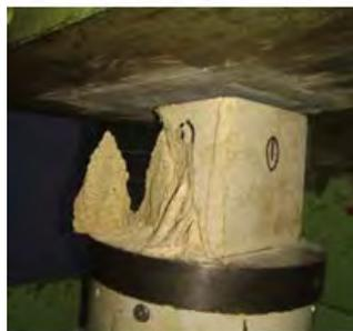
Figure 1. Failure of the coral stone cube under compression
