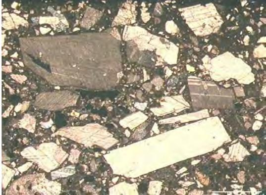
Figure 1 (left) - Single calcite crystals (finish coat of plaster Cividate C., *domus*)
