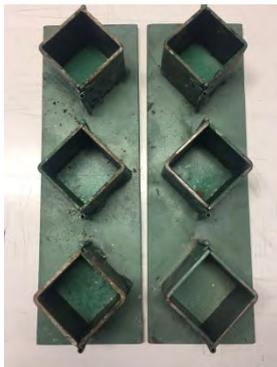
Figure 13 Metal molds for mortars in accordance with ASTM C 1707. TECTRAD INAH 2019
