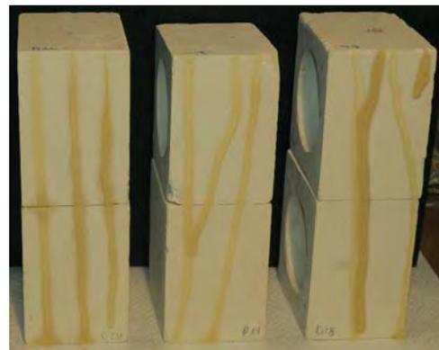
Figure 4: Flow testing (Department of Conservation and Built Heritage, University of Malta, 2017).
