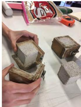
Figure 14 Plywood molds for mortars. TECTRAD INAH 2019
