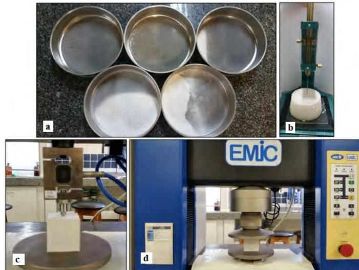
Figure 1. Gypsum plaster tests: a. Grain size tests: sequence of sieves and retained material; b. setting time using the Vicat apparatus; c. Hardness; d. compressive strength.
