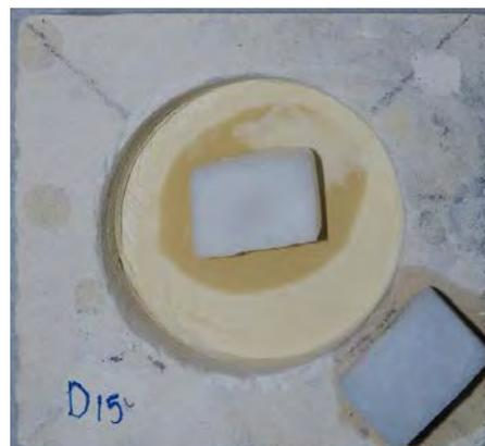
Figure 6: Comparison of DiOx microgrout and Globigerina liquid water absorption. The DiOx sample was applied and set in a Globigerina cup (Department of Conservation and Built Heritage, University of Malta, 2017).
