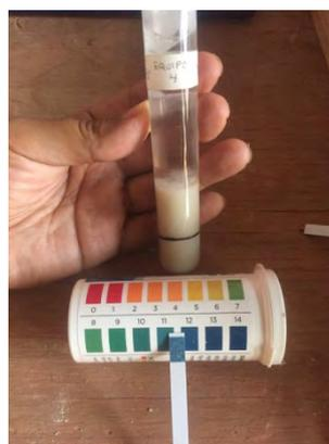
Figure 5. Pozzolan in limewater. Day 7 pH measure 11/12. TECTRAD/ INAH 2019
