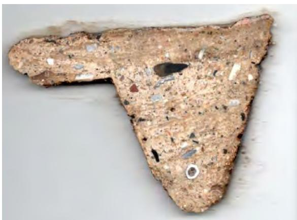
Figure 2b. Thick section mortar Type B. Note very wide mortar tail suggesting much coarser underlying rubble wall; planar face of previous coating surface; high concentration of discoloured bioclasts including probable *maerl* and shell in this particular section. Field of view approx. 100mm; Photograph M. Thacker
