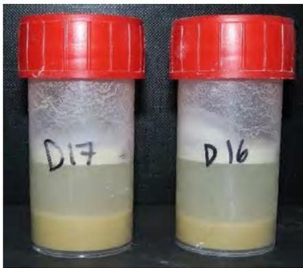
Figure 3: Separation of solid and liquid microgrout components after mixing (Department of Conservation and Built Heritage, University of Malta, 2017).
