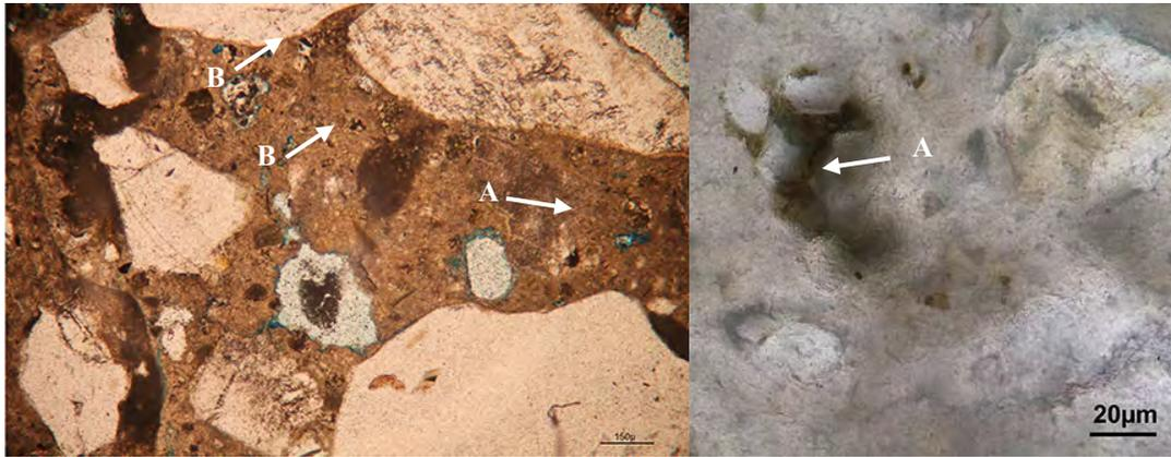
Figure 9. Thin section photomicrograph. Trasmited light. Detail of unhidrated belite (B) and alite (A) crystals.
