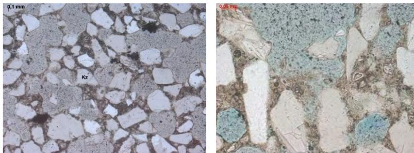
Figure 4. Left: Microphotograph of the aggregate (Kz = quartz sand) in mortar MS (after 28 days curing under outdoor conditions; parallel polarized light). Right: Microphotograph of a detail of mortar MS: in the binder  $C_2S$  and  $C_3S$  can be identified (after 28 days curing under outdoor conditions; parallel polarized light).
