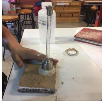
Figure 20. Water absorption test with Karsten tube. TECTRAD / INAH 2018
