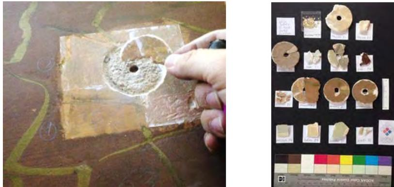
Figure 10. Detail of a sample extracted off the walls' coating in the main room of the Casa Batlló.
