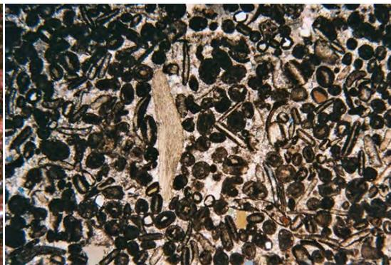
Figure 4. Petrographic image of the Portland stone consisting of ooliths and shells of microcrystalline carbonate cemented with coarser crystalline carbonate. 2X polarised light. Field of view c. 7 mm
