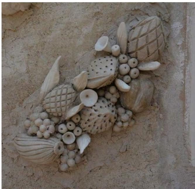
Figure 9. Trial replicas of the fruit decoration made according to the analytical results. Lime binder was made from marble sampled at the original outcrop, burnt in a wood-fired kiln and processed by wet slaking following the historic procedures.
