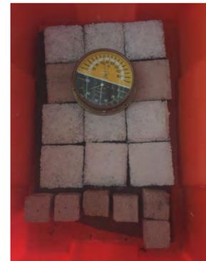
Figure 16 Formulated lime mortars in setting process under a high RH environment in accordance with ASTM C 1707. TECTRAD INAH 2019
