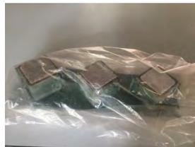
Figure 15 Formulated lime mortars stored in sealed bags before demolding in accordance with ASTM C 1707. TECTRAD INAH 2019
