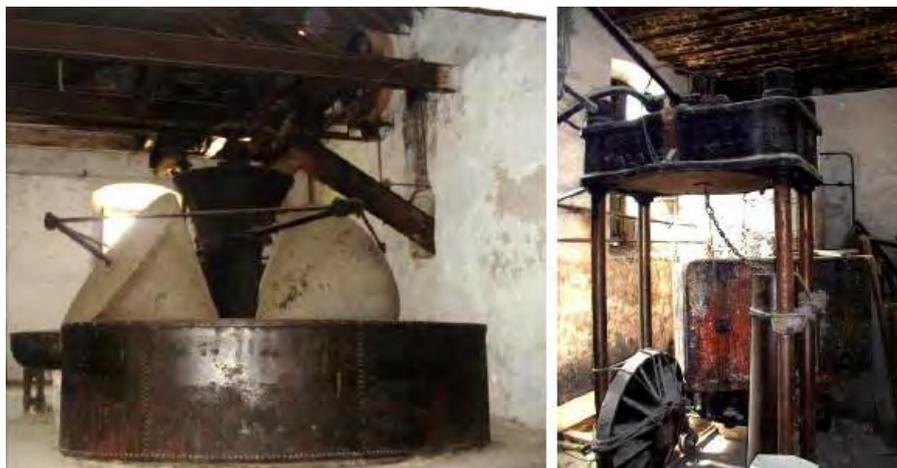
Figure 3. Water mill and presses with steam engine, all of them from 19<sup>th</sup> century
