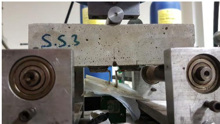
Figure 3. Testing arrangement on notched beams
