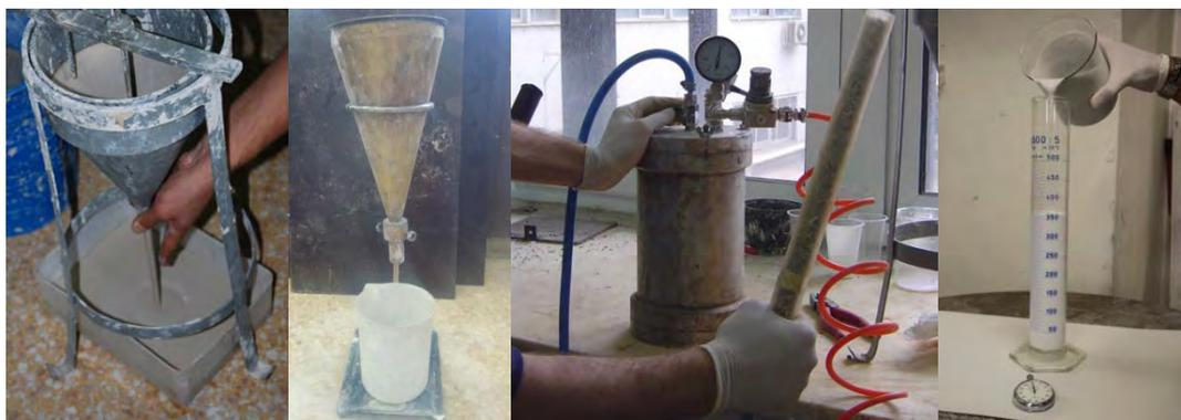
Figure 2. Fresh state properties testing. ASTM and EN flow cones (left), sand column test (middle), volume stability test (right).
