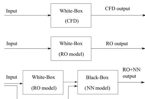
Figure 1: CFD, RO and grey-box (composed by the RO and ML) models.
