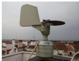
Fig. 2: Burkard 7-Day Volumetric Spore-trap® of Évora monitoring station RPA – SPAIC.
