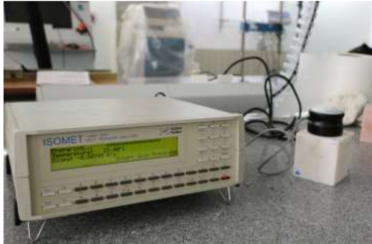
Fig. 1 Heat Transfer Analyser ISOMET 2104. The measuring probe is the black device on top of the rock sample.
