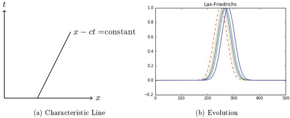
Figure 4.2: Characteristic and solution for the advection equation  $u_t + cu_x = 0, c > 0$
