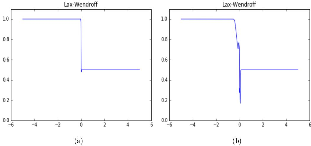
Figure 4.18: Rarefaction plot for the Lax-Wendroff scheme  $u_l = 1$  and  $u_r = \frac{1}{2}$
