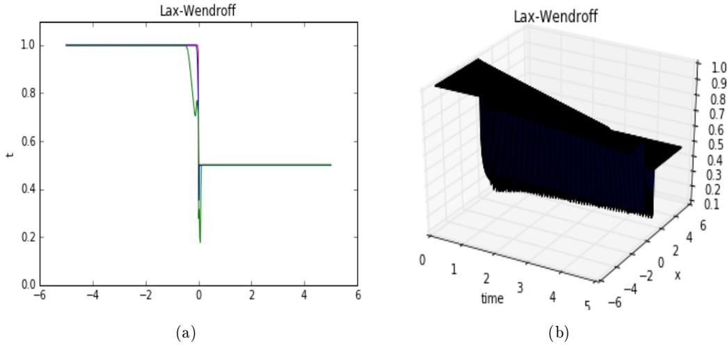
Figure 4.19: Rarefaction plot for the Lax-Wendroff scheme  $u_l = 1$  and  $u_r = \frac{1}{2}$
