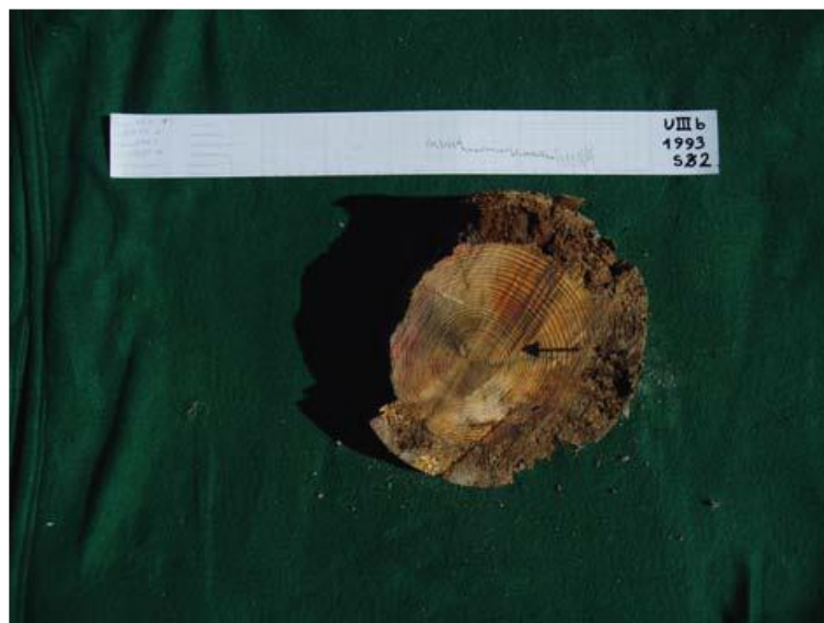
Figure 6 Slice of a wooden element. The resistograph reading is placed on the top of the wooden piece
