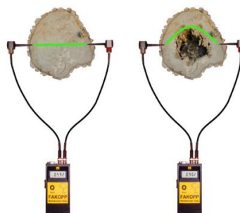
Figure 9 Microsecond timer. The device is designed to measure stress wave propagation time in trees
