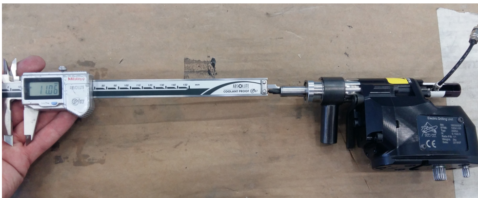
Figure 3.1: Drilling tool clash inside bayonet.
