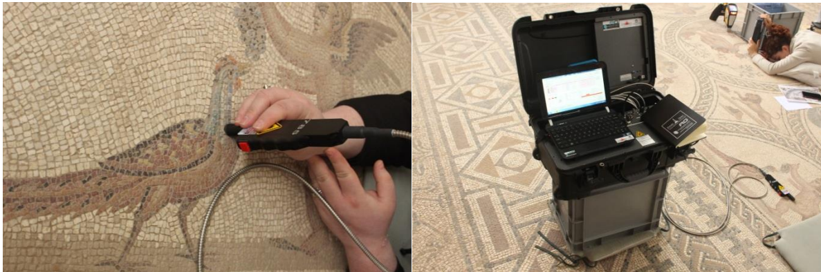
Figure 13 - Set up EZRAMAN-I-DUAL Raman spectrometer in the field.
