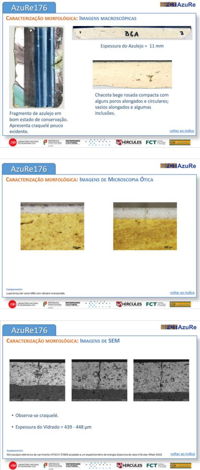
Figure 2. Morphological characterization data that can be found in the digital database: macroscopic observations; OM images and SEM images (top to bottom).
