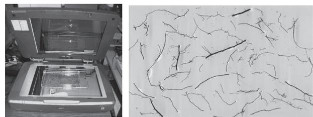
**Fig. 1.** Scanner EPSON Expression 1000XL with TPU in the lid (left), digital image of scanned roots of cork oak.
